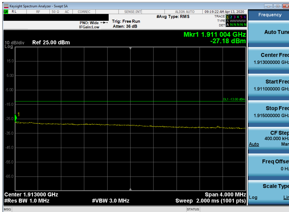
Plot 7-95. Extended Upper Band Edge Plot (LTE Band 2 - 15MHz QPSK – Full RB Configuration)
