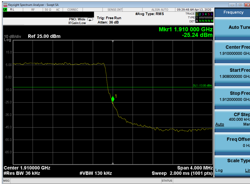
Plot 7-106. Upper Band Edge Plot (LTE Band 2 - 3MHz QPSK – Full RB Configuration)
