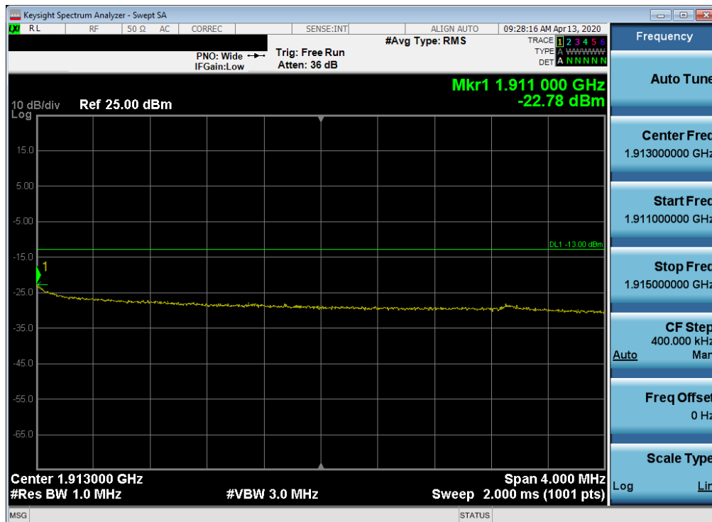
Plot 7-99. Extended Upper Band Edge Plot (LTE Band 2 - 10MHz QPSK – Full RB Configuration)
