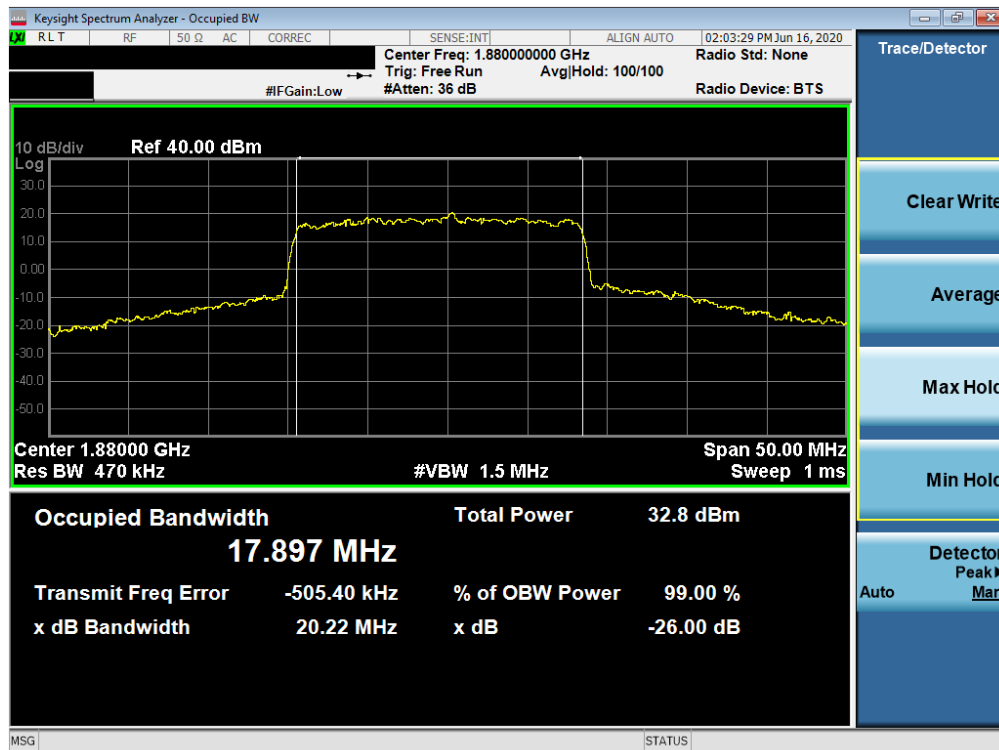
Plot 7-20. Occupied Bandwidth Plot (NR Band n2 - 20.0MHz CP-OFDM QPSK - Full RB)
