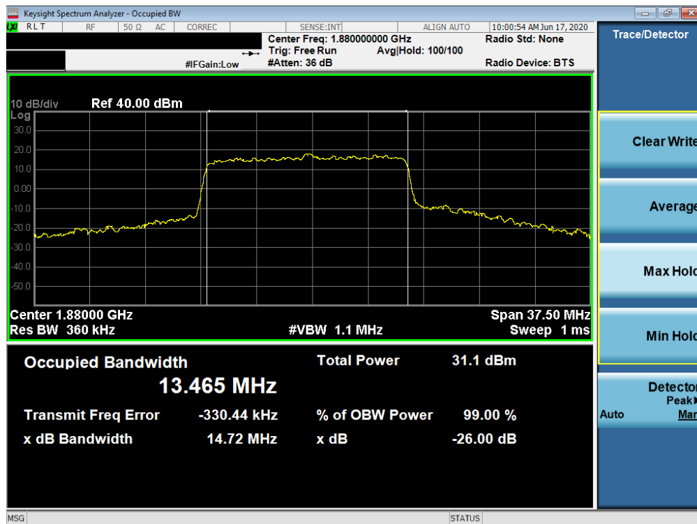
Plot 7-26. Occupied Bandwidth Plot (NR Band n2 - 15.0MHz CP-OFDM 16QAM - Full RB)
