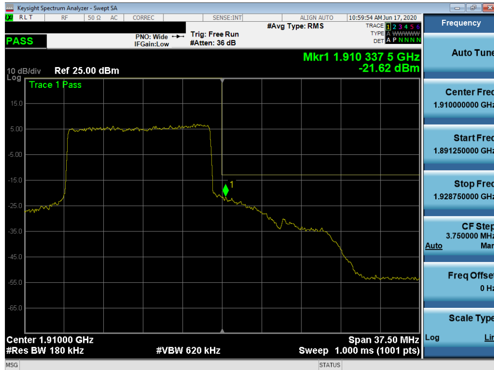
Plot 7-118. Upper Band Edge Plot (NR Band n2 – 15.0MHz - Full RB)
