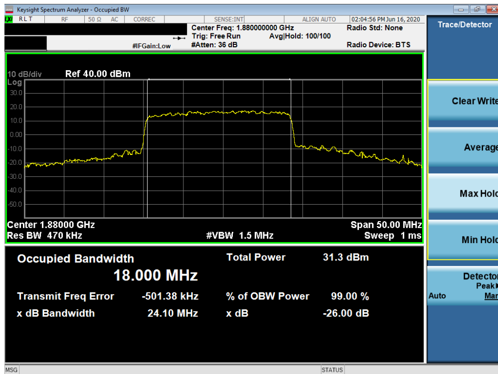
Plot 7-22. Occupied Bandwidth Plot (NR Band n2 - 20.0MHz CP-OFDM 64QAM - Full RB)
