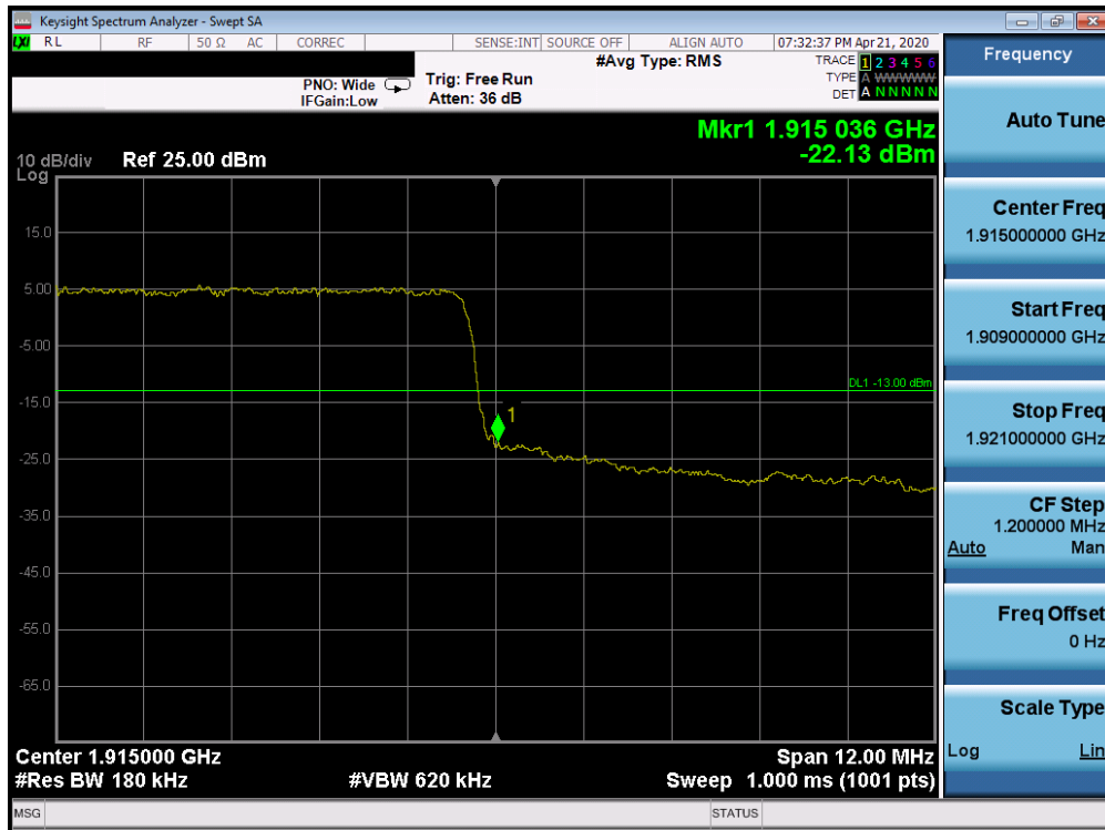
Plot 7-524. Upper 5G sub6 Band Edge Plot (5G sub6 n25 - 15.0MHz QPSK - Full RB Configuration)
