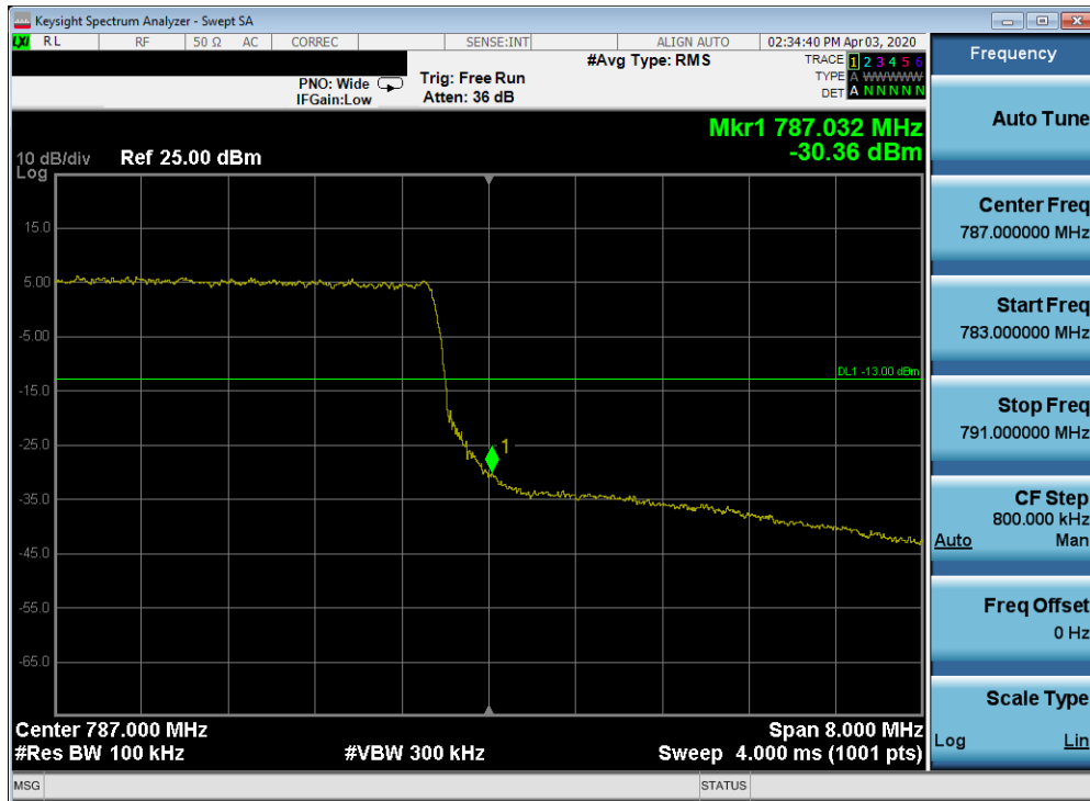
Plot 7-362. Upper Band Edge Plot (Band 13 - 10.0MHz QPSK - Full RB Configuration)
