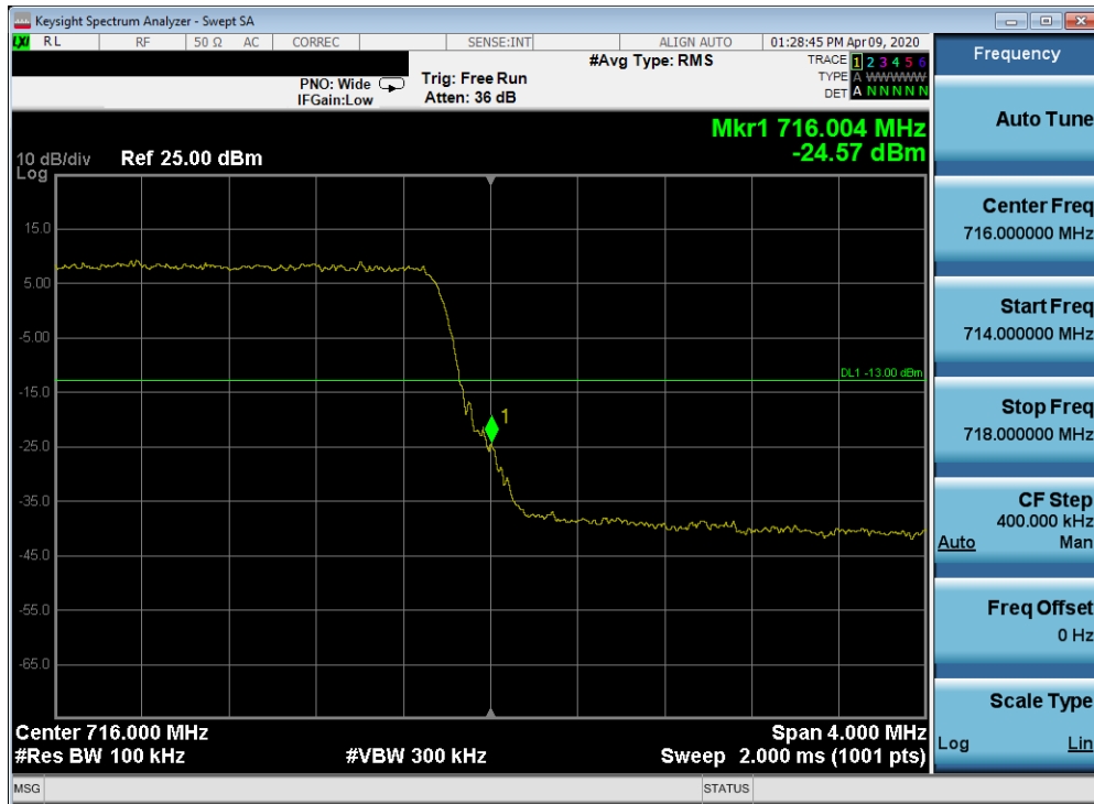
Plot 7-352. Upper Band Edge Plot (Band 12/17 - 5.0MHz QPSK - Full RB Configuration)
