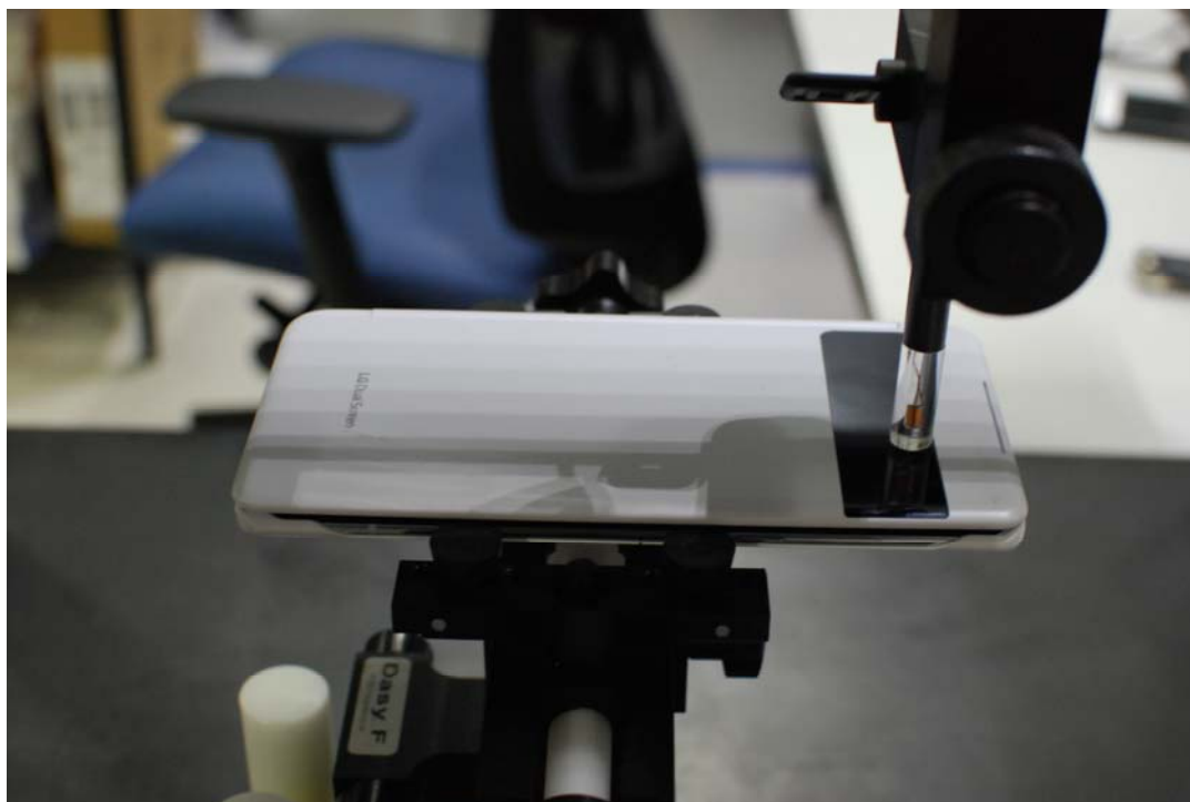
Figure 16-6 Test Setup for Wireless Device with Dual Display Cover - Closed
