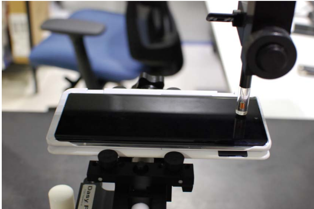
Figure 16-3 Test Setup for Wireless Device with Dual Display Cover - Open
