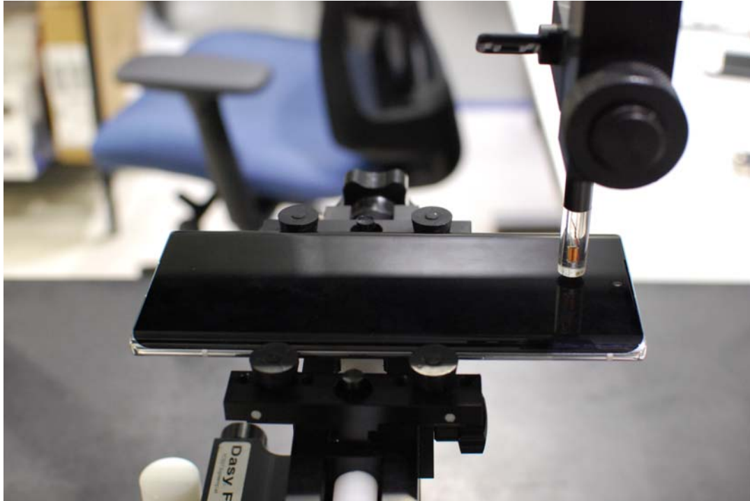
Figure 16-1 Test Setup for Wireless Device
