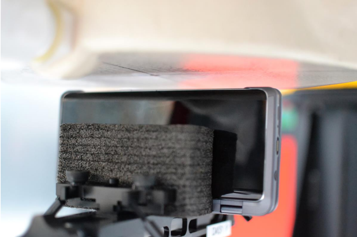
SAR Test Setup Photo 31 – Right Edge with Dual Display Accessory Position #3 at 10 mm
