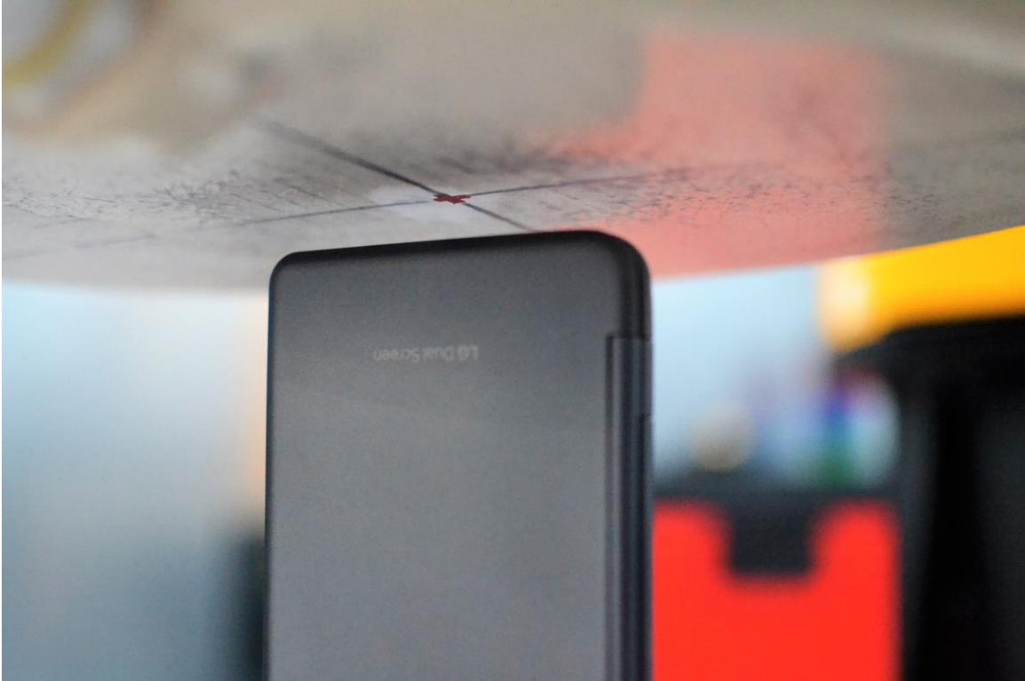
SAR Test Setup Photo 25 – Bottom Edge with Dual Display Accessory Position #1 at 10 mm
