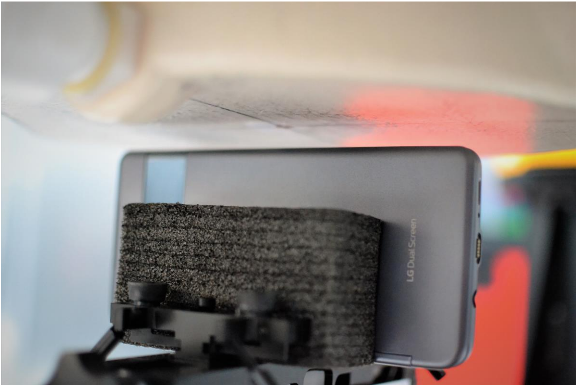
SAR Test Setup Photo 30 – Right Edge with Dual Display Accessory Position #1 at 10 mm
