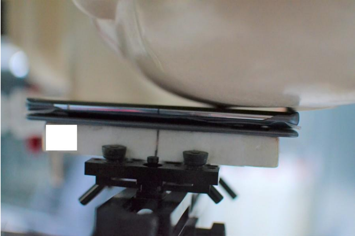
SAR Test Setup Photo 7 – Left Cheek with Dual Display Accessory Position #3
