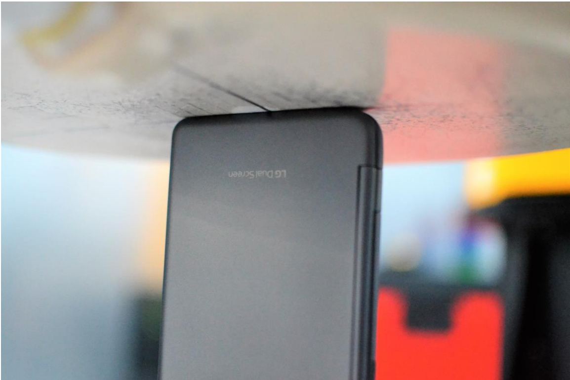
SAR Test Setup Photo 28 – Bottom Edge with Dual Display Accessory Position #1 at 0 mm
