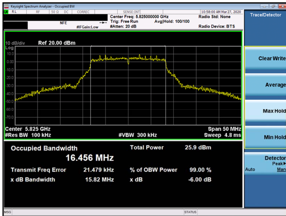
Plot 7-63. 6dB Bandwidth Plot SISO ANT1 (802.11a (UNII Band 3) – Ch. 165)
