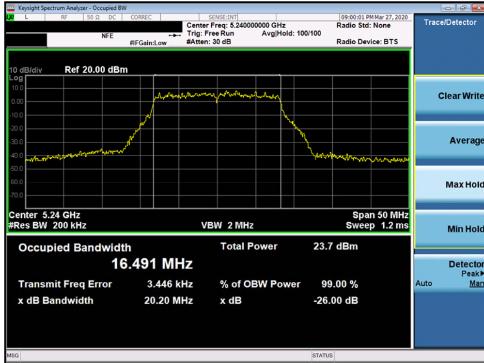
Plot 7-33. 26dB Bandwidth Plot SISO ANT2 (802.11a (UNII Band 1) – Ch. 48)
