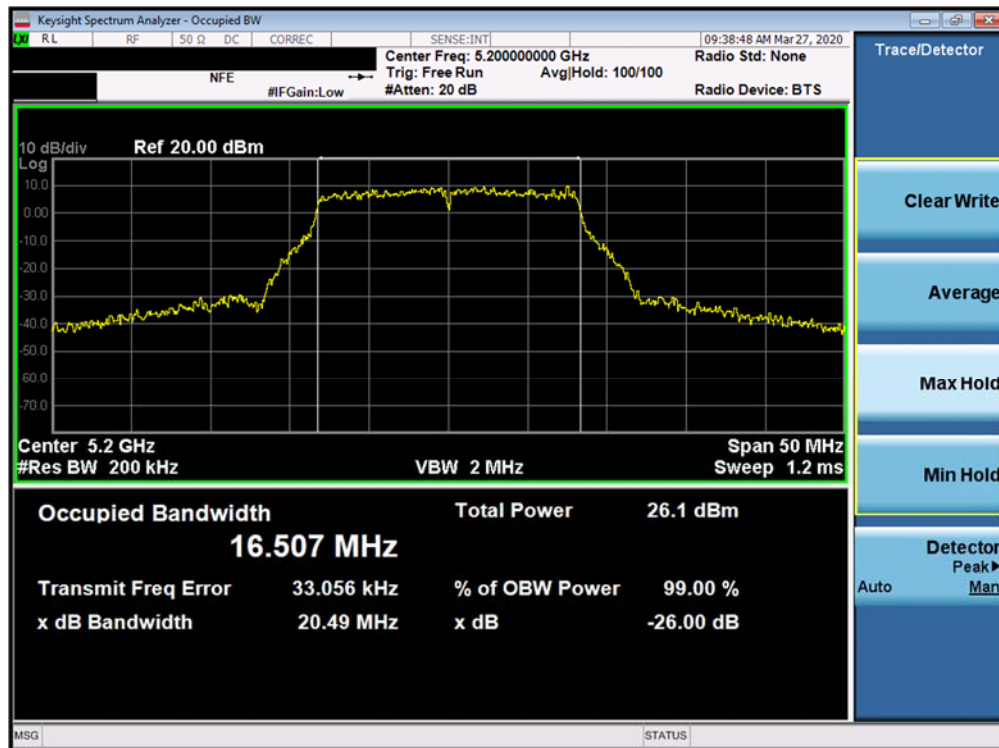
Plot 7-2. 26dB Bandwidth Plot SISO ANT1 (802.11a (UNII Band 1) – Ch. 40)
