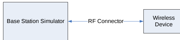
Figure 9-4 Power Measurement Setup
