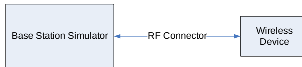
Figure 9-3 Power Measurement Setup
