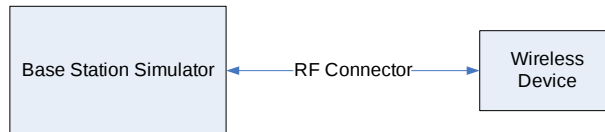
Figure 9-2 Power Measurement Setup
