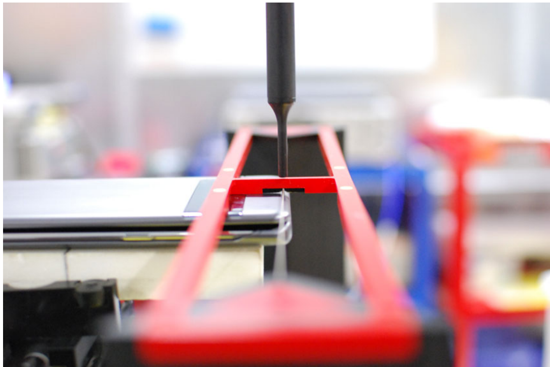
Figure 18-4 HAC Phantom Plane Alignment – Dual Display Closed
