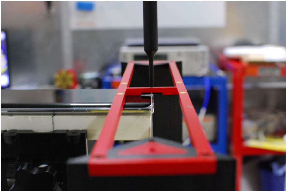
Figure 18-2 HAC Phantom Plane Alignment
