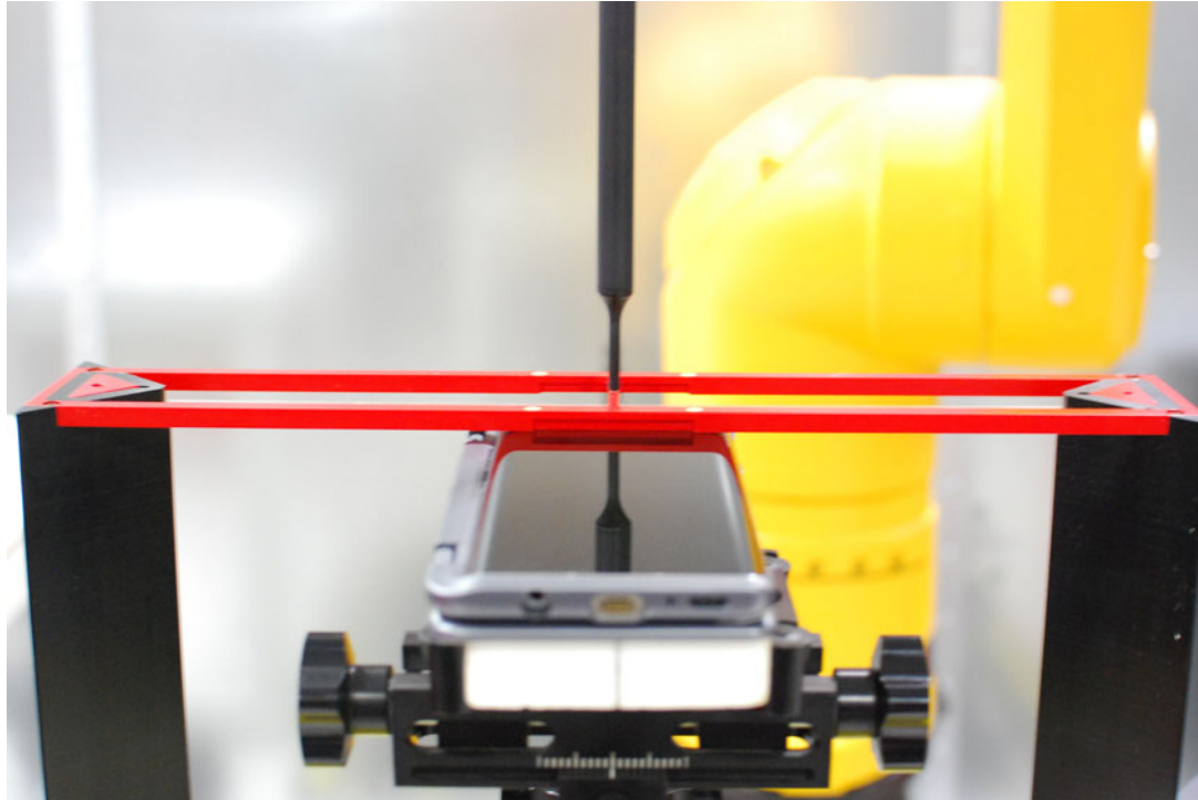
Figure 18-5 Ear Reference Point HAC Phantom Alignment – Dual Display Open
