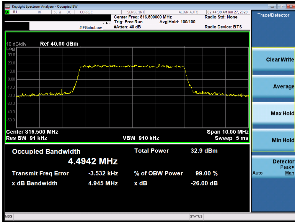
Plot 7-9. Occupied Bandwidth Plot (LTE Band 26 - 5MHz QPSK - Full RB Configuration)
