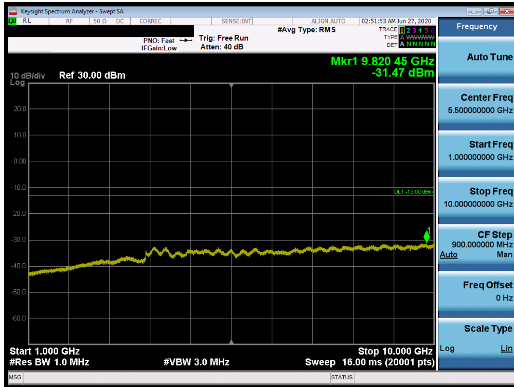
Plot 7-26. Conducted Spurious Plot (LTE Band 26 - 15MHz QPSK - RB Size 1, RB Offset 0 - Mid Channel)
