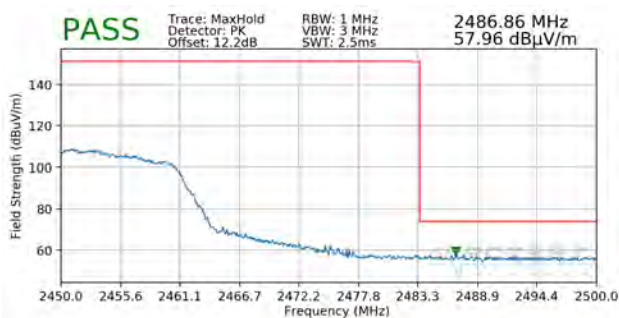
Plot 7-20. Radiated Restricted Upper Band Edge Measurement SISO ANT1 (Peak)
