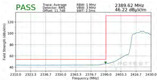
Plot 7-35. Radiated Restricted Lower Band Edge Measurement SISO ANT2 (Average)
