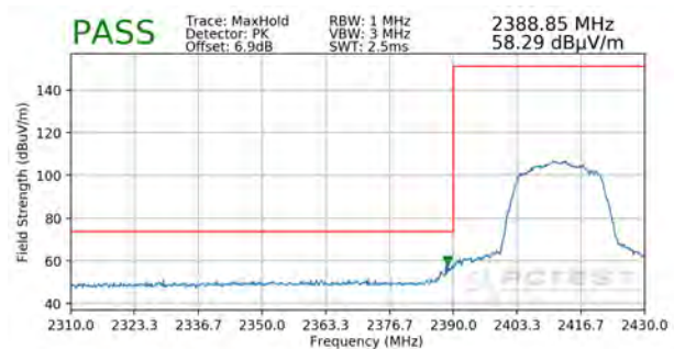
Plot 7-30. Radiated Restricted Band Edge Measurement SISO ANT1 with WCP and DS (Peak)
