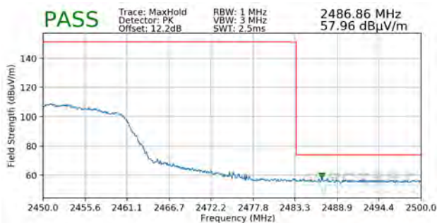
Plot 7-38. Radiated Restricted Upper Band Edge Measurement SISO ANT2 (Peak)
