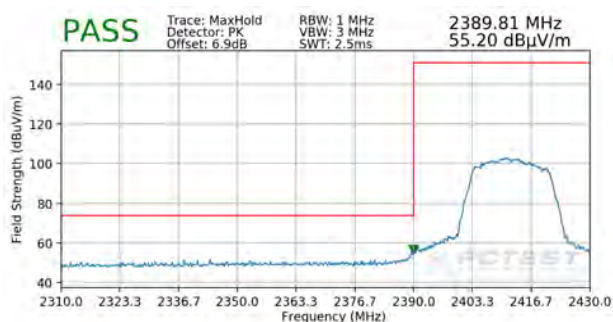
Plot 7-32. Radiated Restricted Lower Band Edge Measurement SISO ANT2 (Peak)
