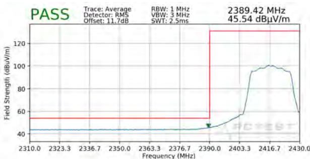
Plot 7-33. Radiated Restricted Lower Band Edge Measurement SISO ANT2 (Average)
