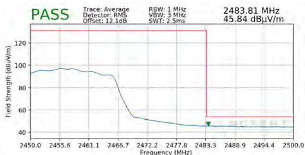
Plot 7-39. Radiated Restricted Upper Band Edge Measurement SISO ANT2 (Average)
