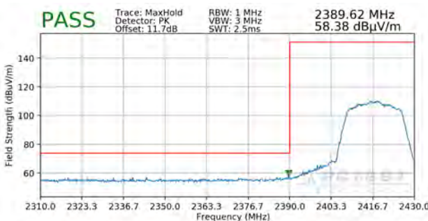
Plot 7-34. Radiated Restricted Lower Band Edge Measurement SISO ANT2 (Peak)
