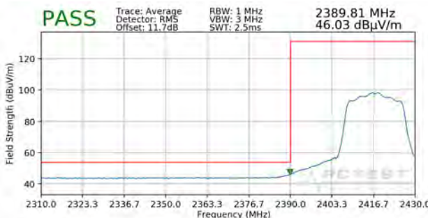
Plot 7-15. Radiated Restricted Lower Band Edge Measurement SISO ANT1 (Average)
