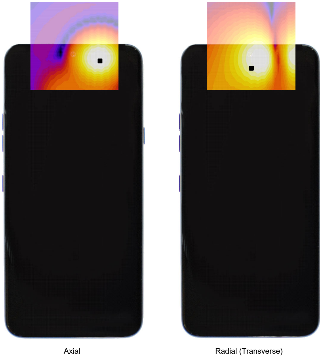
Figure 16-7 T-Coil Scan Overlay Magnetic Field Distributions
