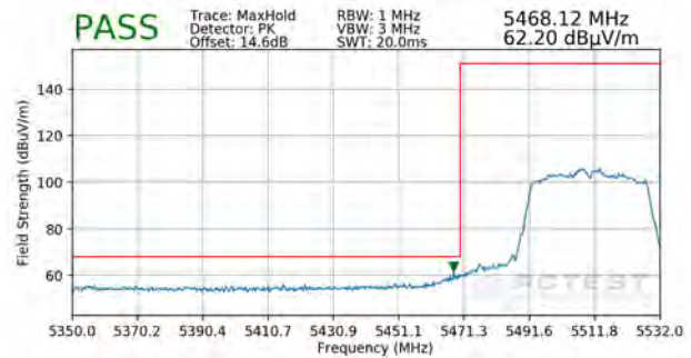
Plot 7-246. Radiated Lower Band Edge Plot MIMO (Peak – UNII Band 2C)
