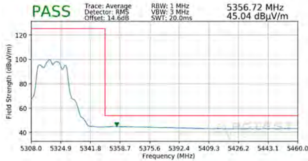
Plot 7-239. Radiated Band Edge Plot MIMO (Average – WCP)
