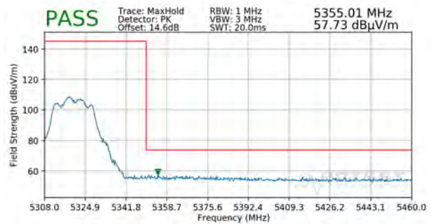
Plot 7-235. Radiated Upper Band Edge Plot MIMO (Peak – UNII Band 2A)
