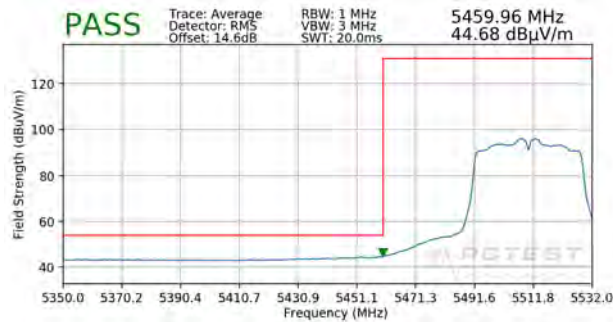
Plot 7-245. Radiated Lower Band Edge Plot MIMO (Average – UNII Band 2C)
