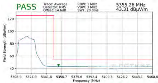
Plot 7-207. Radiated Upper Band Edge Plot SISO ANT2 (Average – UNII Band 2A)
