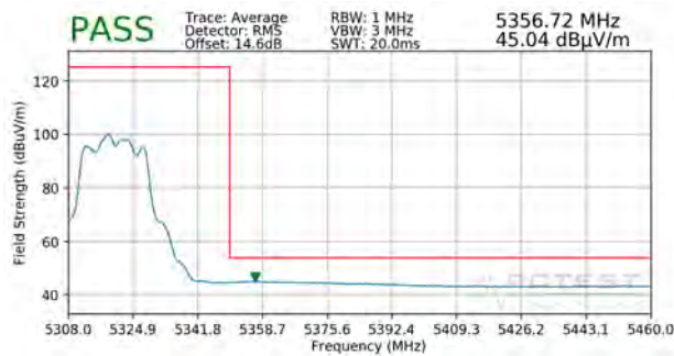
Plot 7-234. Radiated Upper Band Edge Plot MIMO (Average – UNII Band 2A)
