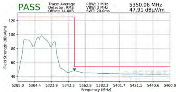
Plot 7-189. Radiated Upper Band Edge Plot SISO ANT1 (Average – UNII Band 2A)
