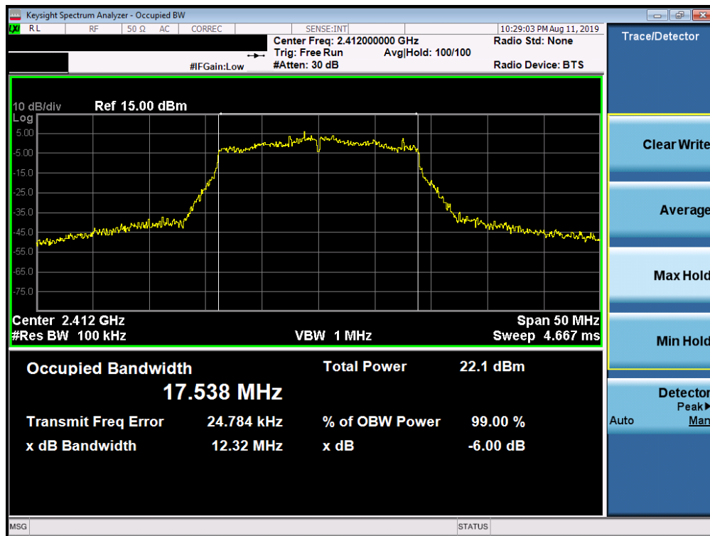
Plot 7-22. 6dB Bandwidth Plot SISO ANT2 (802.11ac (2.4GHz) – Ch. 1)
