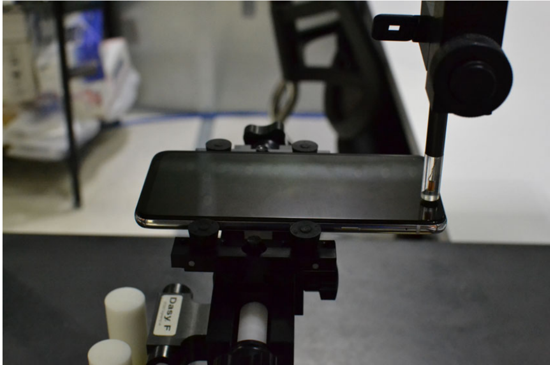
Figure 16-1 Test Setup for Wireless Device
