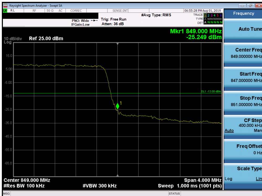
Plot 7-208. Upper Band Edge Plot (Band 26/5 - 5.0MHz QPSK - Full RB Configuration)
