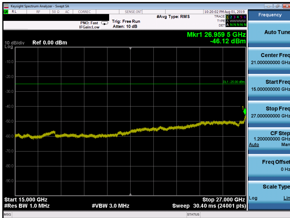
Plot 7-168. Conducted Spurious Plot (Band 7 - 20.0MHz QPSK - RB Size 1, RB Offset 0 – Mid Channel)
