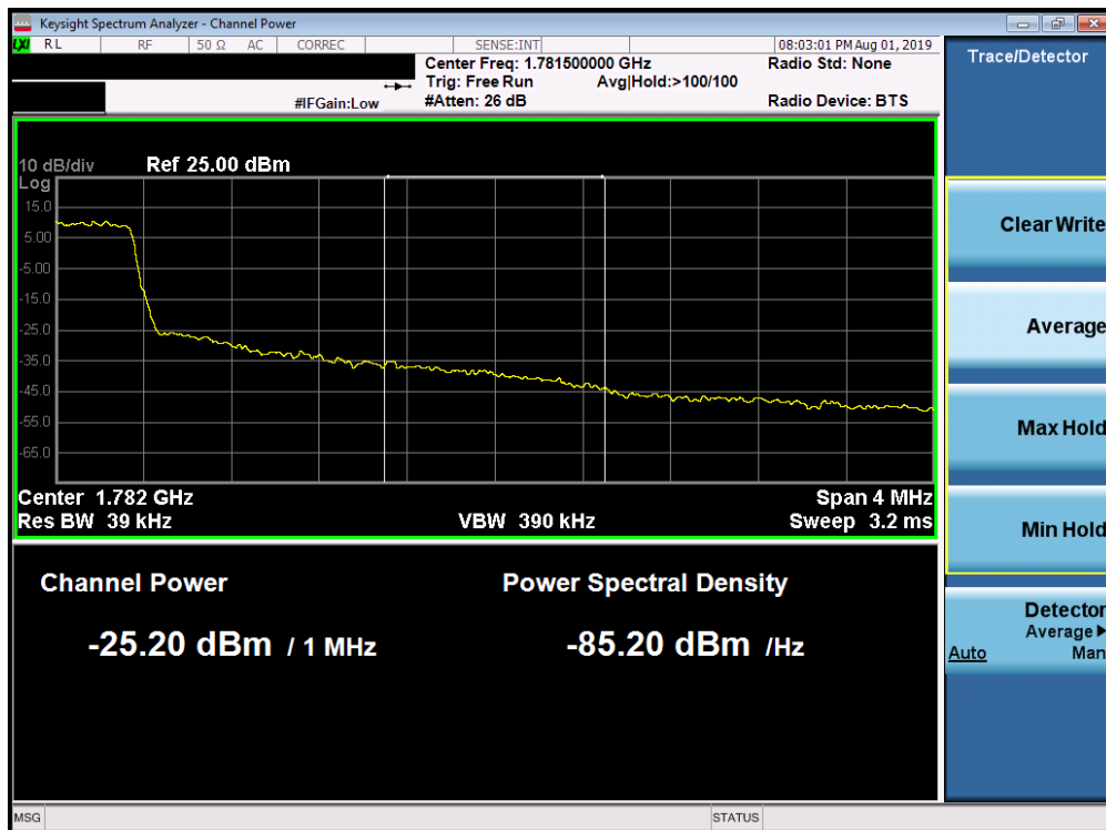
Plot 7-218. Upper Extended Band Edge Plot (Band 66 - 1.4MHz QPSK - Full RB Configuration)
