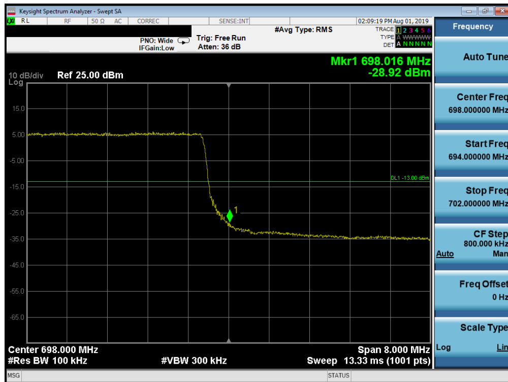
Plot 7-184. Upper Band Edge Plot (Band 71 - 10.0MHz QPSK - Full RB Configuration)
