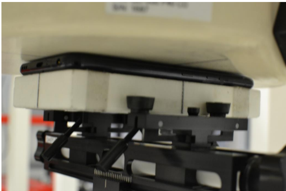
SAR Test Setup Photo 13: Back Side at 0 mm
