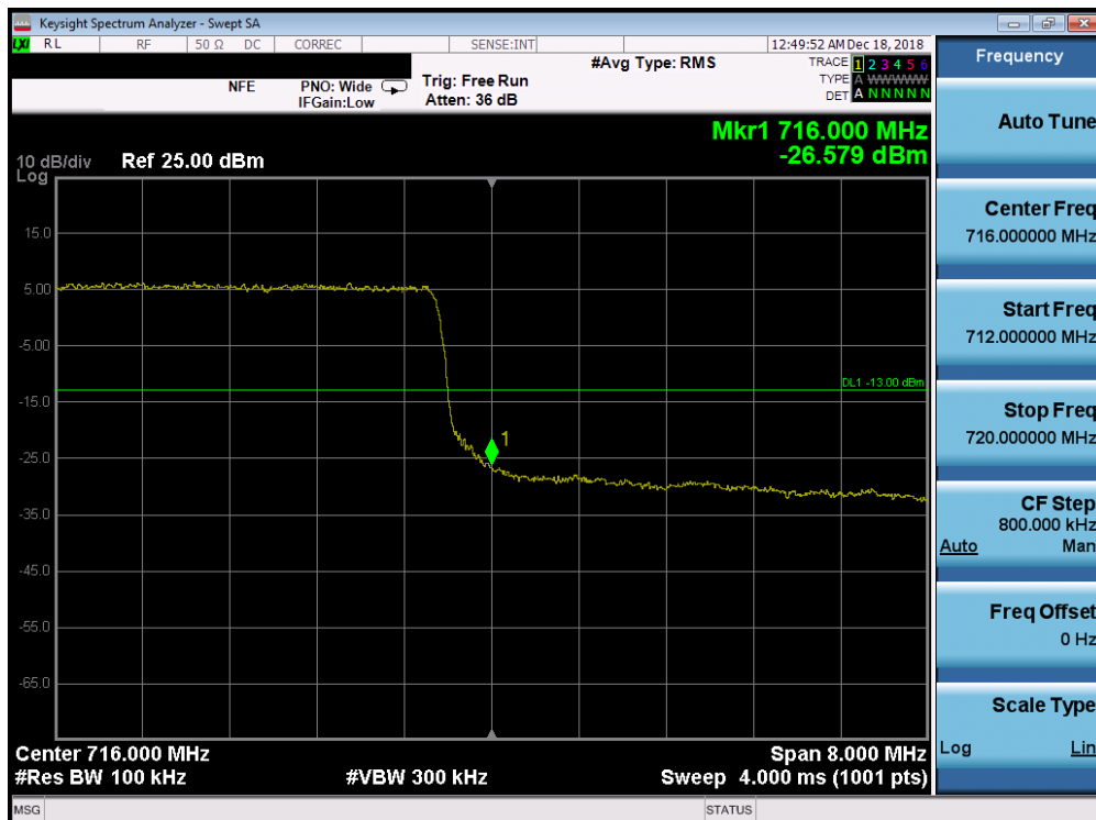
Plot 7-204. Upper Band Edge Plot (Band 12/17 - 10.0MHz QPSK - Full RB Configuration)
