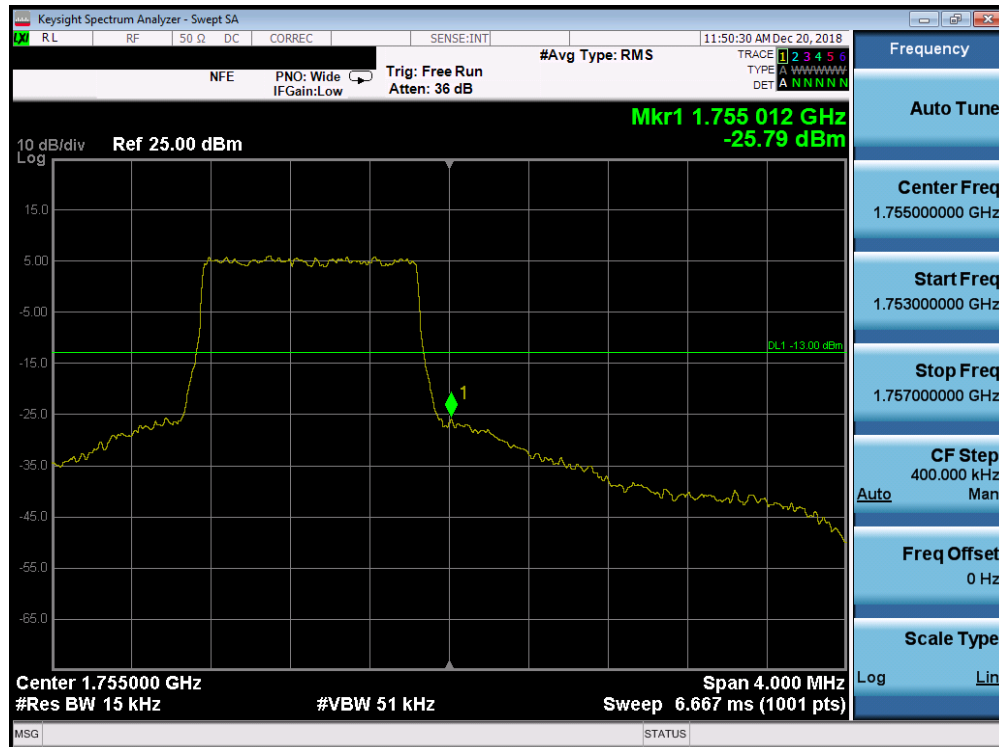
Plot 7-221. Upper Band Edge Plot (Band 4 - 1.4MHz QPSK - Full RB Configuration)
