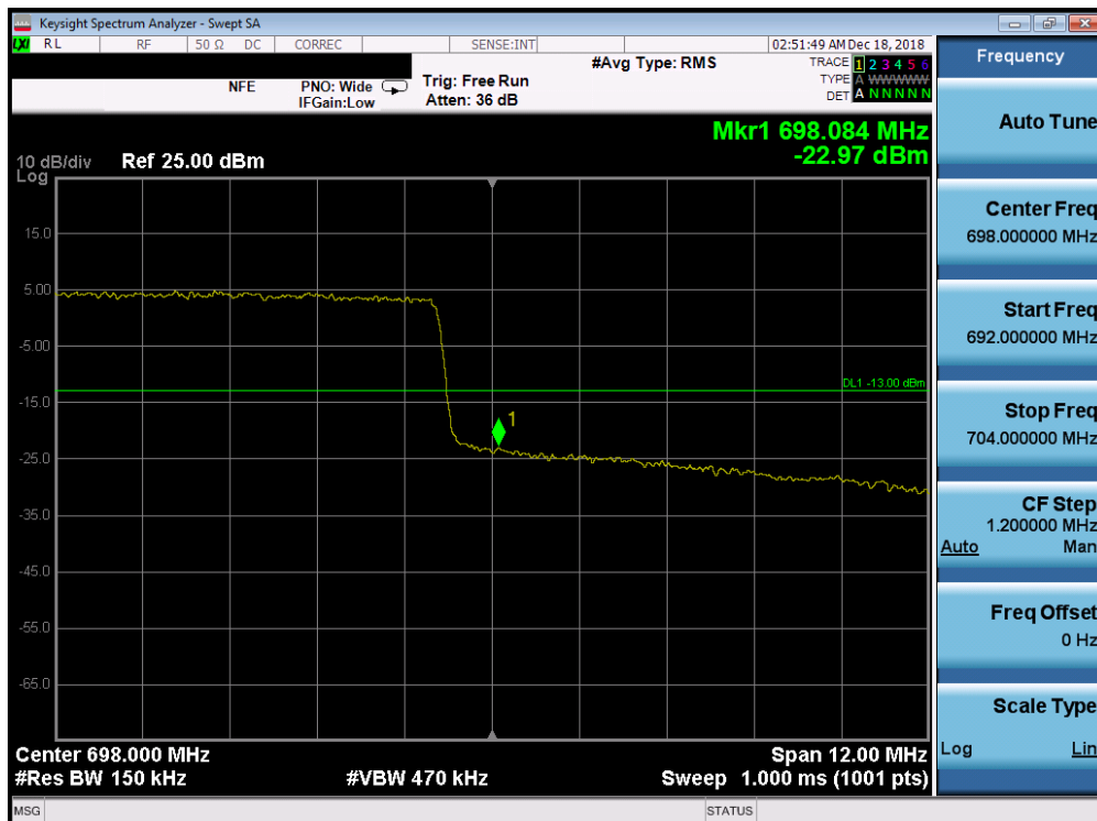
Plot 7-192. Upper Band Edge Plot (Band 71 - 15.0MHz QPSK - Full RB Configuration)
