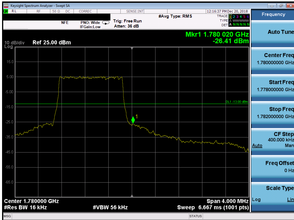
Plot 7-223. Upper Band Edge Plot (Band 66 - 1.4MHz QPSK - Full RB Configuration)
