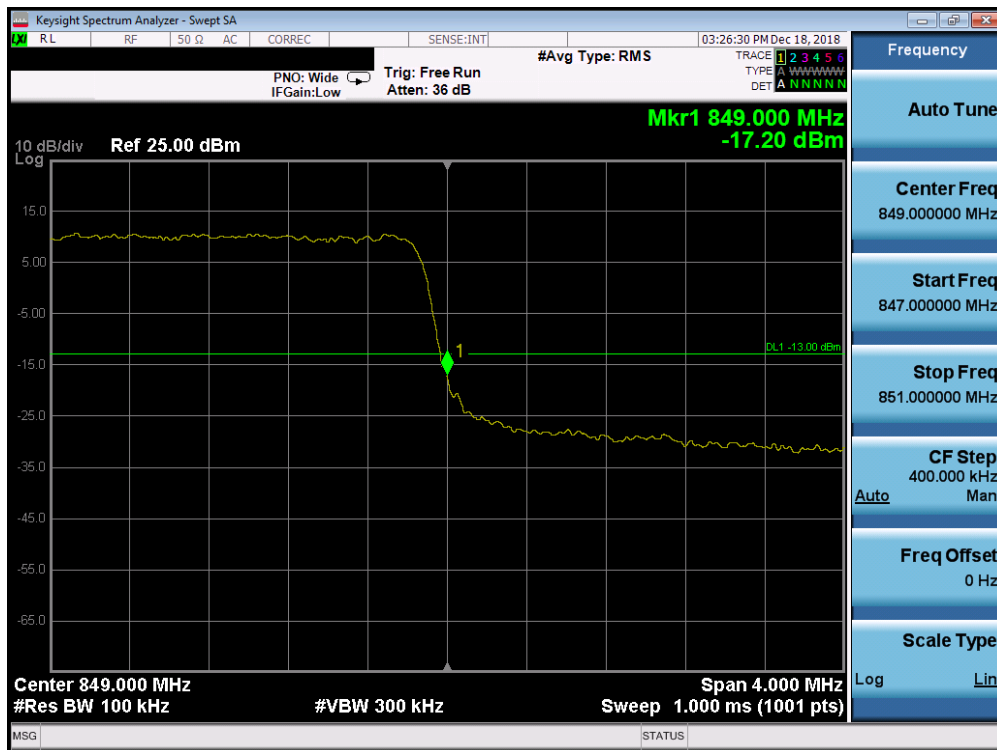
Plot 7-212. Upper Band Edge Plot (Band 26/5 - 3.0MHz QPSK - Full RB Configuration)
