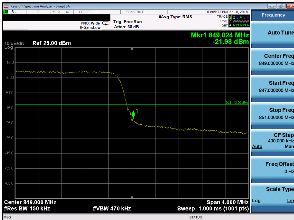
Plot 7-214. Upper Band Edge Plot (Band 26/5 - 5.0MHz QPSK - Full RB Configuration)
