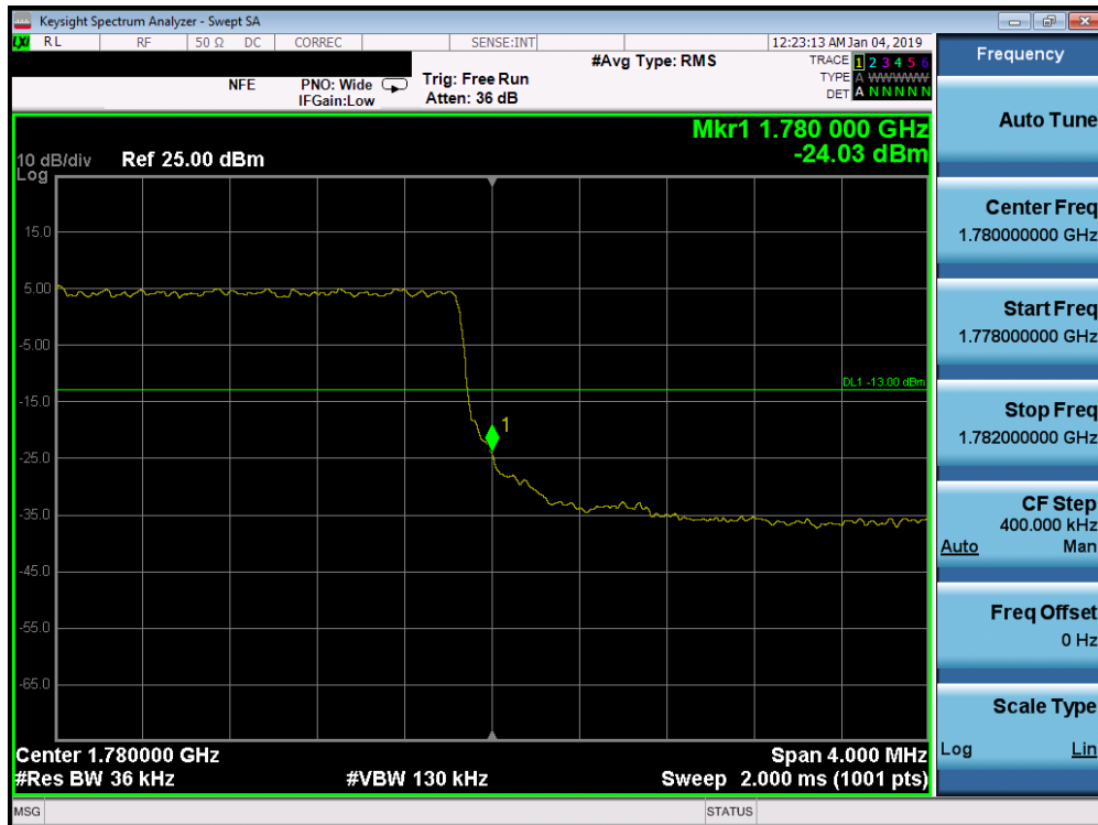
Plot 7-229. Upper Band Edge Plot (Band 66 - 3.0MHz QPSK - Full RB Configuration)
