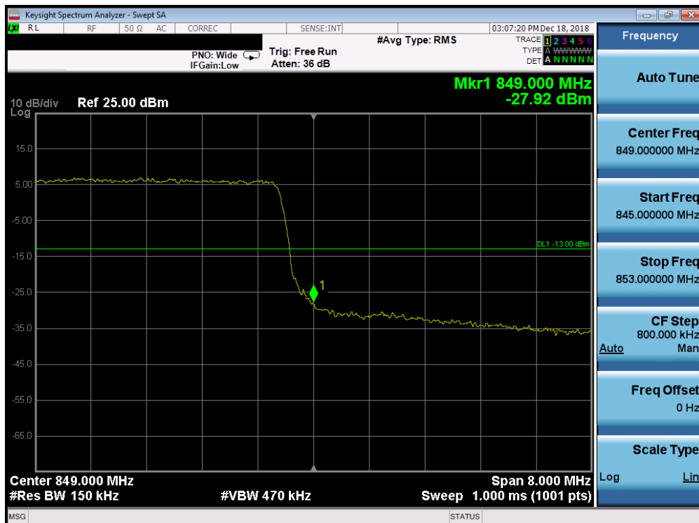
Plot 7-216. Upper Band Edge Plot (Band 26/5 - 10.0MHz QPSK - Full RB Configuration)
