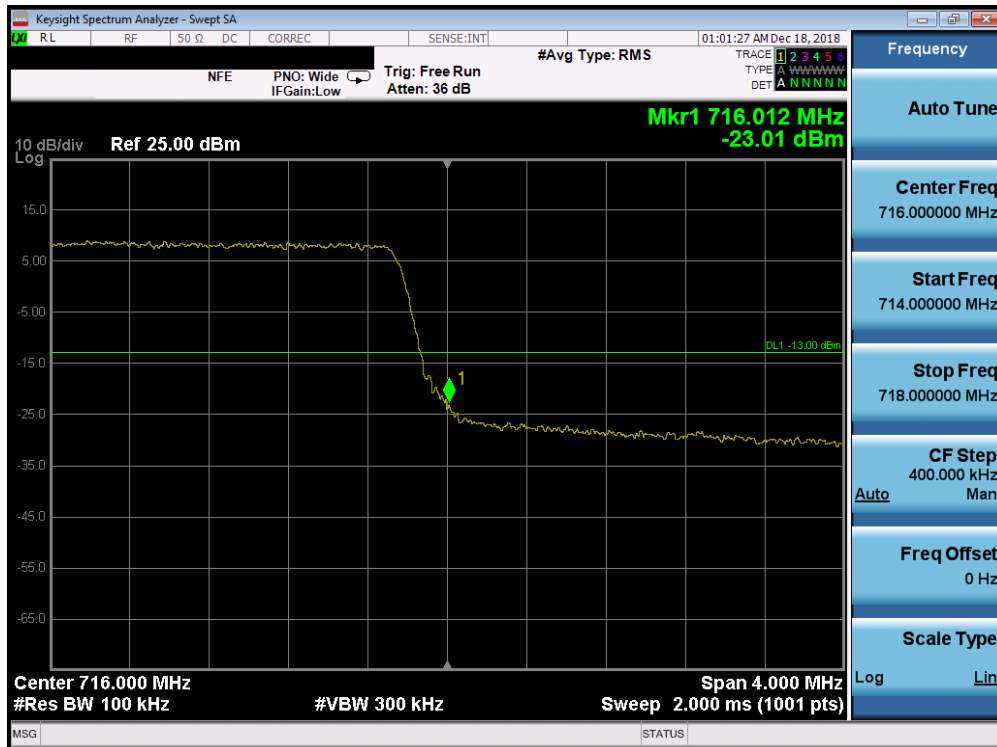
Plot 7-201. Upper Band Edge Plot (Band 12/17 - 5.0MHz QPSK - Full RB Configuration)
