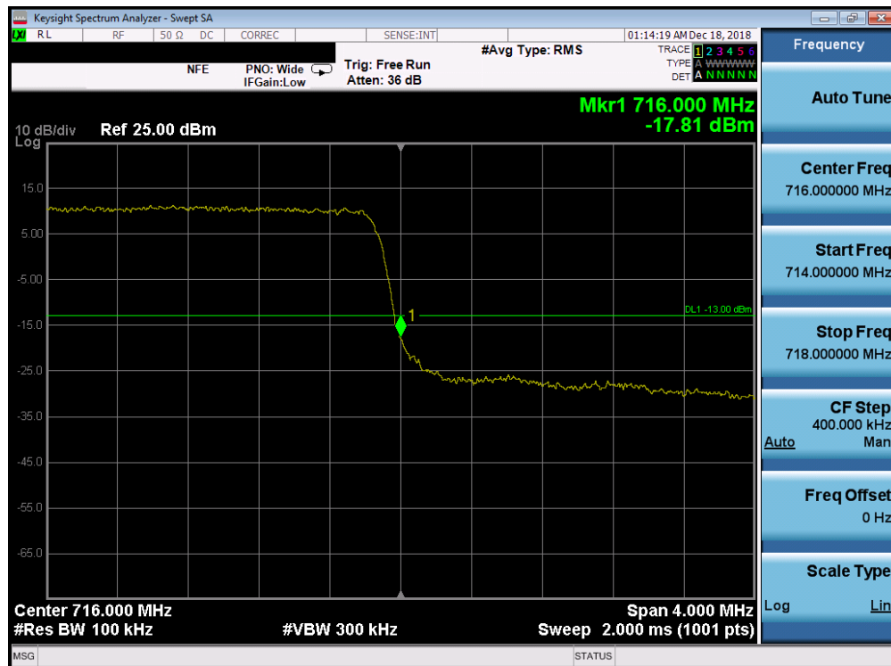
Plot 7-198. Upper Band Edge Plot (Band 12 - 3.0MHz QPSK - Full RB Configuration)
