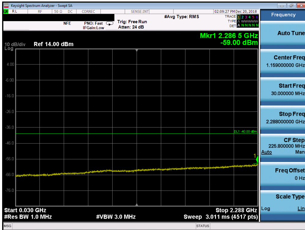
Plot 7-166. Conducted Spurious Plot (Band 30 - 5.0MHz QPSK - RB Size 1, RB Offset 0 - High Channel)
