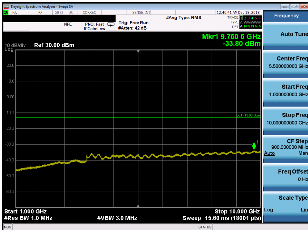
Plot 7-126. Conducted Spurious Plot (Band 12/17 - 10.0MHz QPSK - RB Size 1, RB Offset 0 - Mid Channel)
