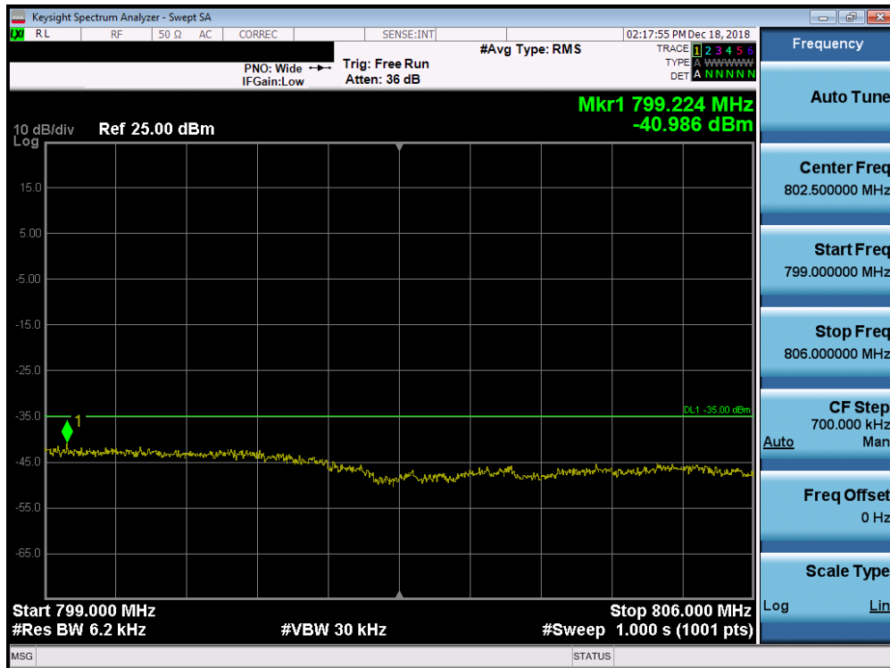
Plot 7-49. Upper Emission Mask Plot (LTE Band 14, 5MHz QPSK - RB Size 25)
