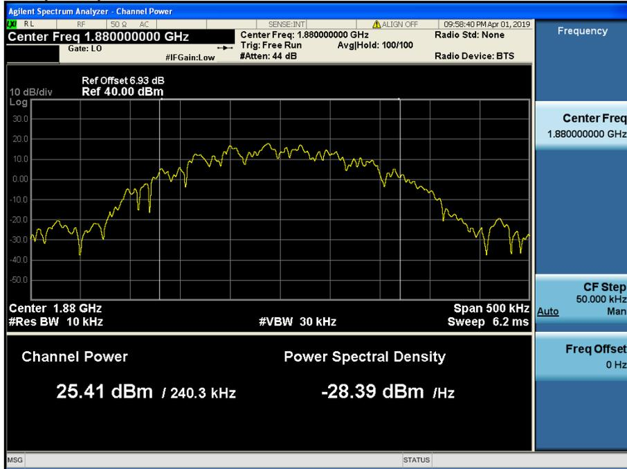
**PAPR (dB) = P<sub>pk</sub> (dBm) - P<sub>avg</sub> (dBm) = 25.83 dBm – 25.41 dBm = 0.42 dB**
