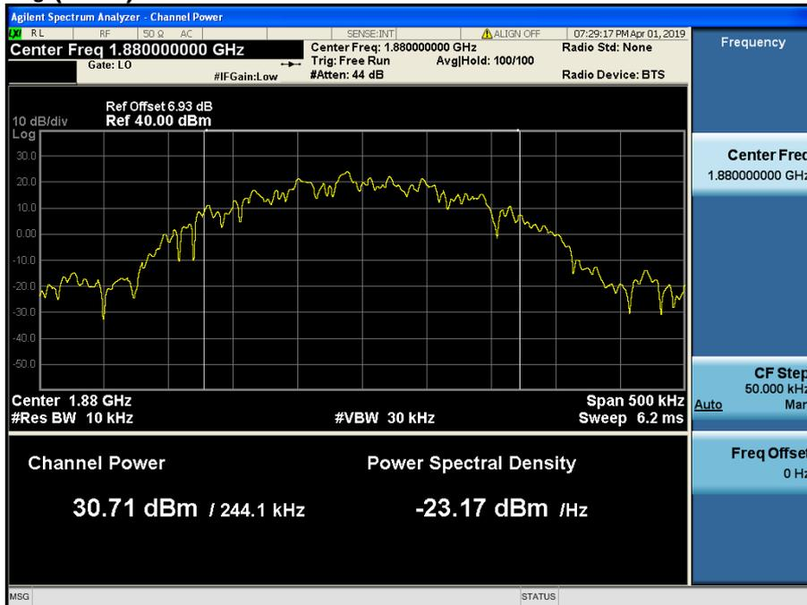
$$PAPR (dB) = P_{Pk} (dBm) - P_{Avg} (dBm) = 31.05 \text{ dBm} - 30.71 \text{ dBm} = 0.34 \text{ dB}$$
