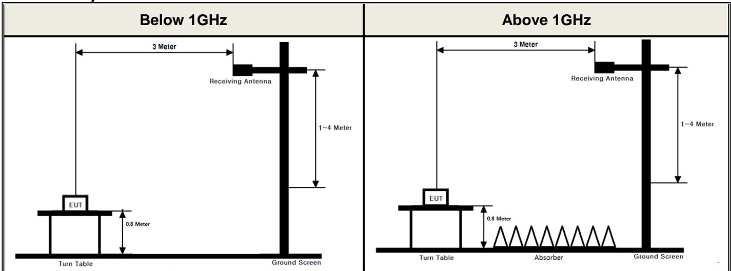
These measurements were performed at 3 m test site. The equipment under test is placed on a non-conductive table 0.8-meters above a turntable which is flush with the ground plane and 3 meters from the receive antenna. For measurements above 1 GHz absorbers are placed on the floor between the turn table and the antenna mast in such a way so as to maximize the reduction of reflections. For measurements below 1 GHz, the absorbers are removed.
