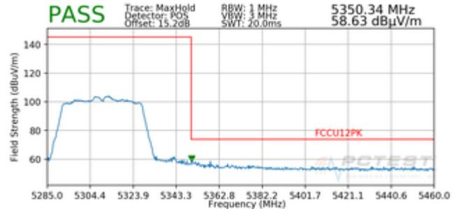
**Plot 7-211. Radiated Upper Band Edge Plot (Peak – UNII Band 2A)**
