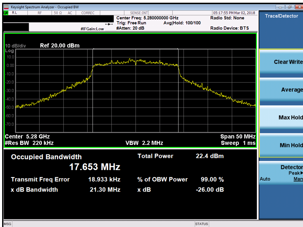
Plot 7-14. 26dB Bandwidth Plot (20MHz BW 802.11n (UNII Band 2A) – Ch. 56)
