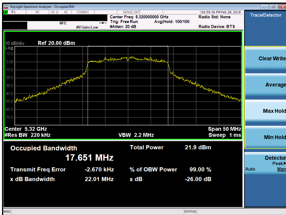
Plot 7-45. 26dB Bandwidth Plot (20MHz BW 802.11n (UNII Band 2A) – Ch. 64)
