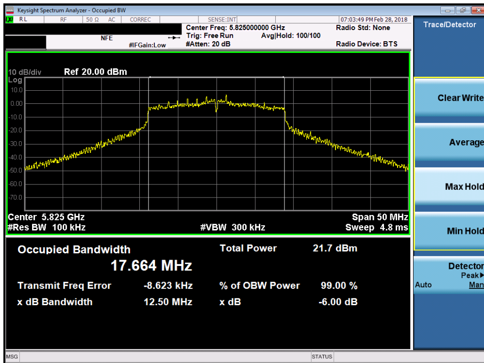
Plot 7-75. 6dB Bandwidth Plot (20MHz BW 802.11n (UNII Band 3) – Ch. 165)
