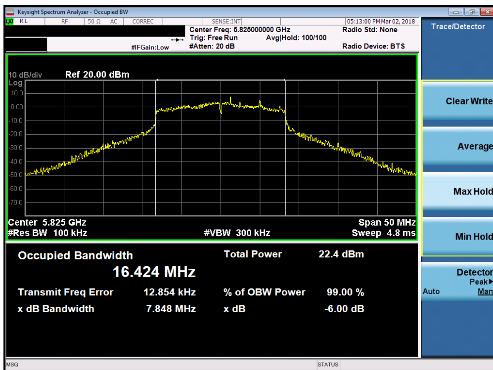
Plot 7-63. 6dB Bandwidth Plot (802.11a (UNII Band 3) – Ch. 165)
