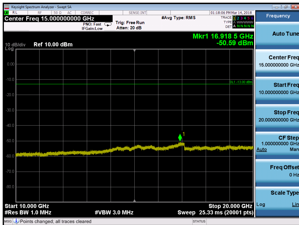
Plot 7-57. Conducted Spurious Plot (AWS WCDMA Mode - Low Channel)
