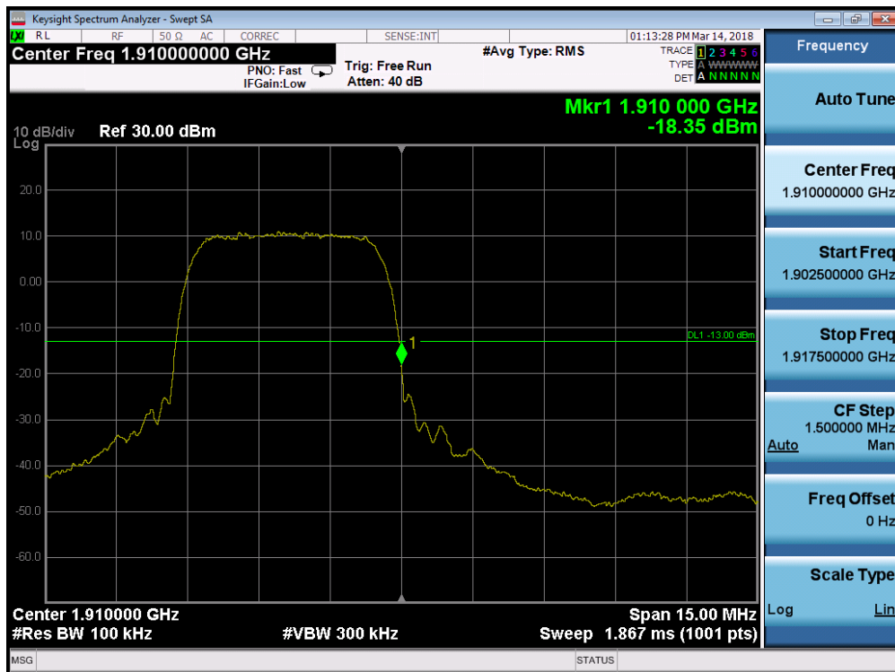
Plot 7-94. Band Edge Plot (PCS WCDMA Mode - High Channel)
