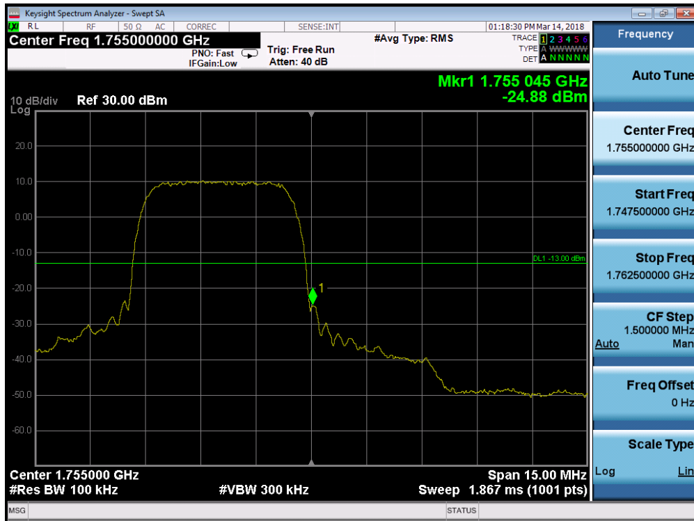
Plot 7-90. Band Edge Plot (AWS WCDMA Mode - High Channel)
