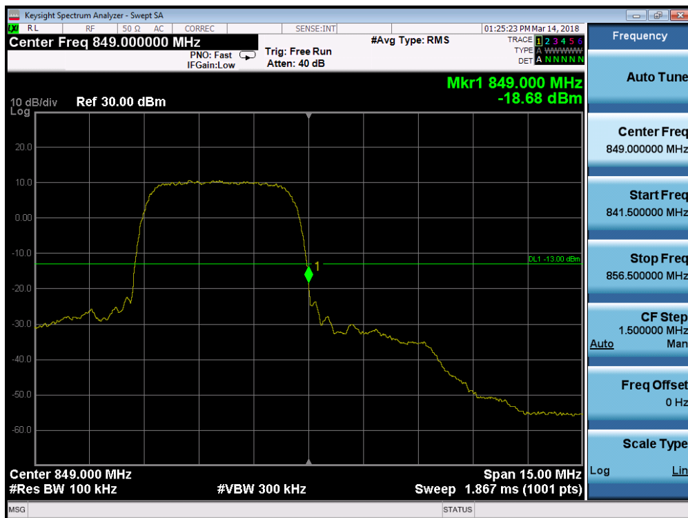
Plot 7-87. Band Edge Plot (Cellular WCDMA Mode - High Channel)
