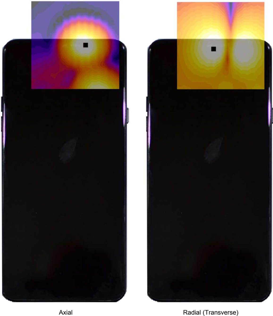
Figure 16-3 T-Coil Scan Overlay Magnetic Field Distributions
