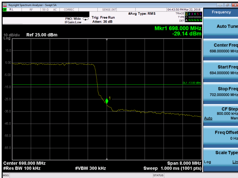
Plot 7-181. Upper Band Edge Plot (Band 71 - 10.0MHz QPSK - Full RB Configuration)
