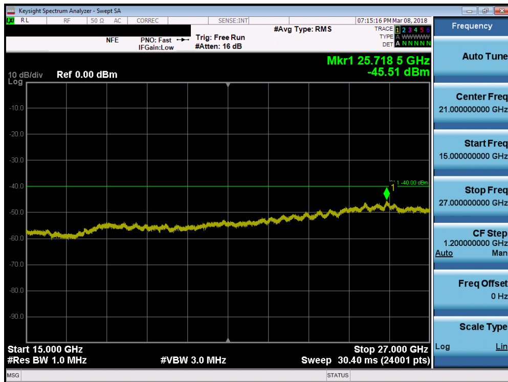
Plot 7-159. Conducted Spurious Plot (Band 30 - 10.0MHz QPSK - RB Size 1, RB Offset 0)
