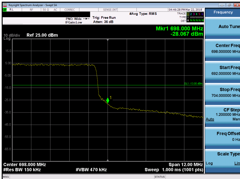
Plot 7-183. Upper Band Edge Plot (Band 71 - 15.0MHz QPSK - Full RB Configuration)
