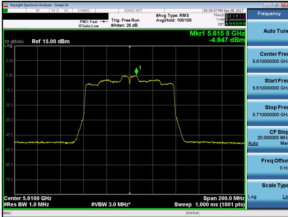
Plot 7-89. Power Spectral Density Plot (80MHz BW 802.11ac (UNII Band 2C) – Ch. 122)
