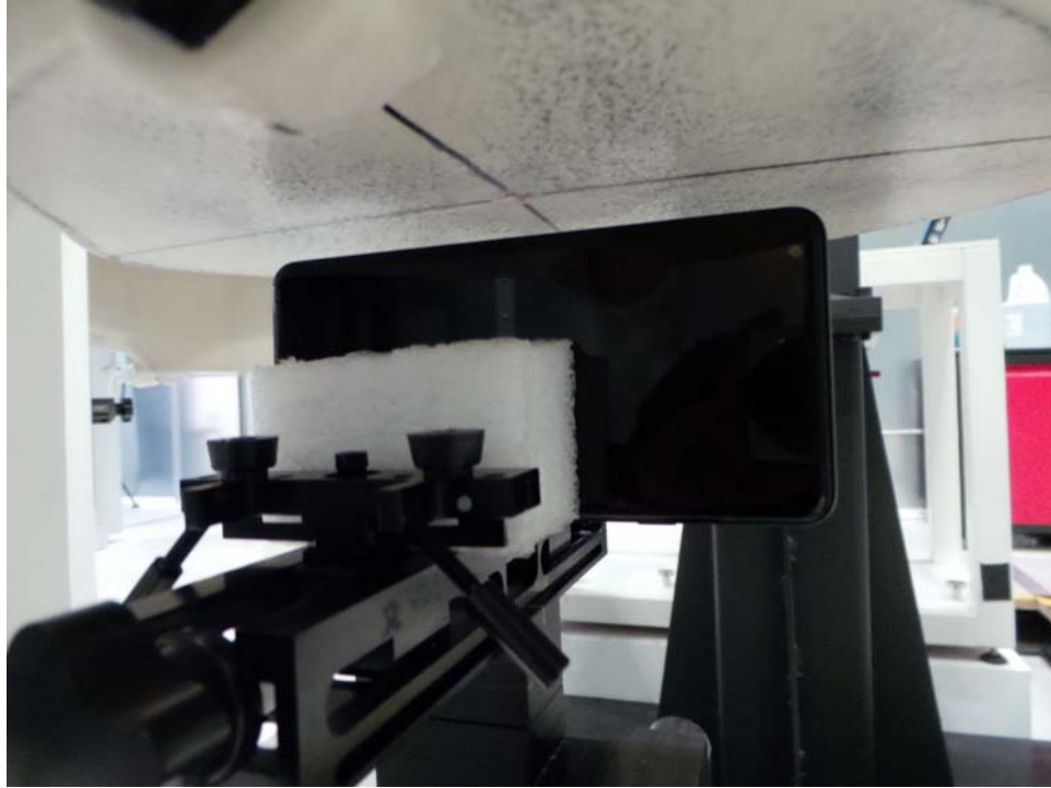
SAR Test Setup Photo 13: Left at 1.0 cm
