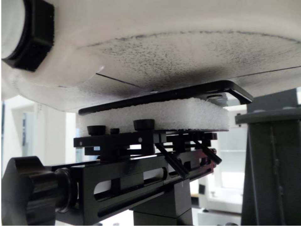
SAR Test Setup Photo 7: Front at 1.0 cm
