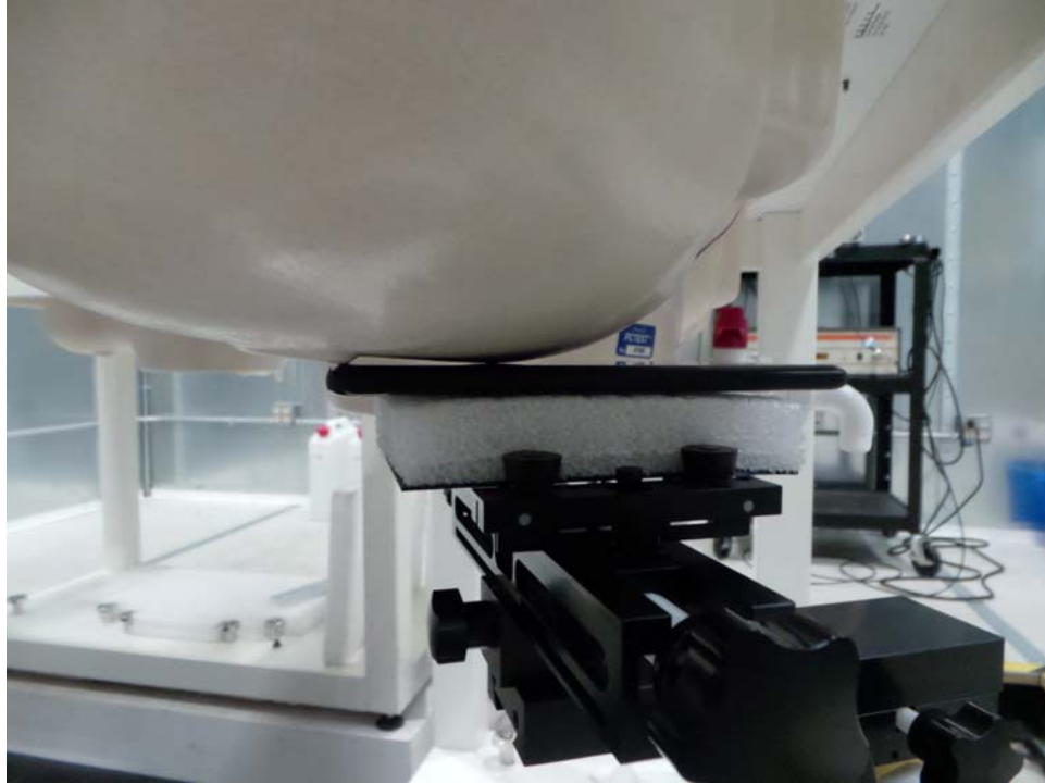
SAR Test Setup Photo 1: Right Cheek
