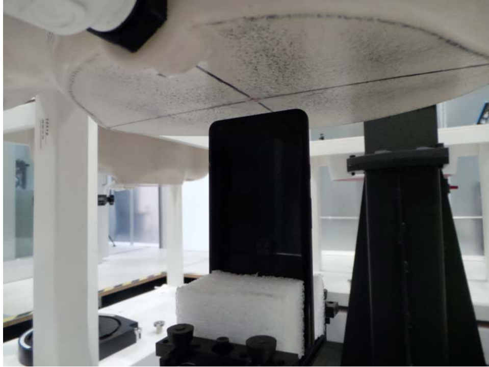
SAR Test Setup Photo 9: Top at 1.0 cm
