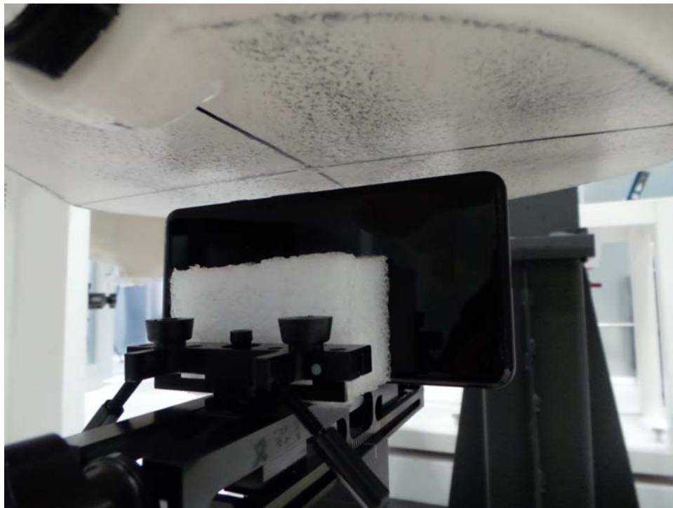
SAR Test Setup Photo 12: Right at 1.0 cm
