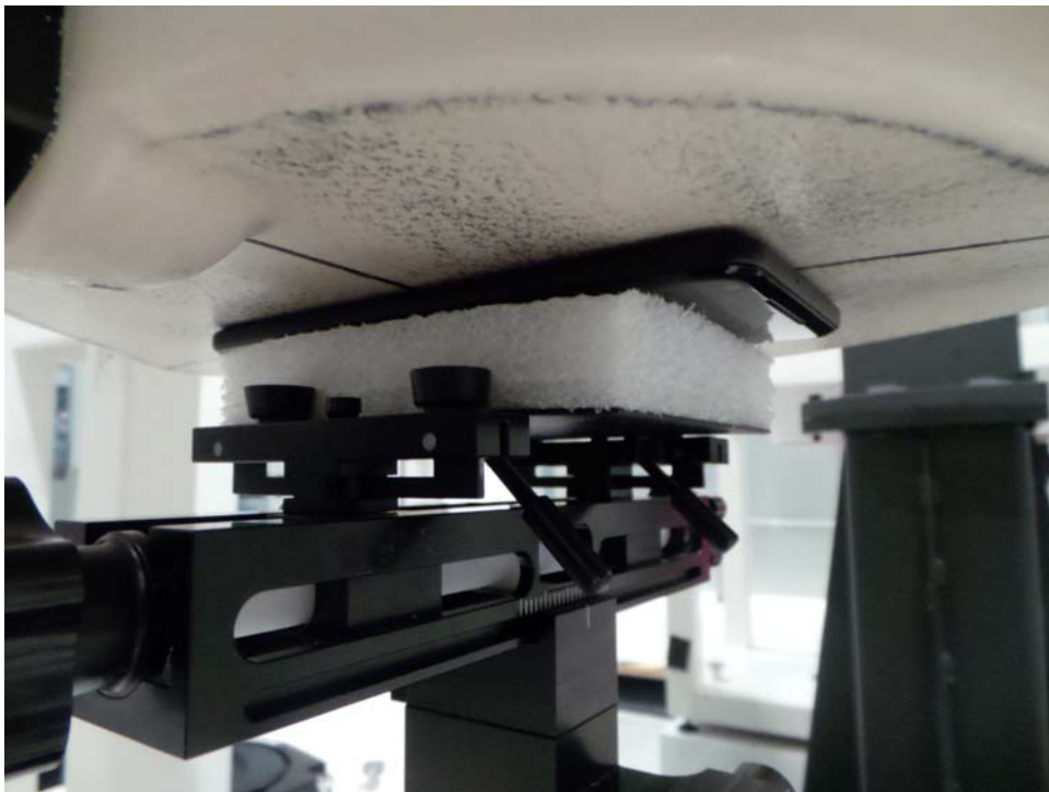
SAR Test Setup Photo 6: Back at 0.0 cm
