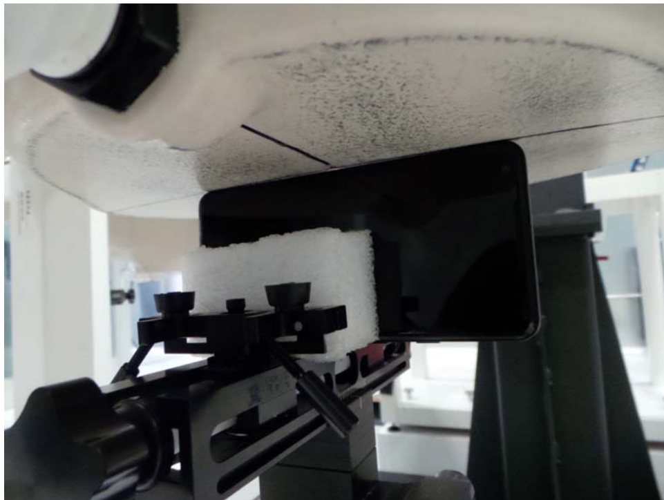
SAR Test Setup Photo 14: Left at 0.0 cm
