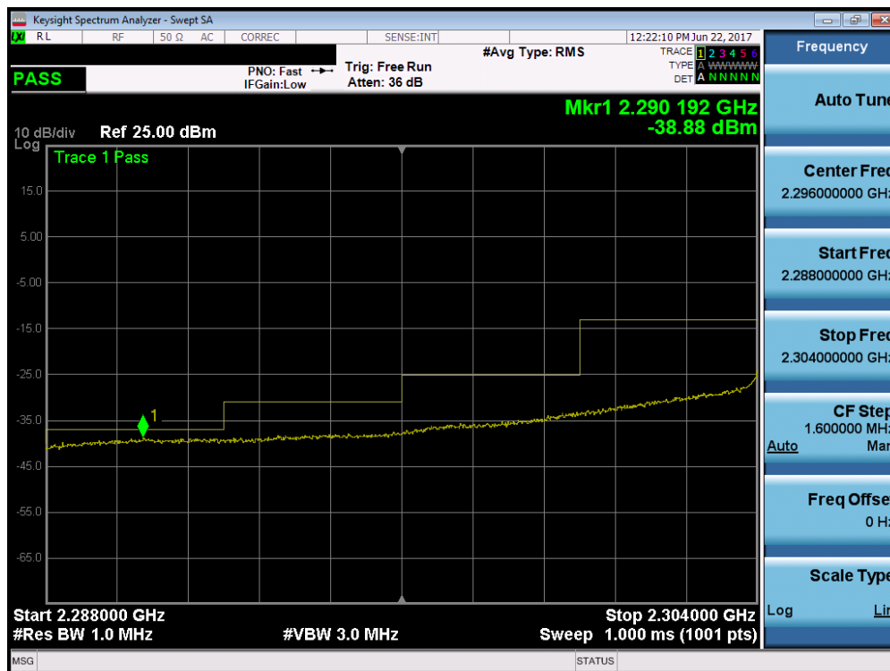
Plot 7-271. Lower Extended Band Edge Plot (Band 30 – 10.0MHz QPSK – RB Size 50)
