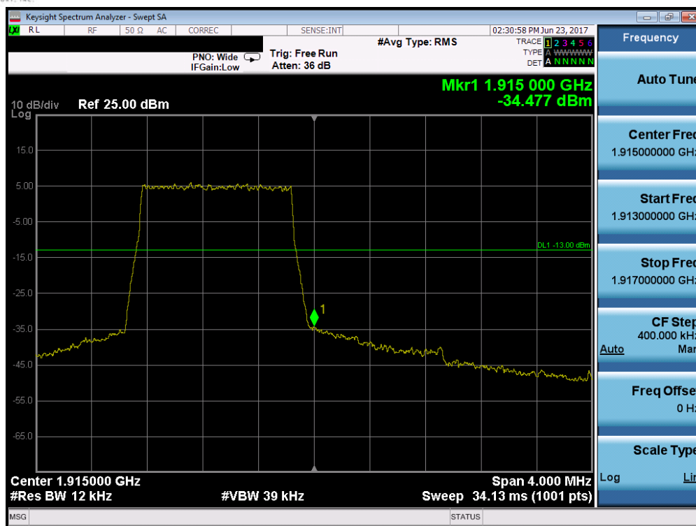
Plot 7-232. Upper Band Edge Plot (Band 25 – 1.4MHz QPSK – RB Size 6)
