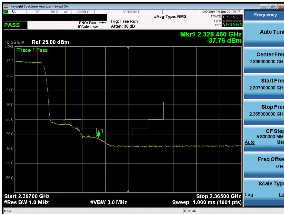
Plot 7-273. Upper Extended Band Edge Plot (Band 30 – 10.0MHz QPSK – RB Size 50)
