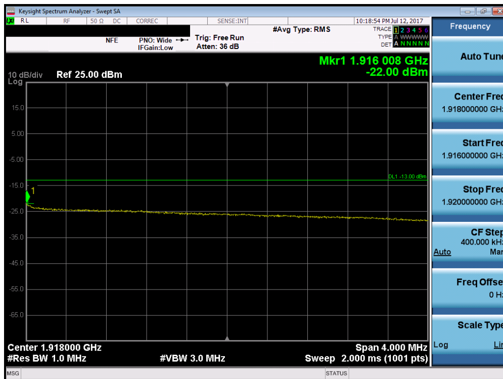
Plot 7-245. Upper Extended Band Edge Plot (Band 25 – 10.0MHz QPSK – RB Size 50)
