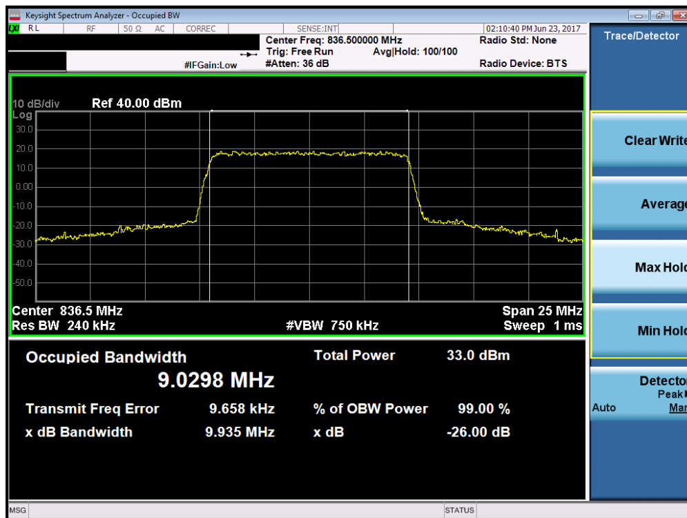
Plot 7-28. Occupied Bandwidth Plot (Band 5/26 – 10.0MHz QPSK – RB Size 50)
