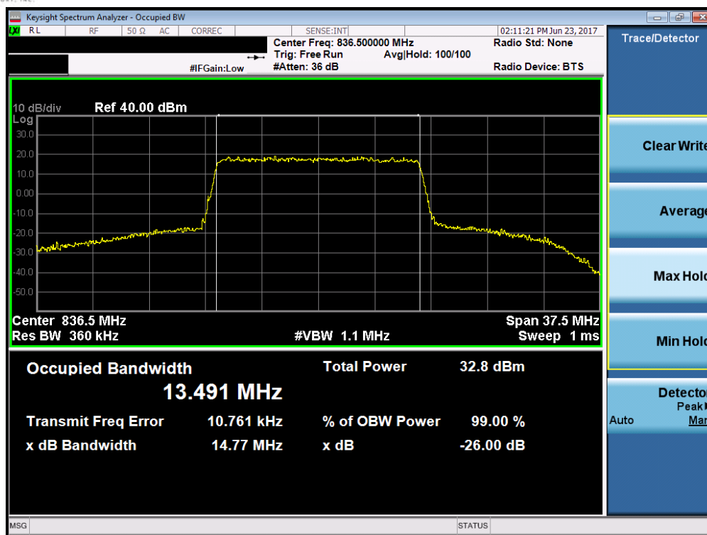
Plot 7-31. Occupied Bandwidth Plot (Band 26 – 15.0MHz QPSK – RB Size 75)
