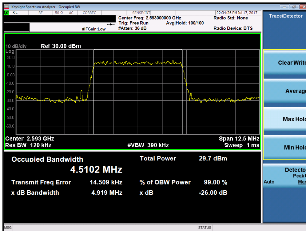
Plot 7-88. Occupied Bandwidth Plot (Band 41 – 5.0MHz QPSK – RB Size 25)
