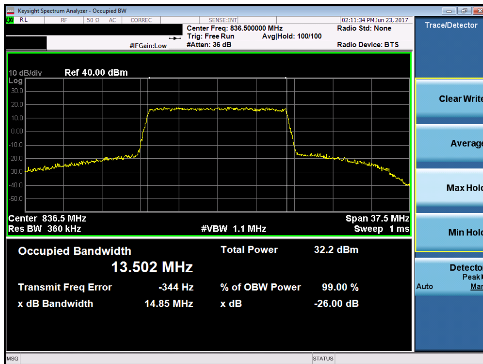
Plot 7-32. Occupied Bandwidth Plot (Band 26 – 15.0MHz 16-QAM – RB Size 75)
