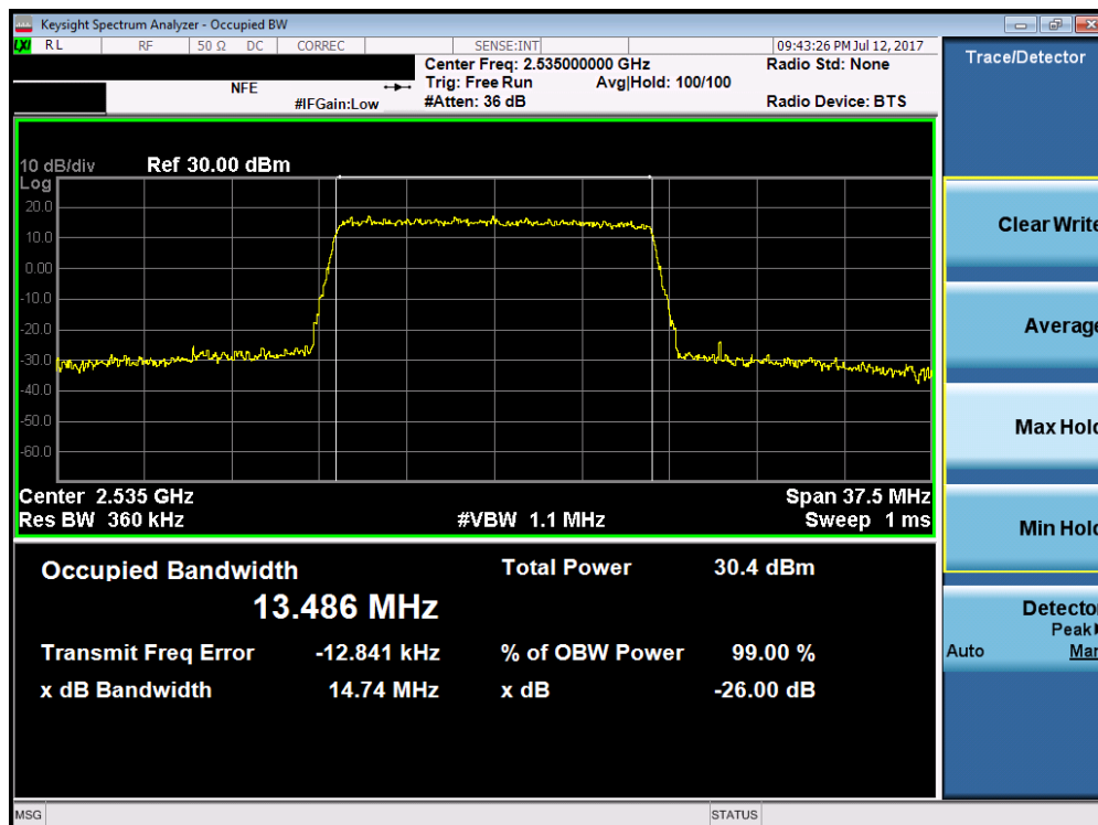
Plot 7-84. Occupied Bandwidth Plot (Band 7 – 15.0MHz 64-QAM – RB Size 75)
