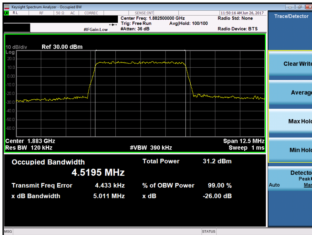
Plot 7-60. Occupied Bandwidth Plot (Band 2/25 – 5.0MHz 64-QAM – RB Size 25)
