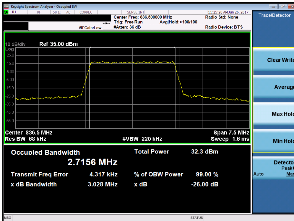
Plot 7-24. Occupied Bandwidth Plot (Band 5/26 – 3.0MHz 64-QAM – RB Size 15)
