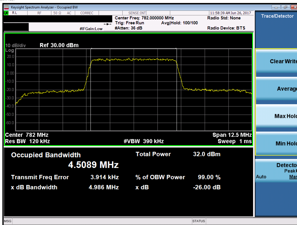
Plot 7-15. Occupied Bandwidth Plot (Band 13 – 5.0MHz 64-QAM – RB Size 25)
