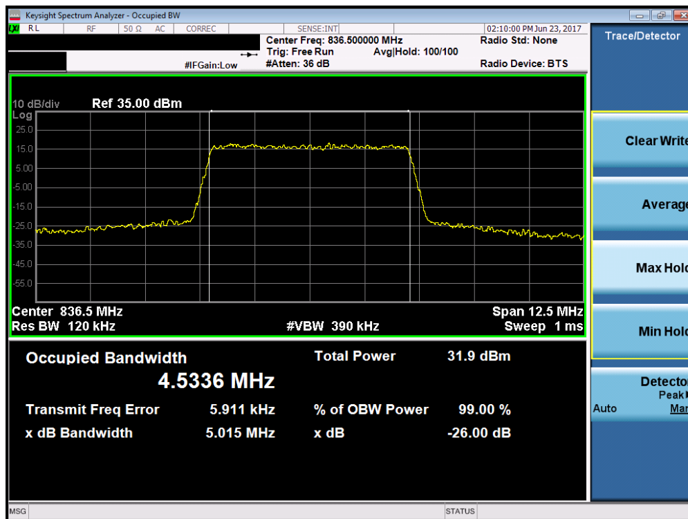
Plot 7-26. Occupied Bandwidth Plot (Band 5/26 – 5.0MHz 16-QAM – RB Size 25)
