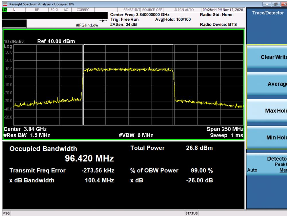
Plot 7-5. Occupied Bandwidth Plot (NR Band n77 - 100MHz 256-QAM - Full RB Configuration)
