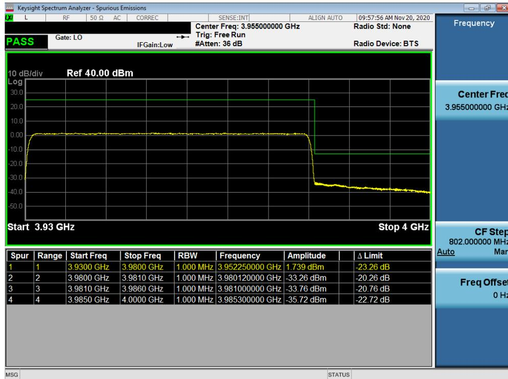
Plot 7-54. Upper Band Edge Plot (NR Band n77 - 50MHz CP-OFDM-QPSK – Full RB Configuration)
