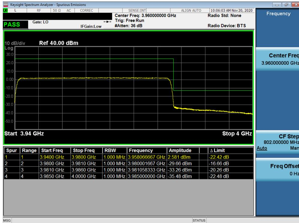
Plot 7-56. Upper Band Edge Plot (NR Band n77 - 40MHz CP-OFDM-QPSK – Full RB Configuration)
