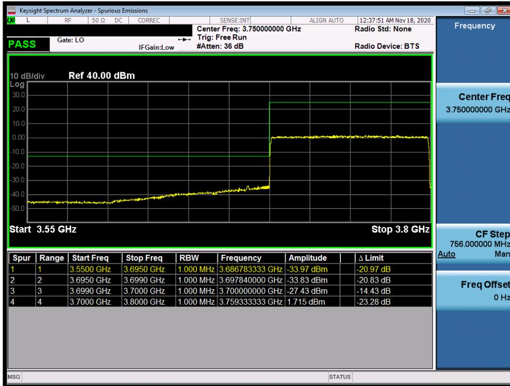
Plot 7-45. Lower Band Edge Plot (NR Band n77 - 100MHz CP-OFDM-QPSK – Full RB Configuration)
