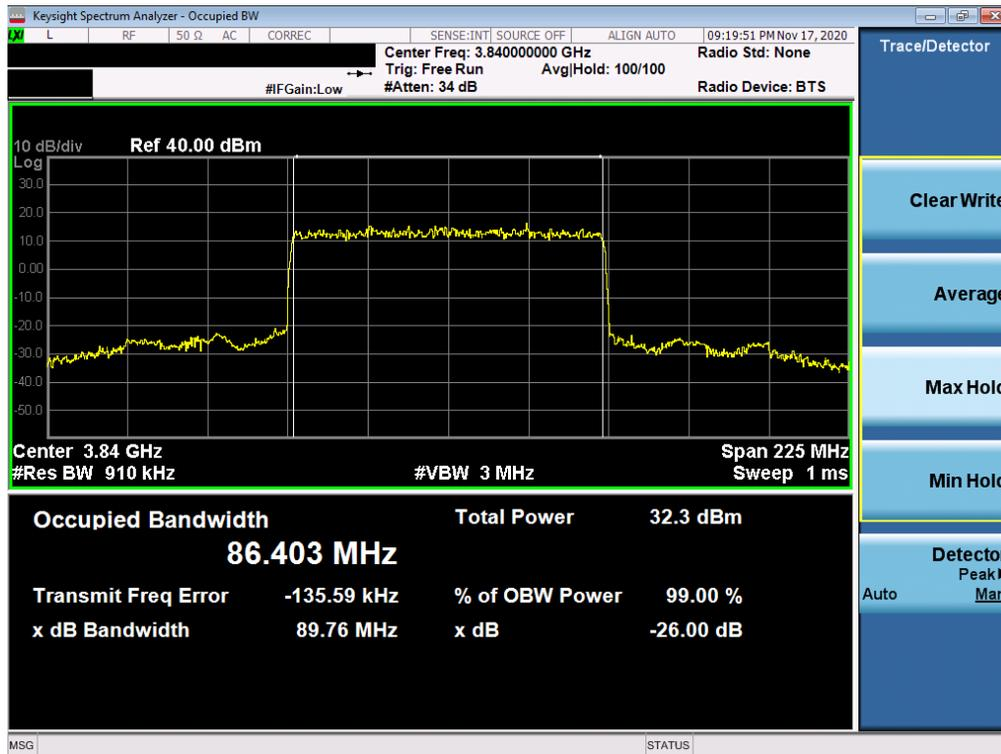
Plot 7-6. Occupied Bandwidth Plot (NR Band n77 - 90MHz  $\pi/2$  BPSK - Full RB Configuration)
