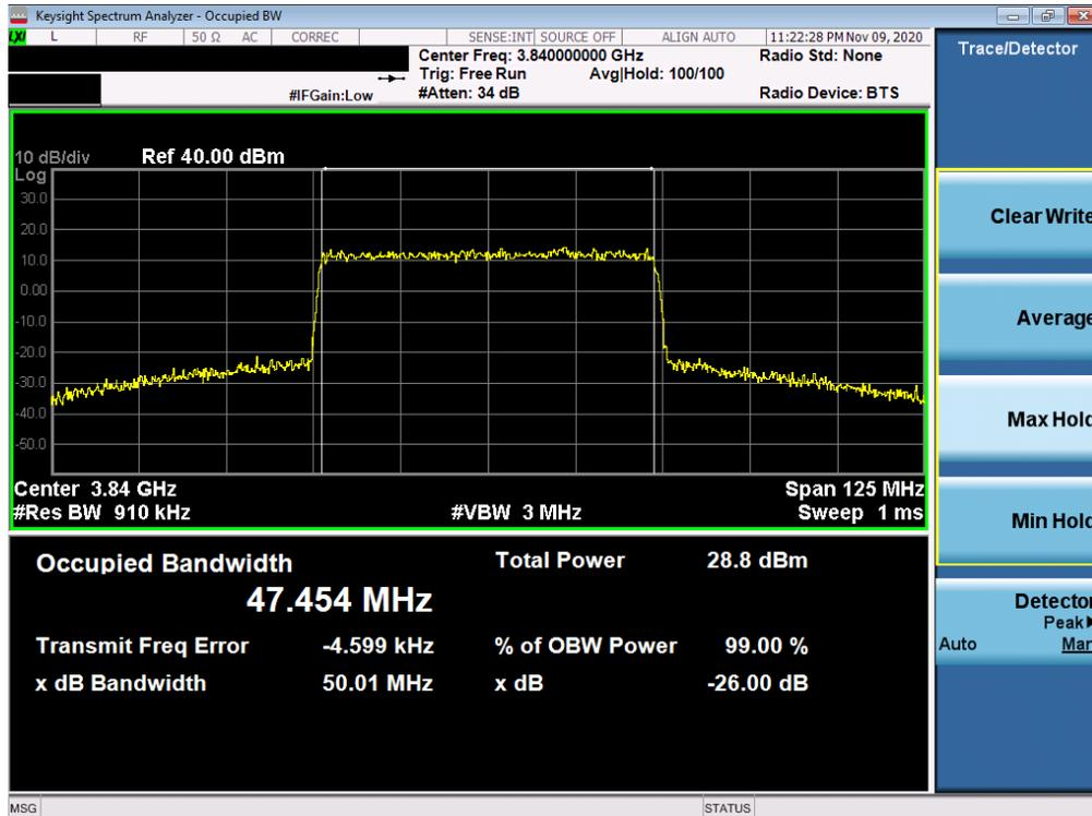
Plot 7-23. Occupied Bandwidth Plot (NR Band n77 - 50MHz 16-QAM - Full RB Configuration)
