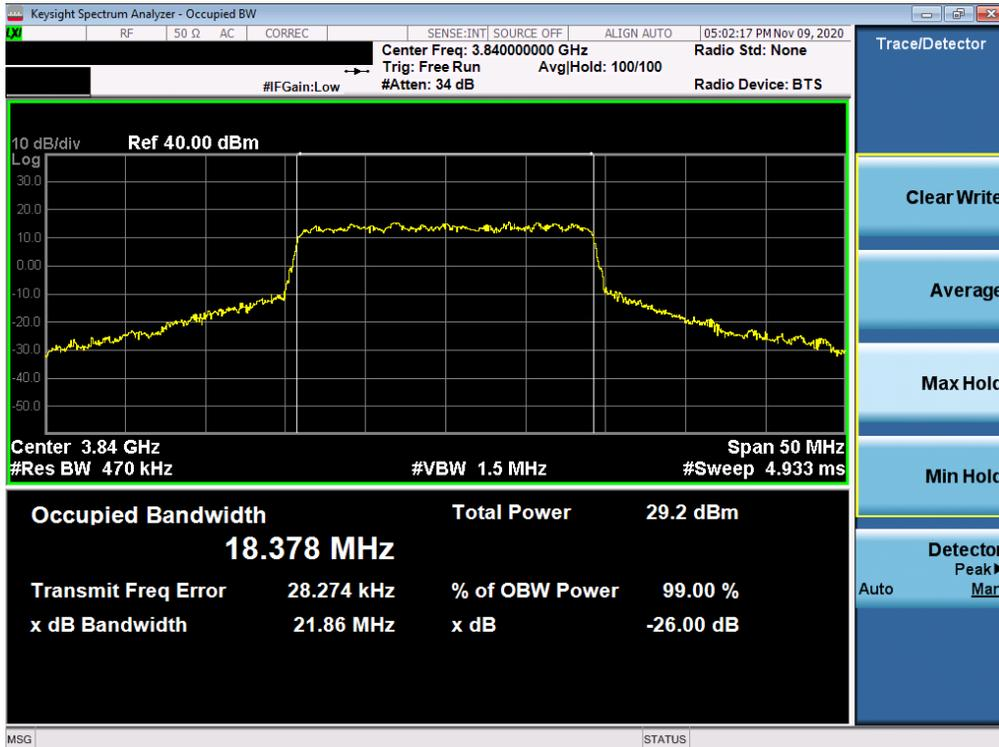
Plot 7-34. Occupied Bandwidth Plot (NR Band n77 - 20MHz 64-QAM - Full RB Configuration)
