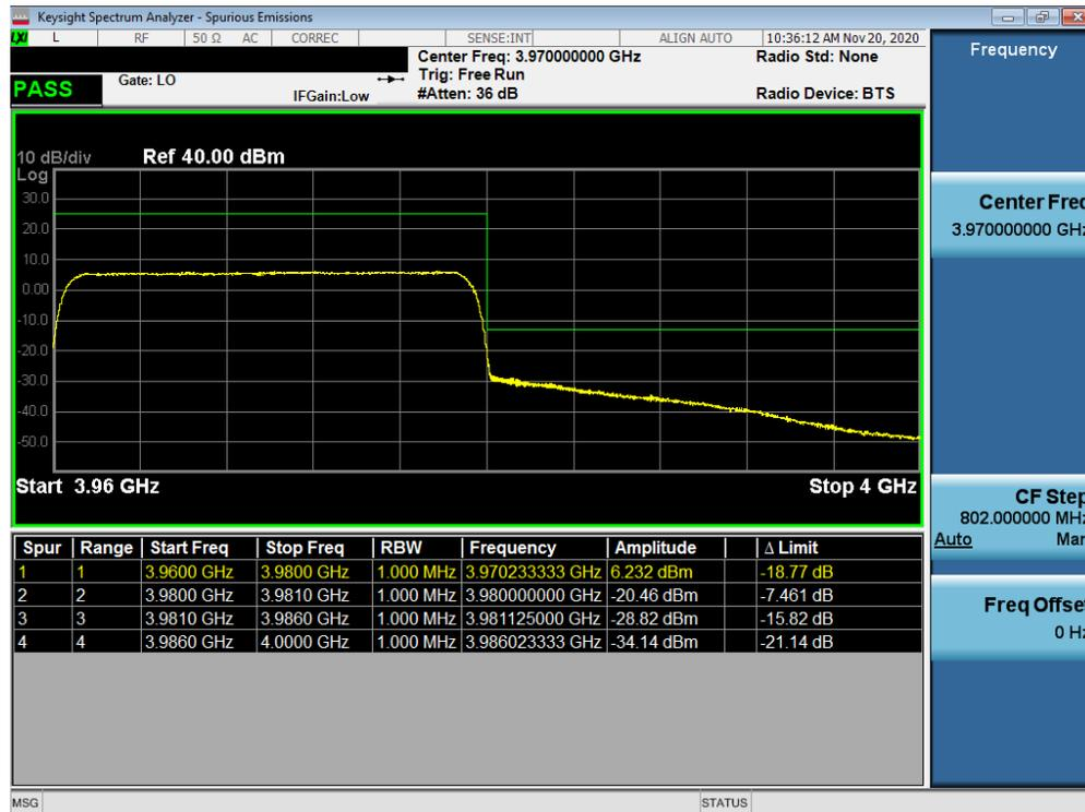
Plot 7-58. Upper Band Edge Plot (NR Band n77 - 20MHz CP-OFDM-QPSK – Full RB Configuration)
