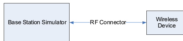
Figure 9-4 Power Measurement Setup
