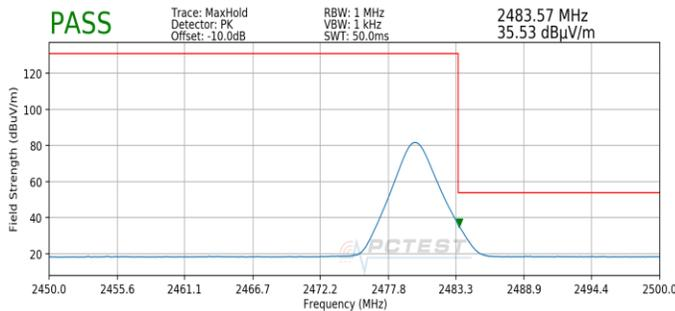
**Plot 7-48. Radiated Restricted Upper Band Edge Measurement with WCP (Average)**
