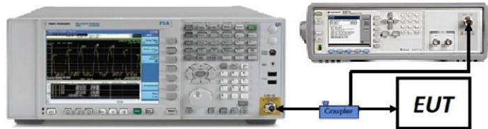
Figure 7-4. Test Instrument & Measurement Setup
