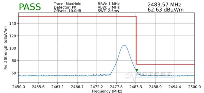
**Plot 7-49. Radiated Restricted Upper Band Edge Measurement with WCP (Peak)**
