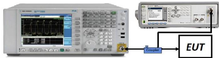
**Figure 7-7. Test Instrument & Measurement Setup**
