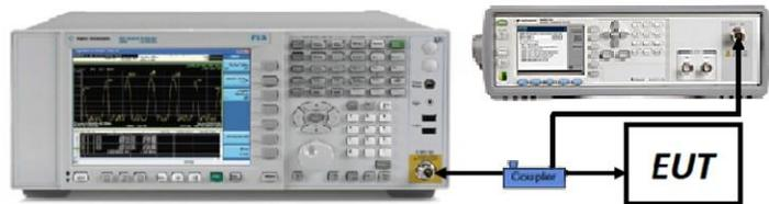
**Figure 7-2. Test Instrument & Measurement Setup**
