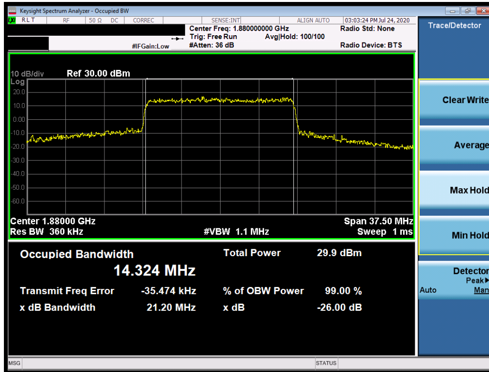
Plot 7-119. Occupied Bandwidth Plot (NR Band n2 - 15.0MHz CP-OFDM 16QAM - Full RB)
