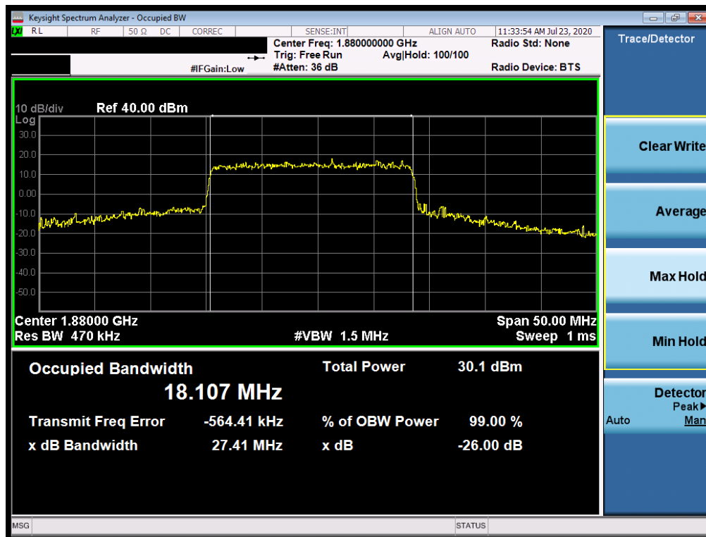
Plot 7-124. Occupied Bandwidth Plot (NR Band n2 - 20.0MHz CP-OFDM 16QAM - Full RB)
