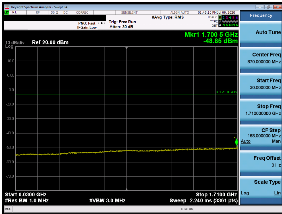
Plot 7-178. Conducted Spurious Plot (Band 66/4 - 20.0MHz QPSK - RB Size 1, RB Offset 0 - Mid Channel)
