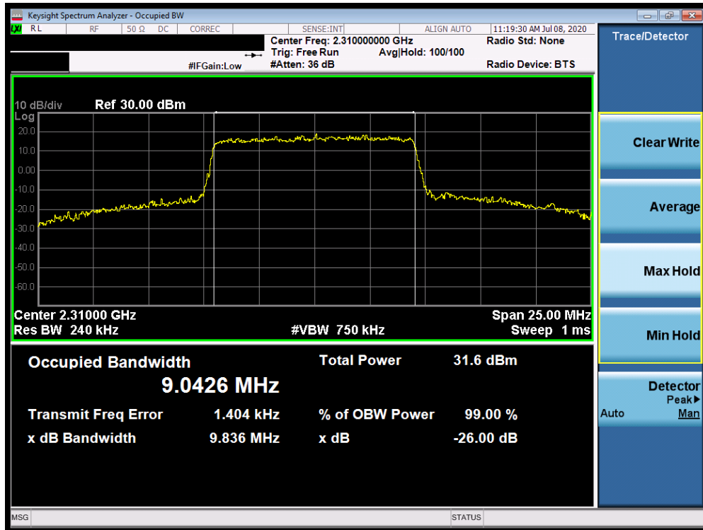
Plot 7-131. Occupied Bandwidth Plot (Band 30 - 10.0MHz 16-QAM - Full RB Configuration)
