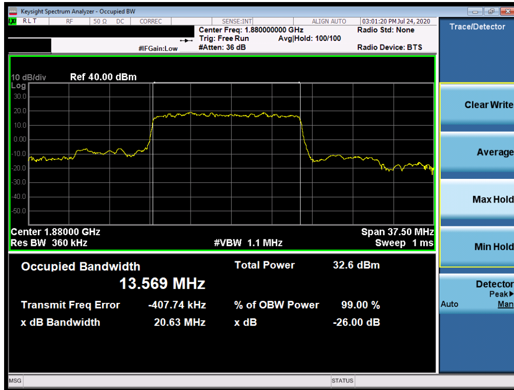
Plot 7-117. Occupied Bandwidth Plot (NR Band n2 - 15.0MHz DFT-s-OFDM BPSK - Full RB)
