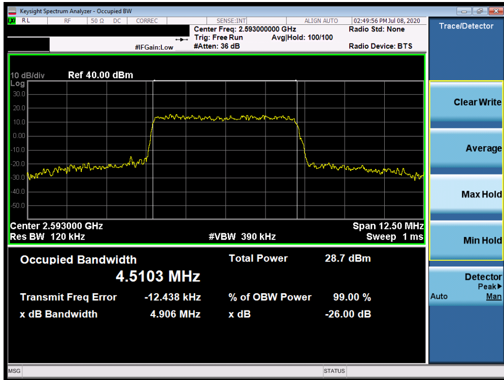
Plot 7-135. Occupied Bandwidth Plot (Band 41 – 5.0MHz 64-QAM - Full RB Configuration)
