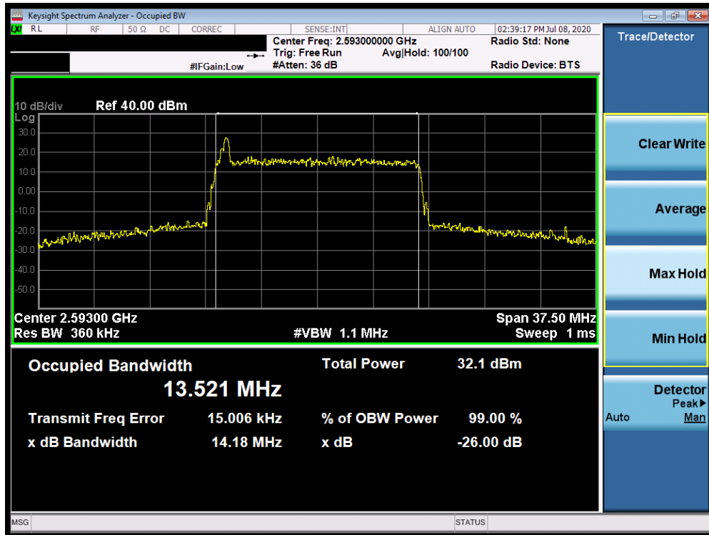
Plot 7-139. Occupied Bandwidth Plot (Band 41 - 15.0MHz QPSK - Full RB Configuration)
