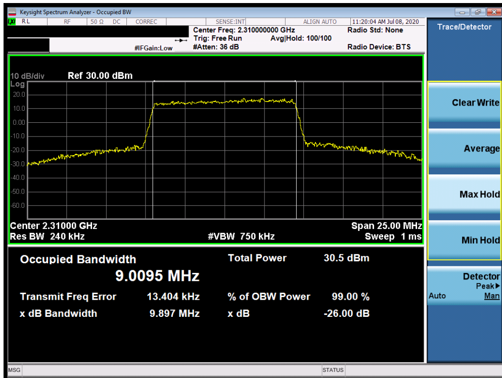
Plot 7-132. Occupied Bandwidth Plot (Band 30 - 10.0MHz 64-QAM - Full RB Configuration)
