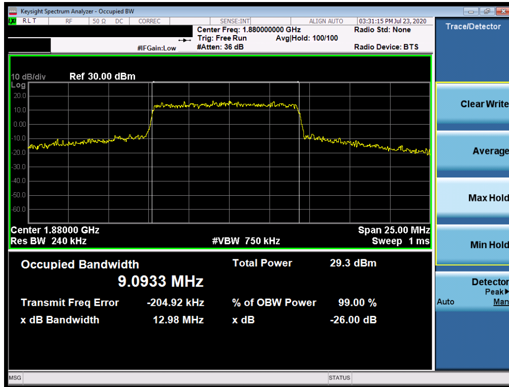
Plot 7-115. Occupied Bandwidth Plot (NR Band n2 - 10.0MHz CP-OFDM 64QAM - Full RB)
