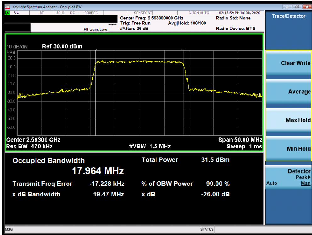
Plot 7-143. Occupied Bandwidth Plot (Band 41 - 20.0MHz 16-QAM - Full RB Configuration)
