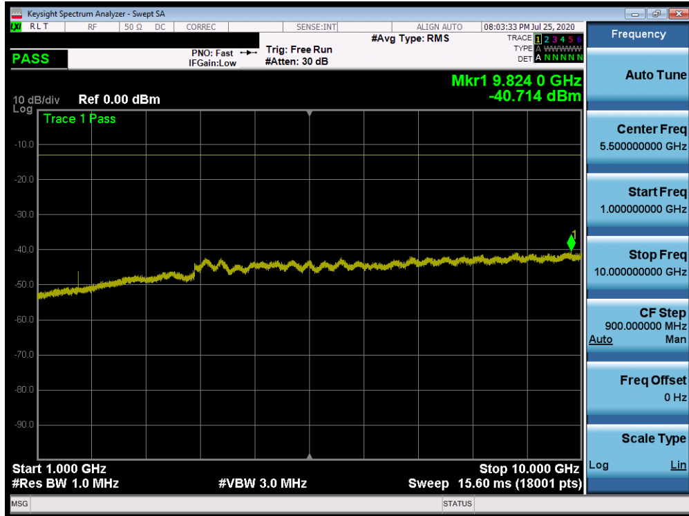
Plot 7-174. Conducted Spurious Plot (NR Band n5 - 20.0MHz - RB Size 1, RB Offset 0 - High Channel)
