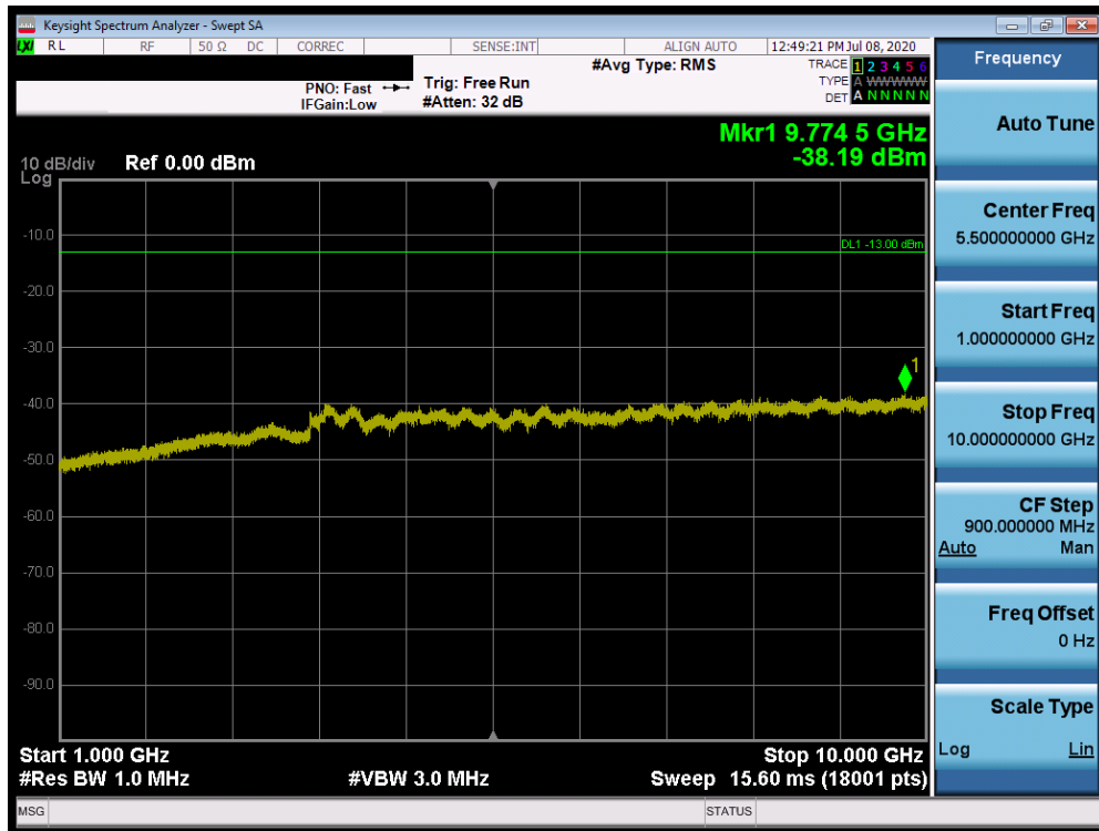
Plot 7-147. Conducted Spurious Plot (Band 12 - 10.0MHz QPSK - RB Size 1, RB Offset 0 - Low Channel)
