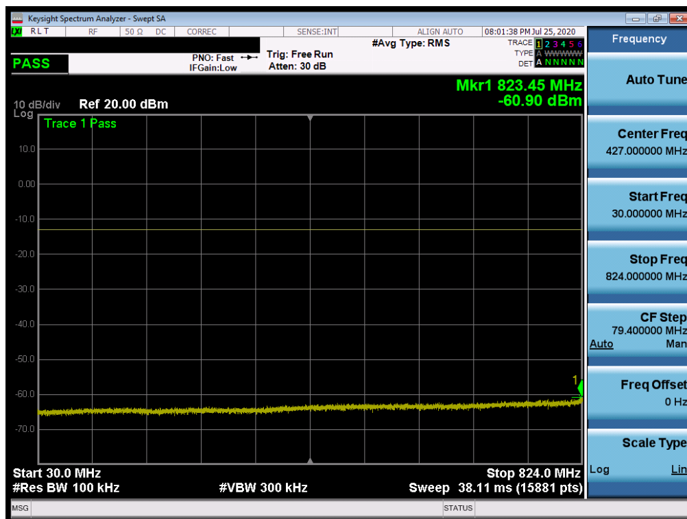
Plot 7-169. Conducted Spurious Plot (NR Band n5 - 20.0MHz - RB Size 1, RB Offset 0 - Mid Channel)
