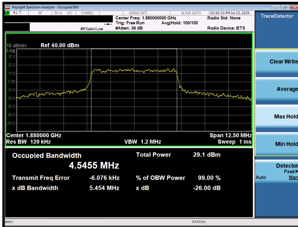
Plot 7-110. Occupied Bandwidth Plot (NR Band n2 - 5.0MHz CP-OFDM 64QAM - Full RB)
