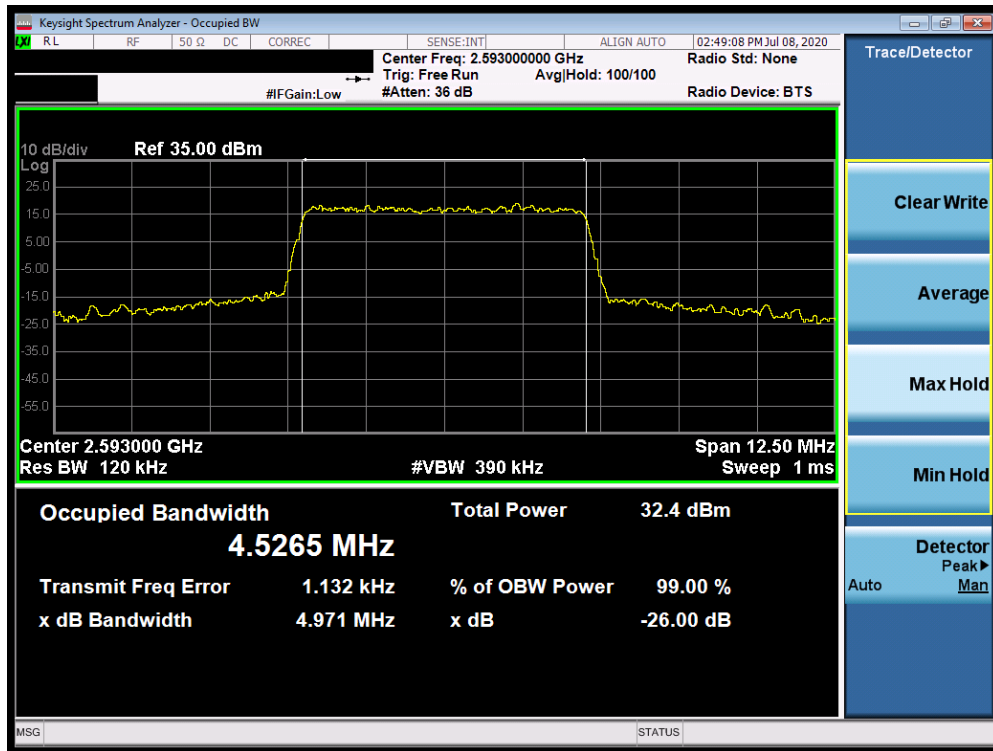
Plot 7-133. Occupied Bandwidth Plot (Band 41 – 5.0MHz QPSK - Full RB Configuration)
