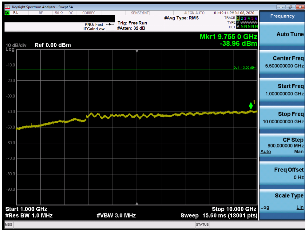
Plot 7-156. Conducted Spurious Plot (Band 13 - 10.0MHz QPSK - RB Size 1, RB Offset 0)
