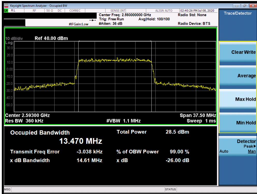
Plot 7-141. Occupied Bandwidth Plot (Band 41 - 15.0MHz 64-QAM - Full RB Configuration)
