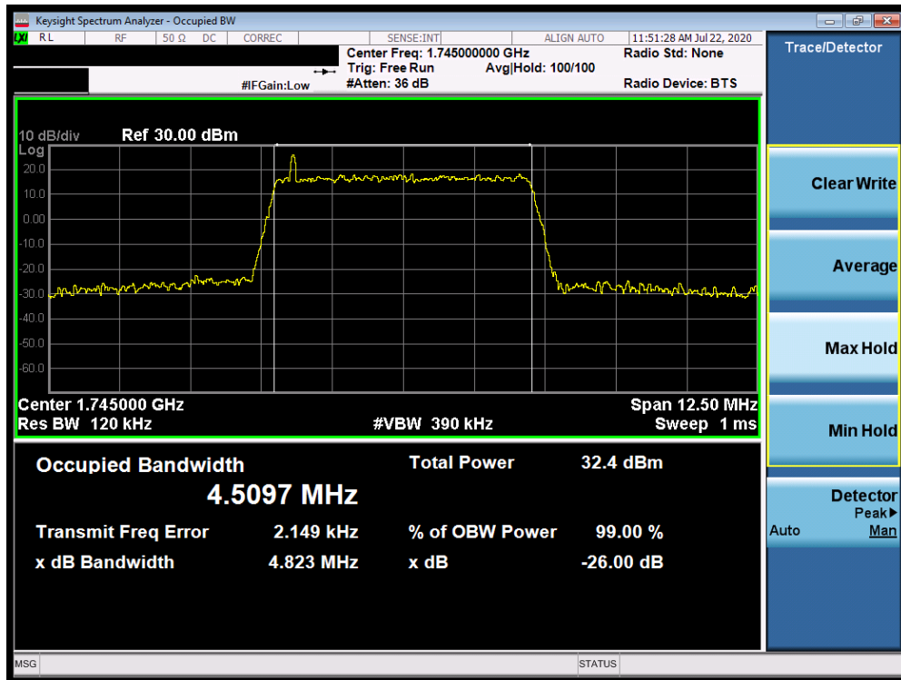
Plot 7-57. Occupied Bandwidth Plot (Band 66/4 - 5.0MHz QPSK - Full RB Configuration)
