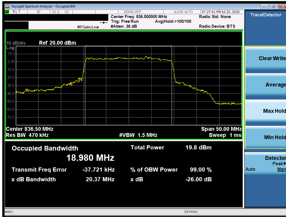
Plot 7-49. Occupied Bandwidth Plot (NR Band n5 - 20.0MHz CP-OFDM 64QAM - Full RB)
