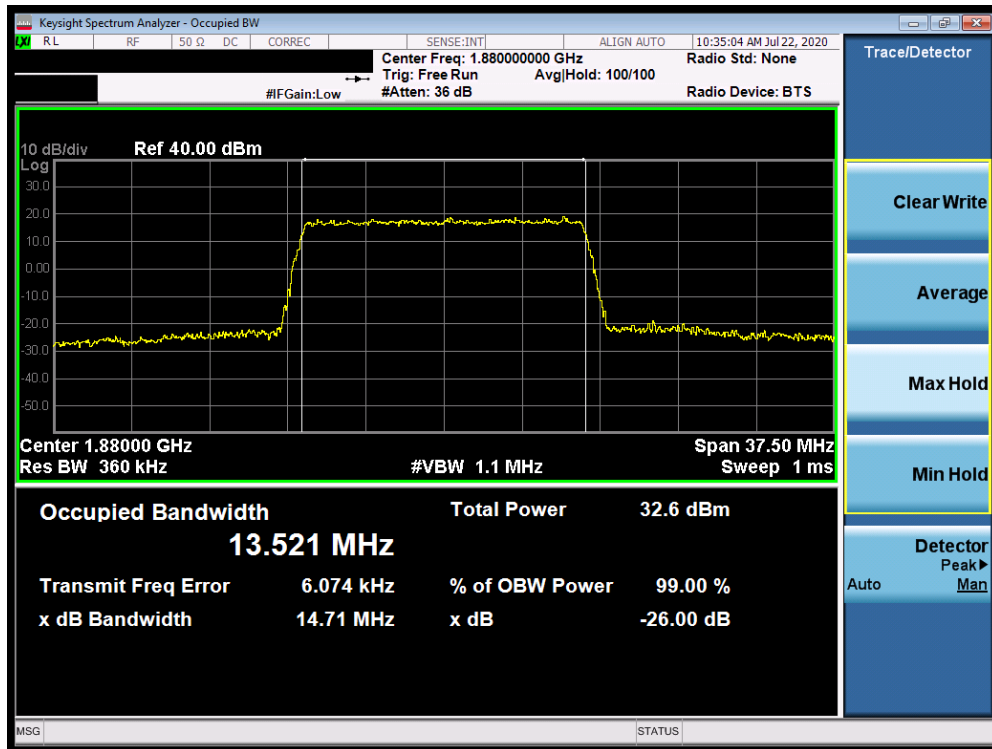
Plot 7-101. Occupied Bandwidth Plot (Band 2 - 15.0MHz QPSK - Full RB Configuration)
