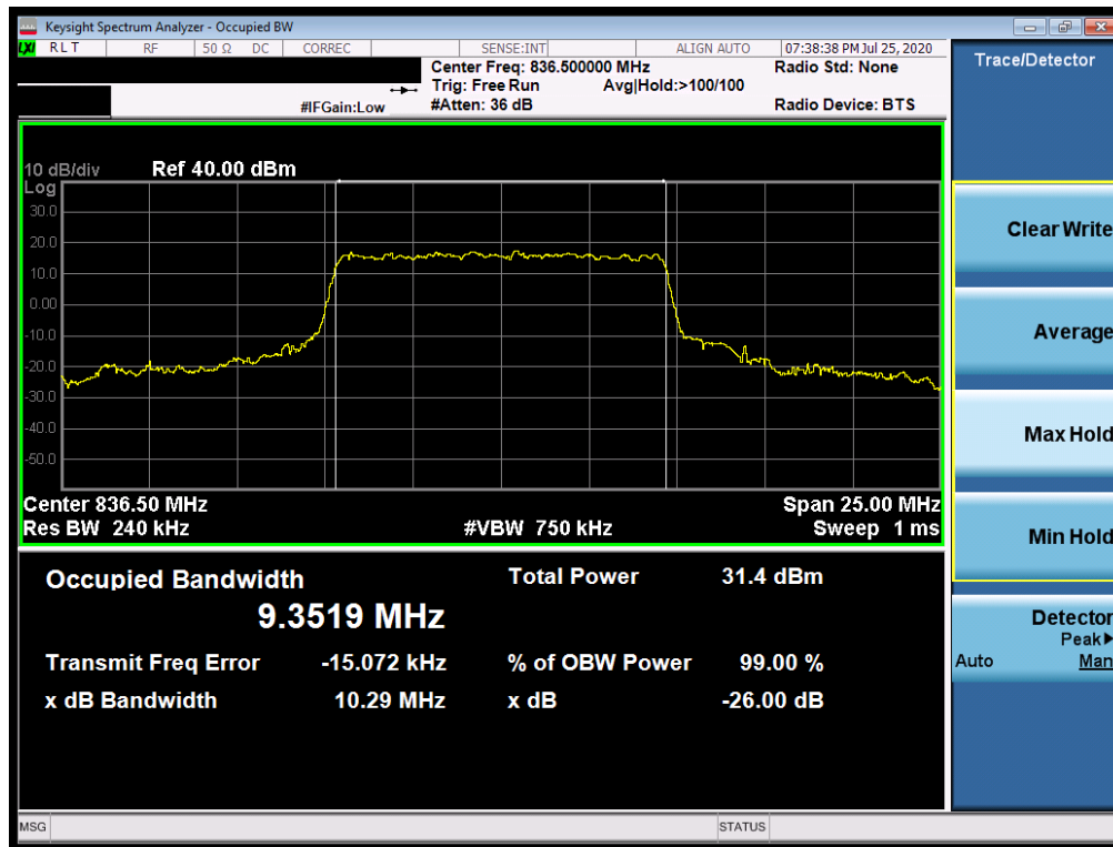
Plot 7-37. Occupied Bandwidth Plot (NR Band n5 - 10.0MHz CP-OFDM QPSK - Full RB)
