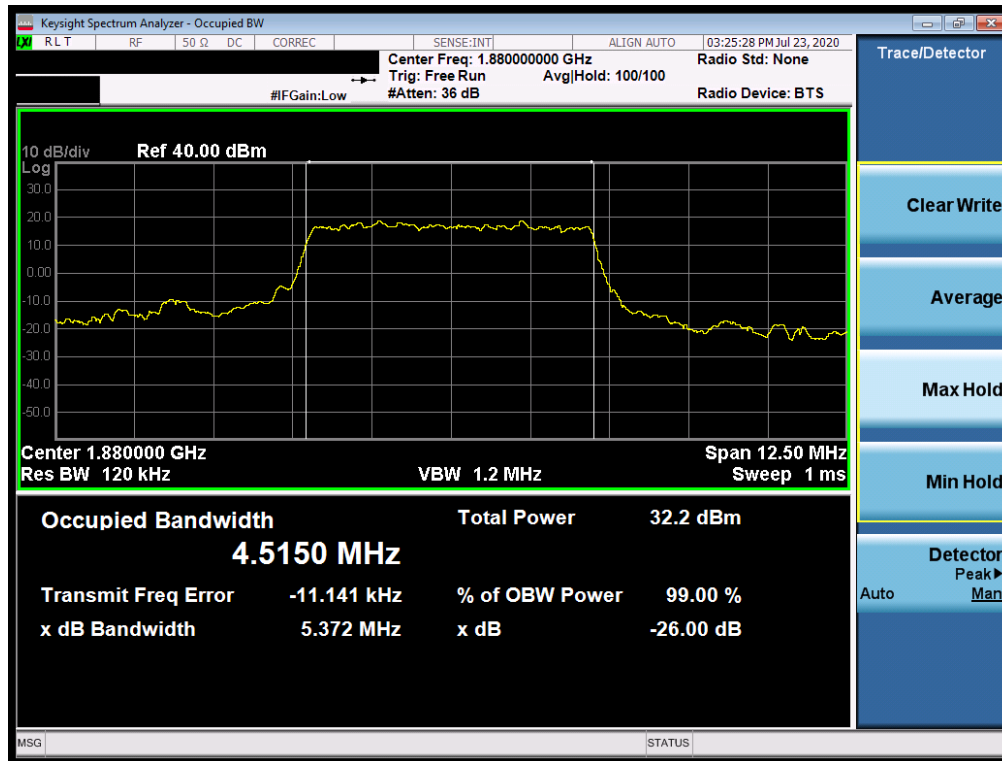
Plot 7-107. Occupied Bandwidth Plot (NR Band n2 - 5.0MHz DFT-s-OFDM BPSK - Full RB)
