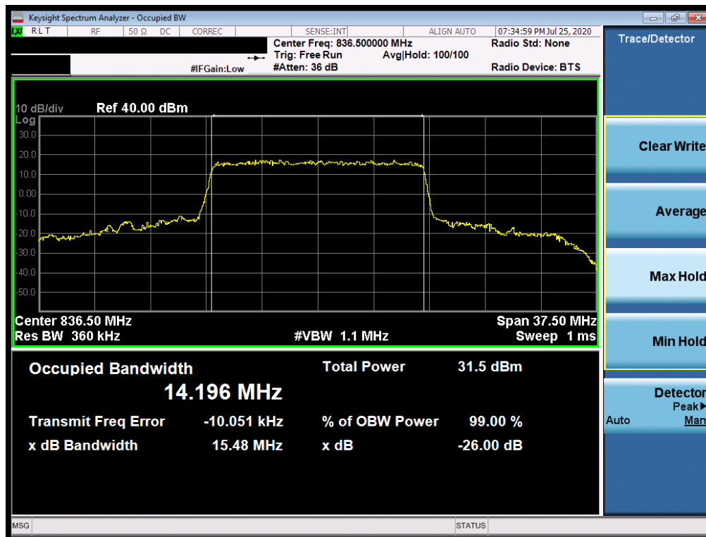
Plot 7-42. Occupied Bandwidth Plot (NR Band n5 - 15.0MHz CP-OFDM QPSK - Full RB)
