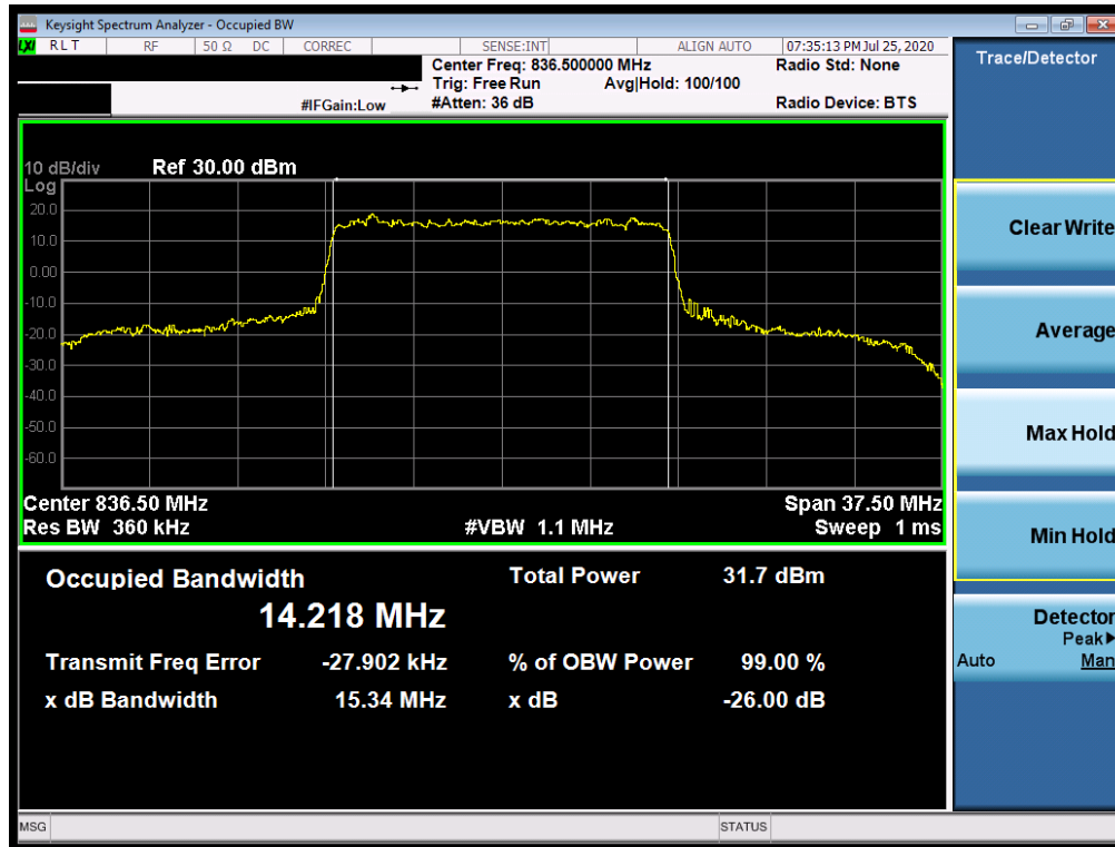
Plot 7-43. Occupied Bandwidth Plot (NR Band n5 - 15.0MHz CP-OFDM 16QAM - Full RB)
