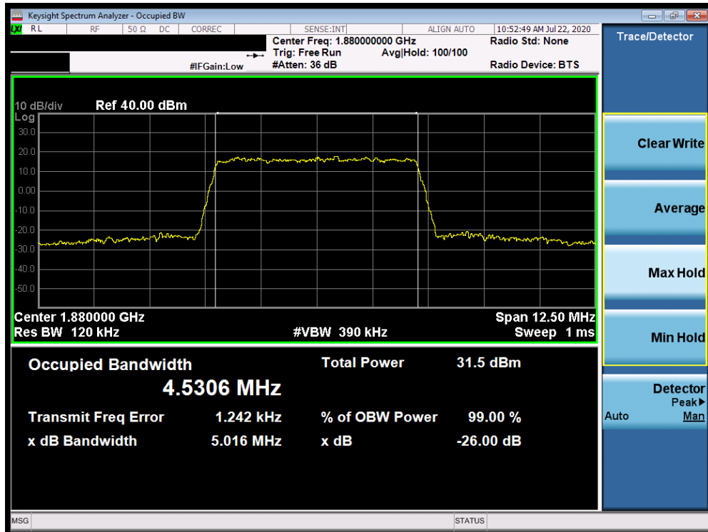
Plot 7-96. Occupied Bandwidth Plot (Band 2 - 5.0MHz 16-QAM - Full RB Configuration)
