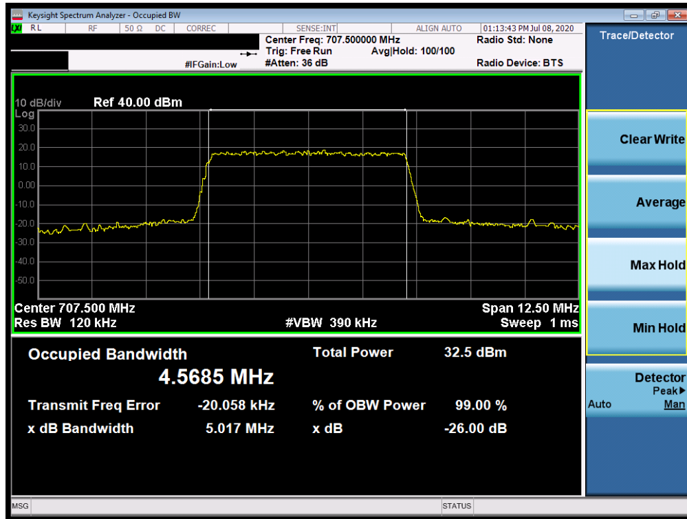
Plot 7-7. Occupied Bandwidth Plot (Band 12 - 5.0MHz QPSK - Full RB Configuration)
