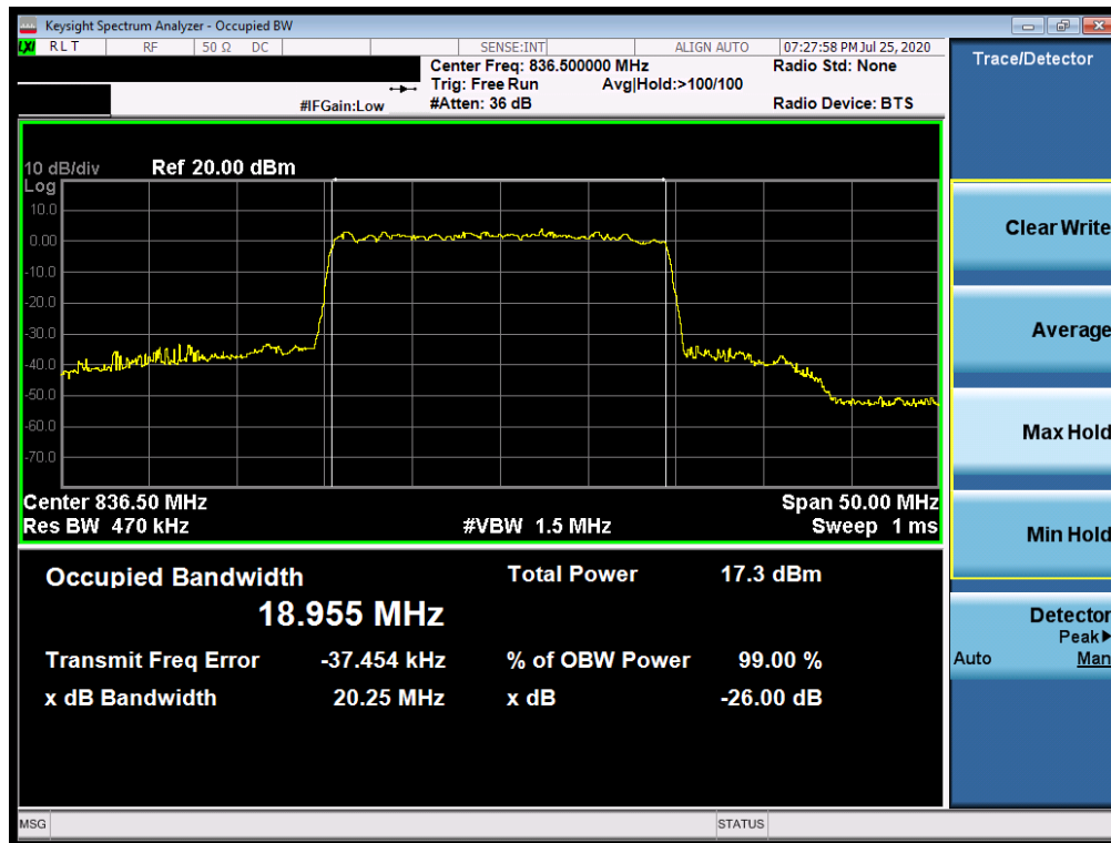
Plot 7-50. Occupied Bandwidth Plot (NR Band n5 - 20.0MHz CP-OFDM 256QAM - Full RB)
