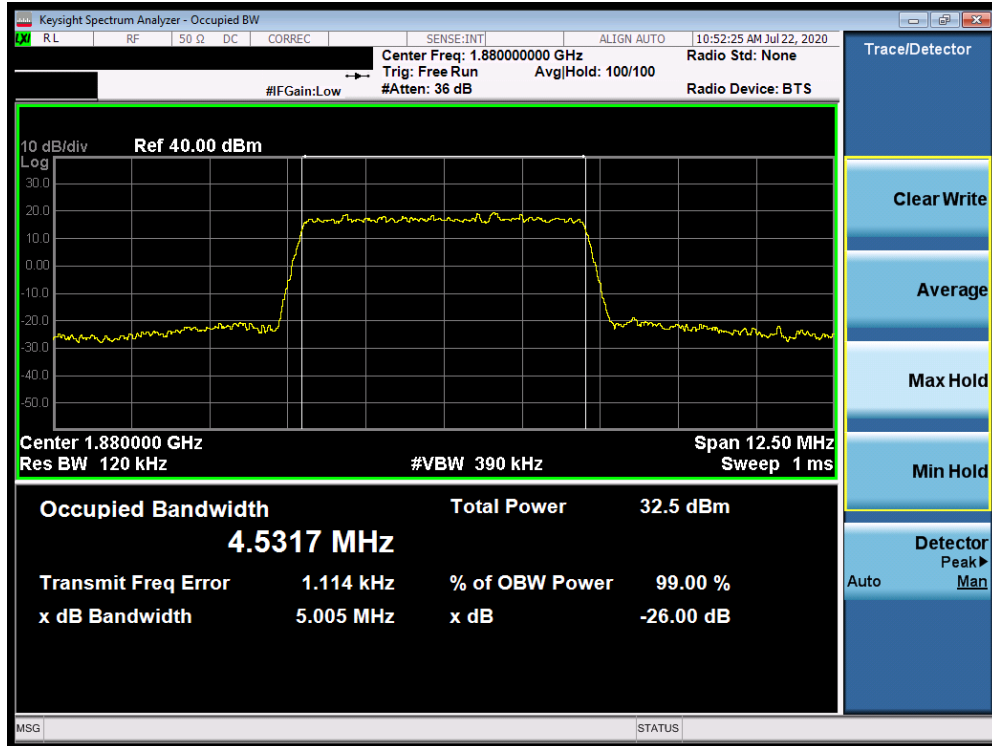
Plot 7-95. Occupied Bandwidth Plot (Band 2 - 5.0MHz QPSK - Full RB Configuration)
