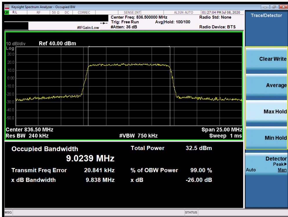
Plot 7-28. Occupied Bandwidth Plot (Band 5 - 10.0MHz QPSK - Full RB Configuration)
