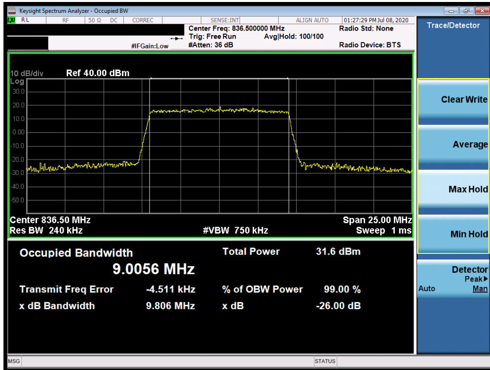
Plot 7-29. Occupied Bandwidth Plot (Band 5 - 10.0MHz 16-QAM - Full RB Configuration)
