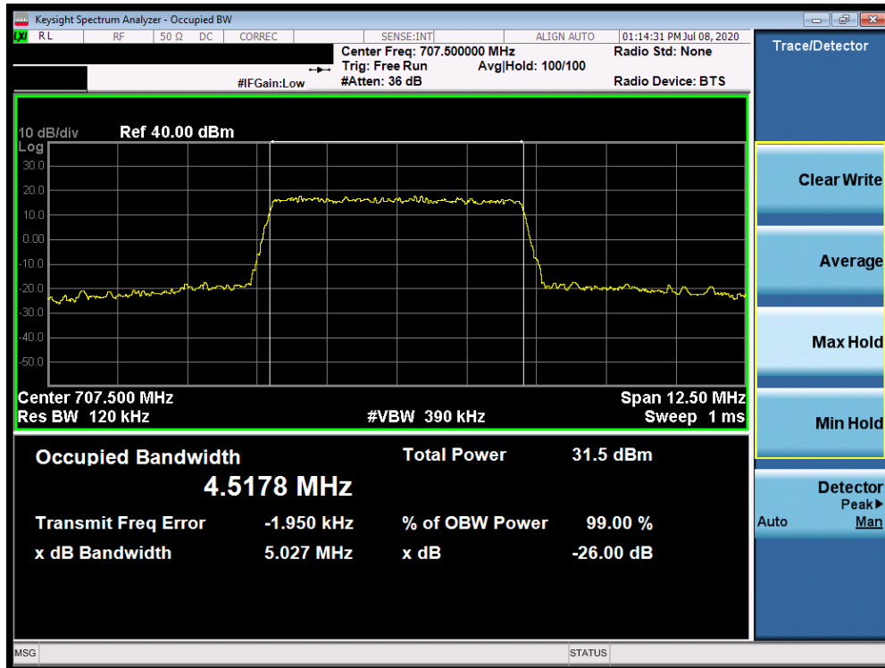
Plot 7-8. Occupied Bandwidth Plot (Band 12 - 5.0MHz 16-QAM - Full RB Configuration)
