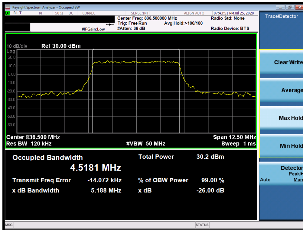
Plot 7-34. Occupied Bandwidth Plot (NR Band n5 - 5.0MHz CP-OFDM 64QAM - Full RB)
