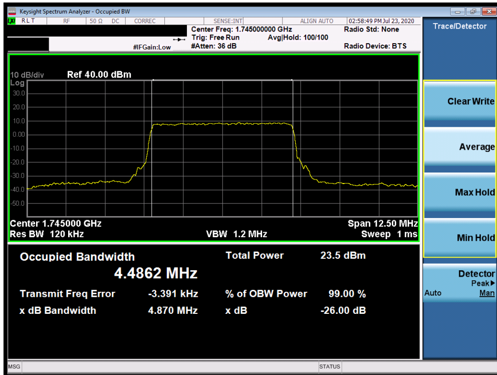
Plot 7-70. Occupied Bandwidth Plot (NR Band n66 - 5.0MHz CP-OFDM QPSK - Full RB)
