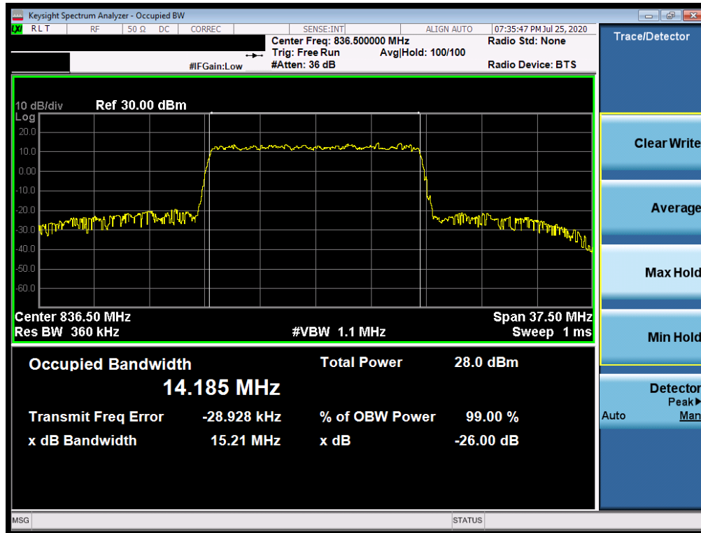
Plot 7-45. Occupied Bandwidth Plot (NR Band n5 - 15.0MHz CP-OFDM 256QAM - Full RB)
