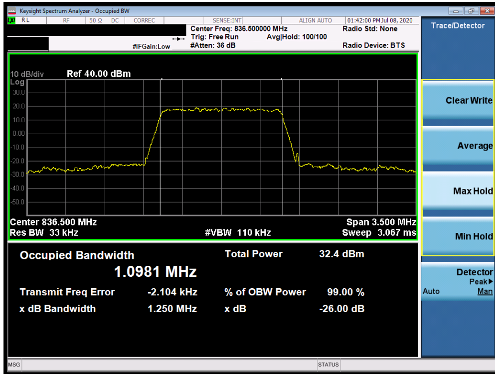
Plot 7-19. Occupied Bandwidth Plot (Band 5 - 1.4MHz QPSK - Full RB Configuration)
