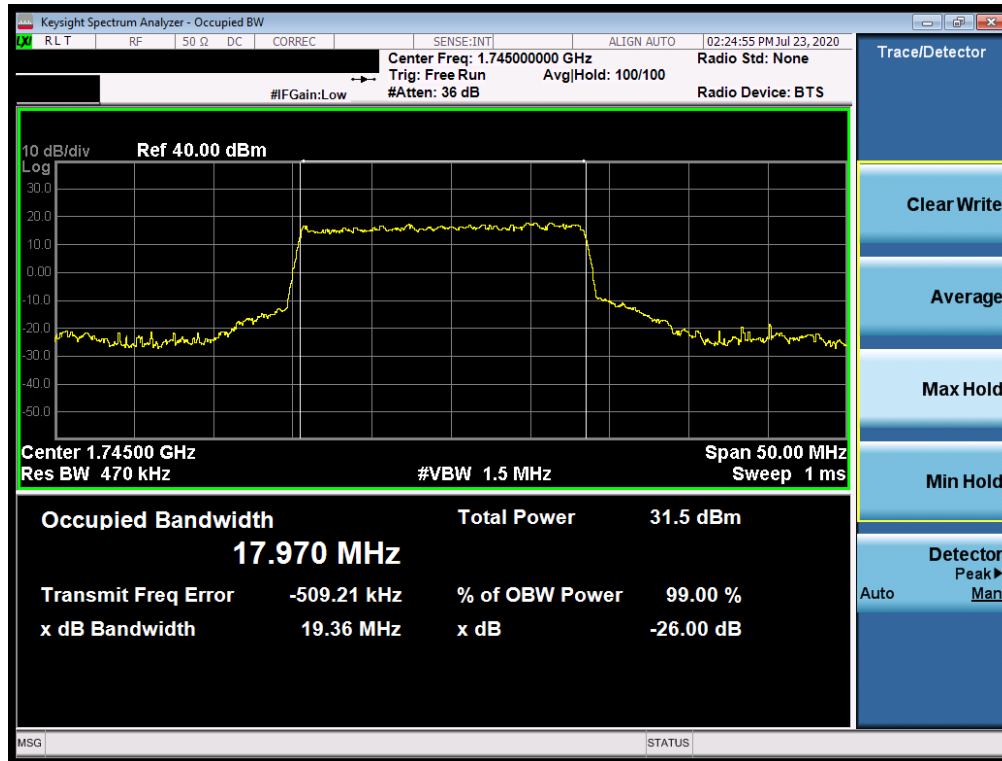
Plot 7-85. Occupied Bandwidth Plot (NR Band n66 - 20.0MHz CP-OFDM QPSK - Full RB)
