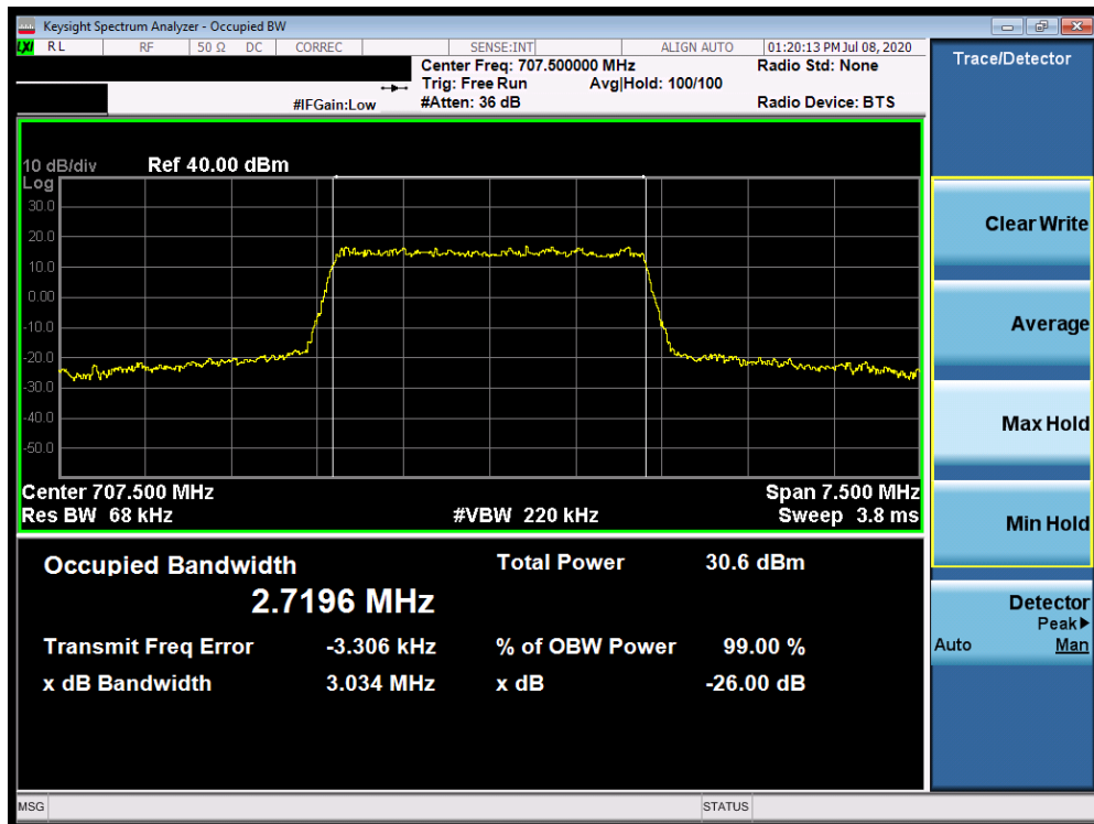
Plot 7-6. Occupied Bandwidth Plot (Band 12 - 3.0MHz 64-QAM - Full RB Configuration)
