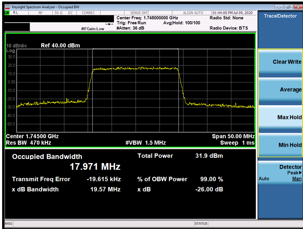
Plot 7-67. Occupied Bandwidth Plot (Band 66/4 - 20.0MHz 16-QAM - Full RB Configuration)
