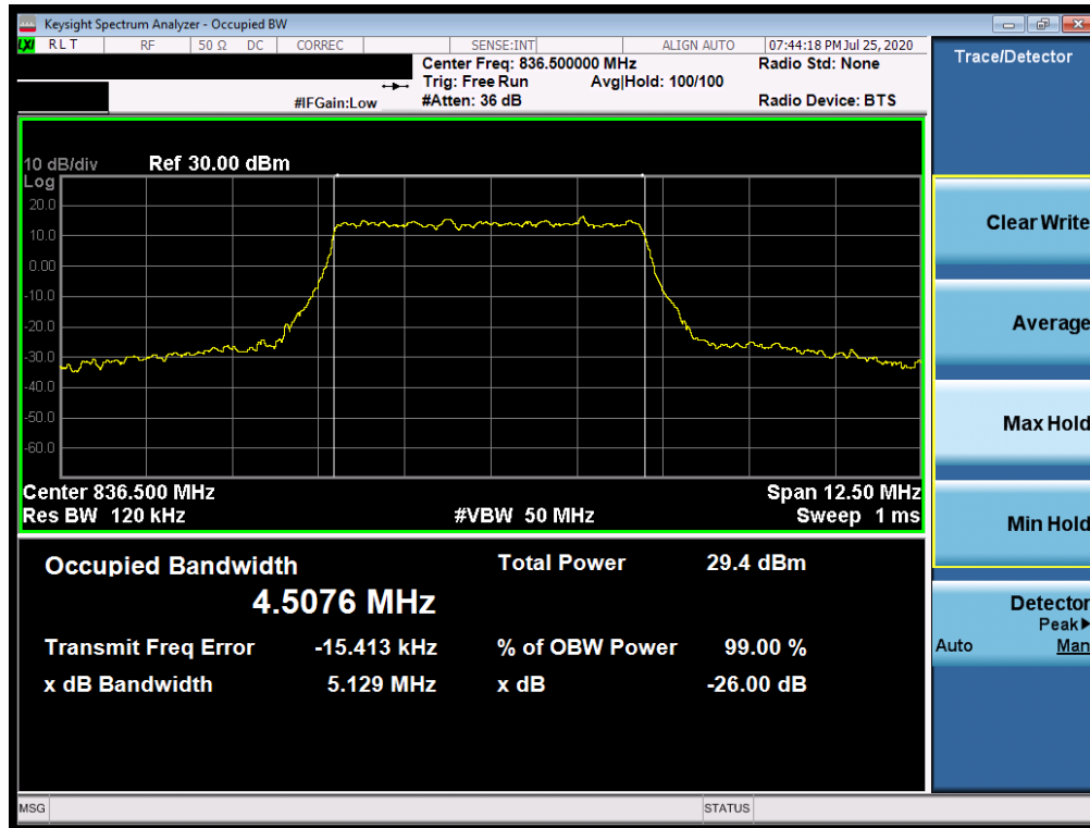
Plot 7-35. Occupied Bandwidth Plot (NR Band n5 - 5.0MHz CP-OFDM 256QAM - Full RB)
