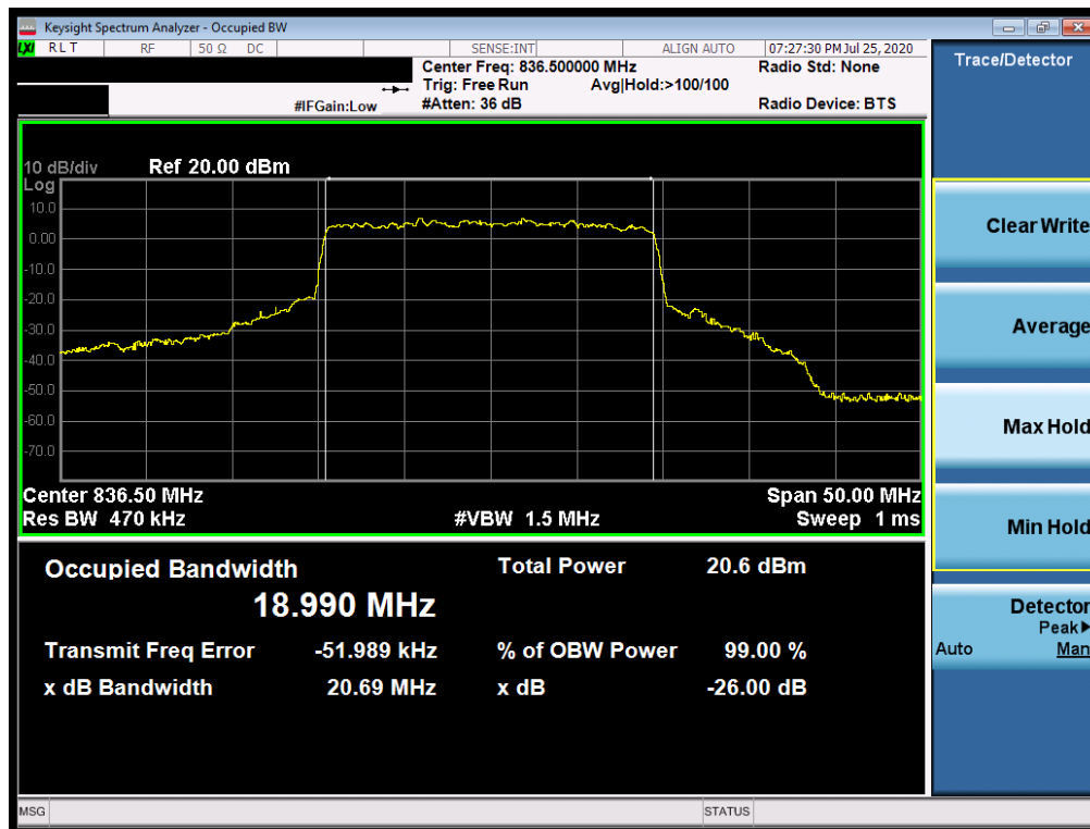
Plot 7-48. Occupied Bandwidth Plot (NR Band n5 - 20.0MHz CP-OFDM 16QAM - Full RB)
