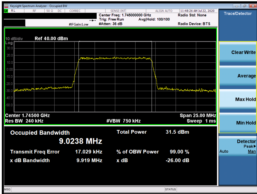
Plot 7-61. Occupied Bandwidth Plot (Band 66/4 - 10.0MHz 16-QAM - Full RB Configuration)
