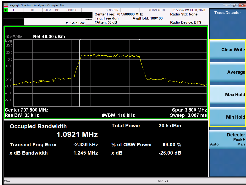
Plot 7-3. Occupied Bandwidth Plot (Band 12 - 1.4.0MHz 64-QAM - Full RB Configuration)
