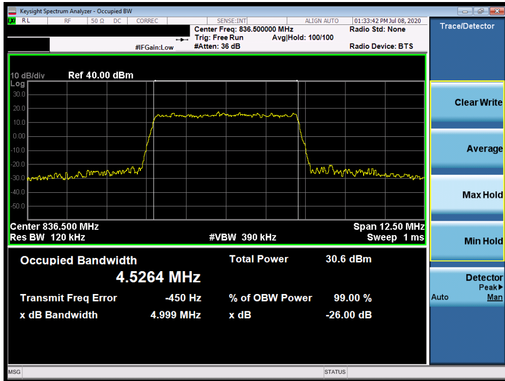
Plot 7-27. Occupied Bandwidth Plot (Band 5 - 5.0MHz 64-QAM - Full RB Configuration)
