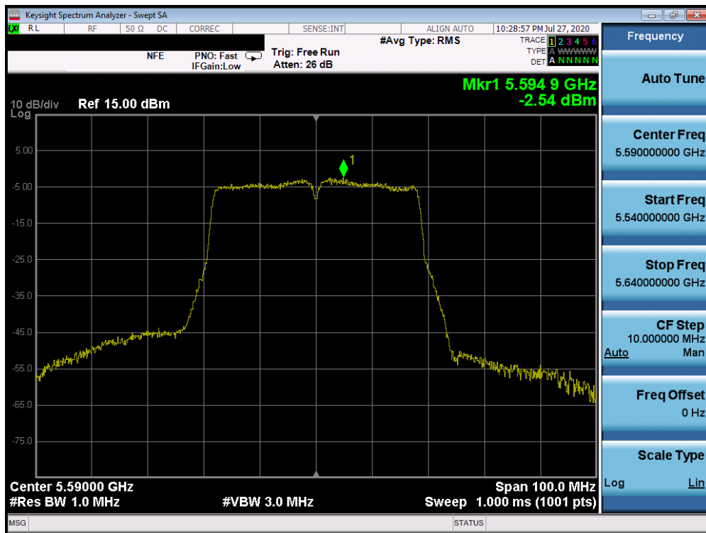
Plot 7-143. Power Spectral Density Plot SISO ANT2 (40MHz BW 802.11n (UNII Band 2C) – Ch. 118)
