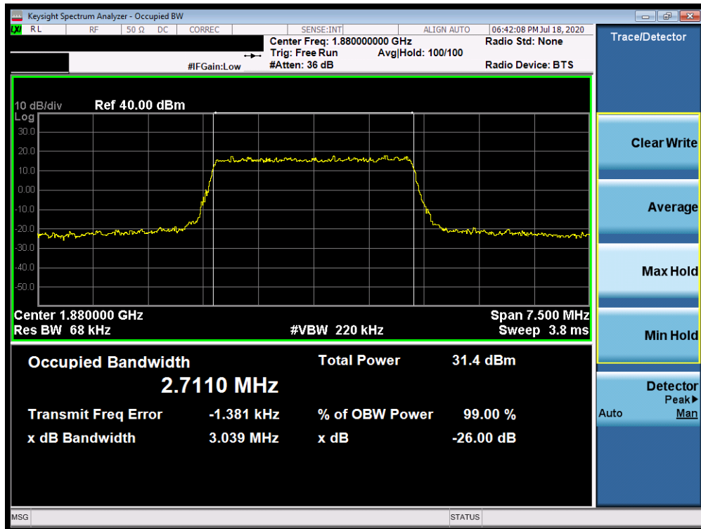
Plot 7-129. Occupied Bandwidth Plot (Band 25/2 - 3.0MHz 64-QAM - Full RB Configuration)
