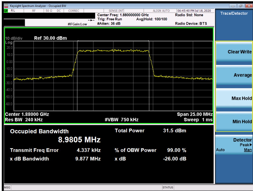
Plot 7-135. Occupied Bandwidth Plot (Band 25/2 - 10.0MHz 64-QAM - Full RB Configuration)
