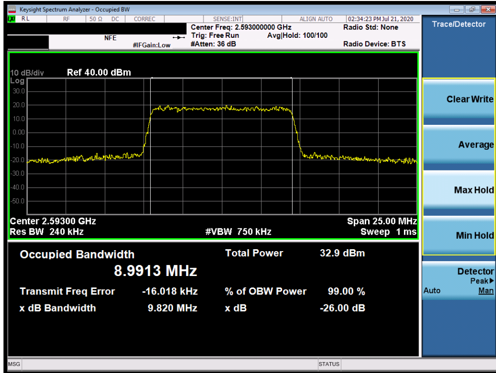
Plot 7-166. Occupied Bandwidth Plot (Band 41 - 10.0MHz 16-QAM - Full RB Configuration)
