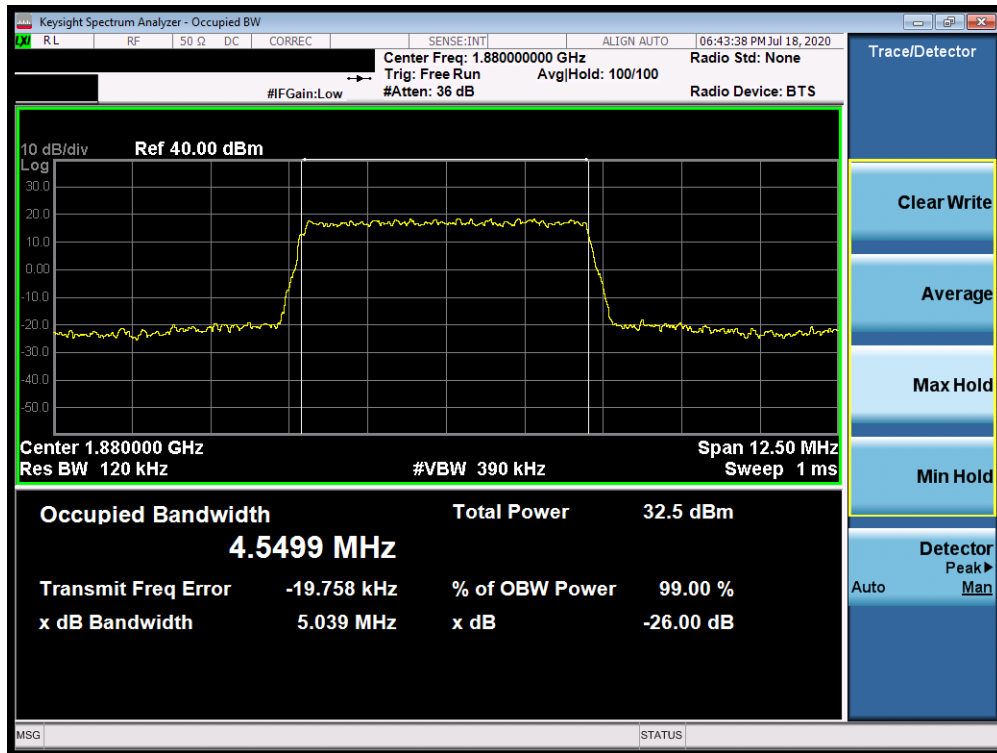
Plot 7-132. Occupied Bandwidth Plot (Band 25/2 - 5.0MHz 64-QAM - Full RB Configuration)
