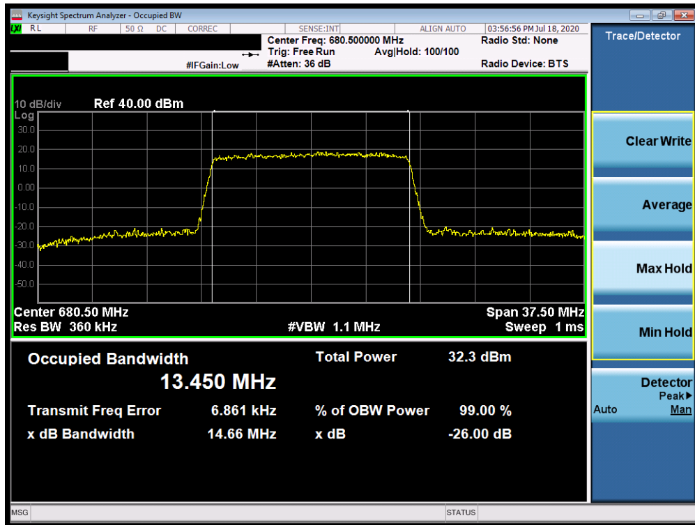
Plot 7-9. Occupied Bandwidth Plot (Band 71 - 15.0MHz 64-QAM - Full RB Configuration)
