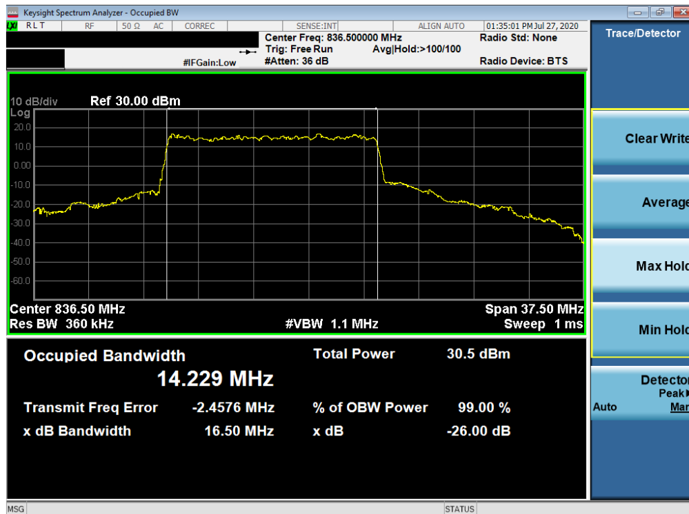
Plot 7-79. Occupied Bandwidth Plot (NR Band n5 - 15.0MHz CP-OFDM 64QAM - Full RB)
