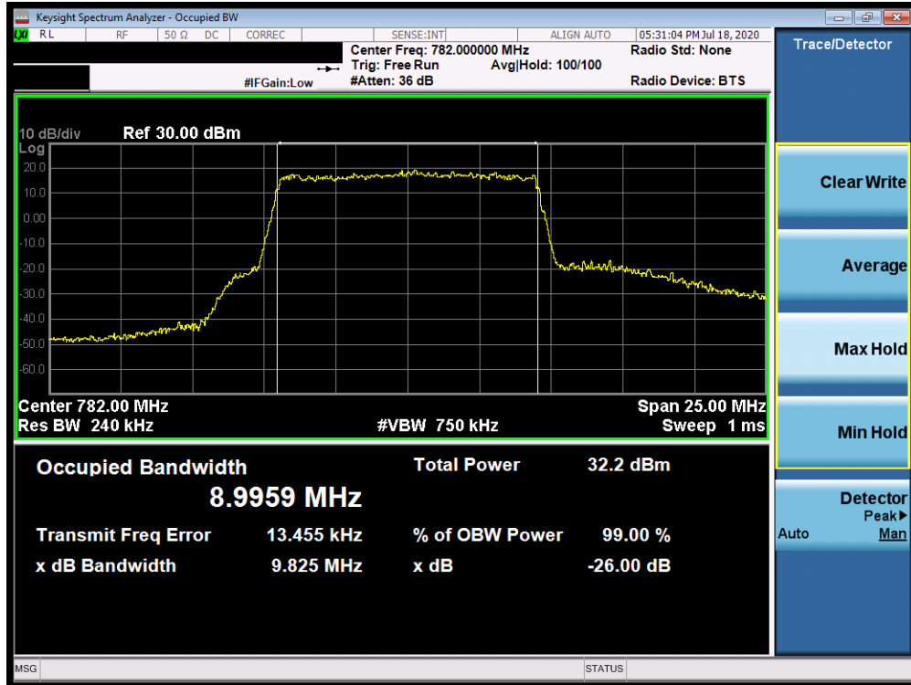
Plot 7-49. Occupied Bandwidth Plot (Band 13 - 10.0MHz 16-QAM - Full RB Configuration)
