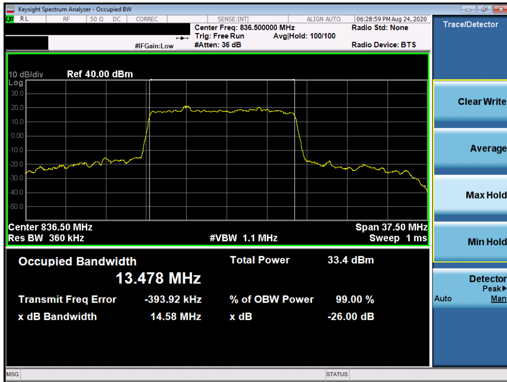
Plot 7-76. Occupied Bandwidth Plot (NR Band n5 - 15.0MHz DFT-s-OFDM BPSK - Full RB)
