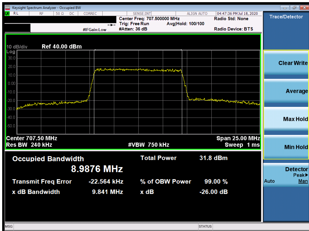
Plot 7-44. Occupied Bandwidth Plot (Band 12/17 - 10.0MHz 64-QAM - Full RB Configuration)
