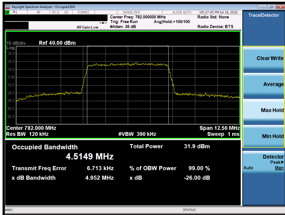
Plot 7-46. Occupied Bandwidth Plot (Band 13 - 5.0MHz 16-QAM - Full RB Configuration)
