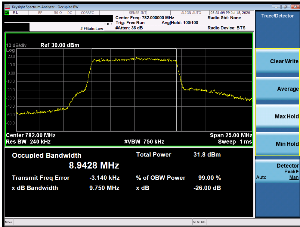
Plot 7-50. Occupied Bandwidth Plot (Band 13 - 10.0MHz 64-QAM - Full RB Configuration)
