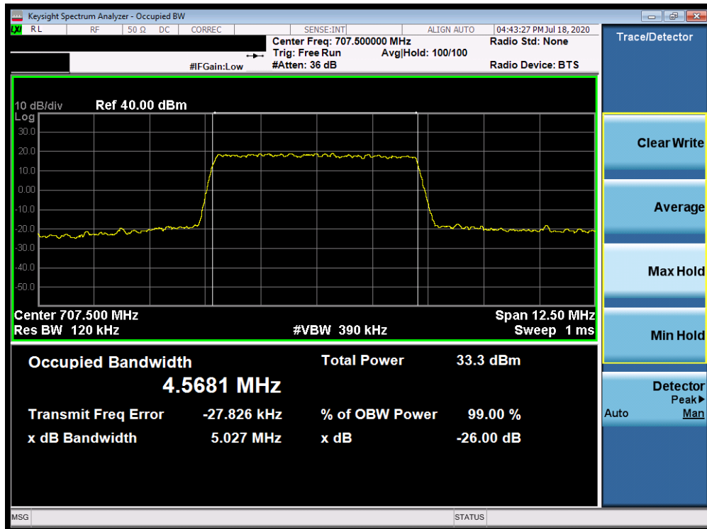
Plot 7-39. Occupied Bandwidth Plot (Band 12/17 - 5.0MHz QPSK - Full RB Configuration)
