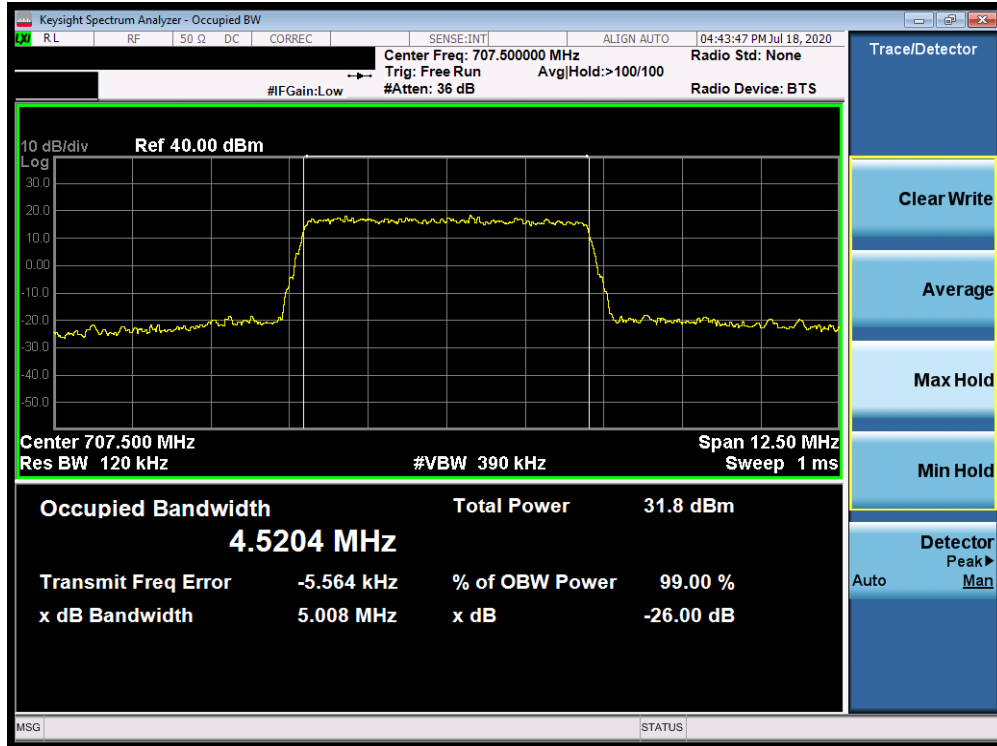
Plot 7-41. Occupied Bandwidth Plot (Band 12/17 - 5.0MHz 64-QAM - Full RB Configuration)
