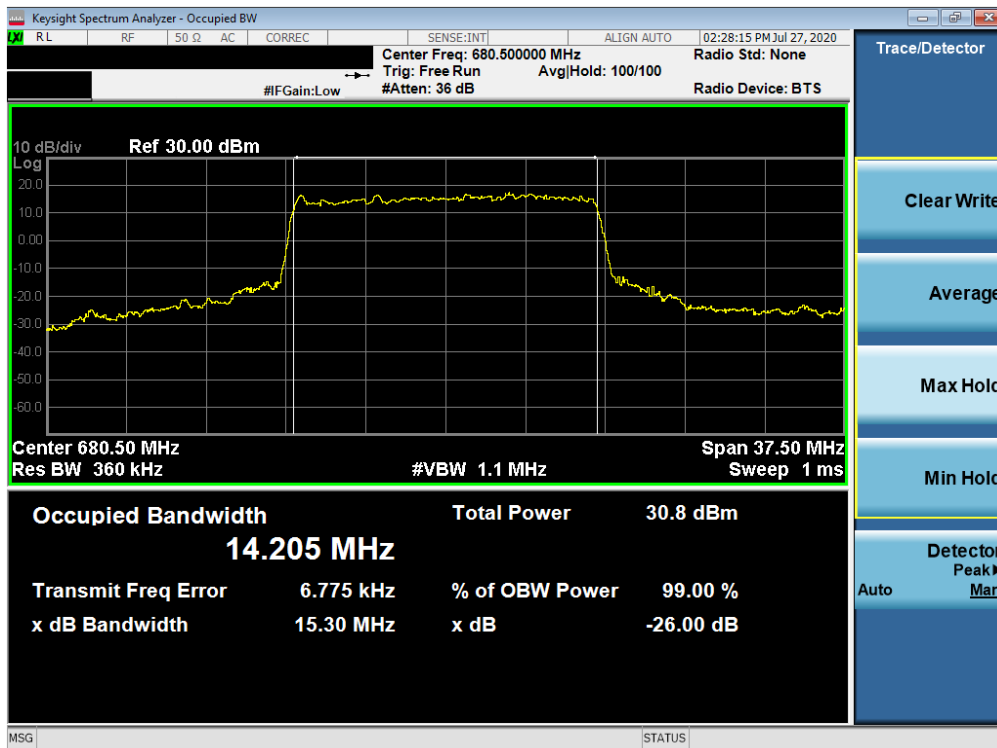
Plot 7-24. Occupied Bandwidth Plot (NR Band n71 - 15MHz CP-OFDM QPSK - Full RB)
