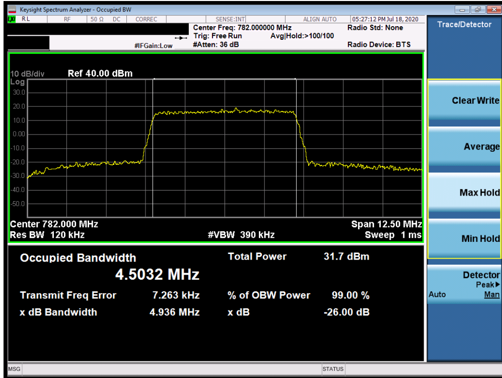
Plot 7-47. Occupied Bandwidth Plot (Band 13 - 5.0MHz 64-QAM - Full RB Configuration)
