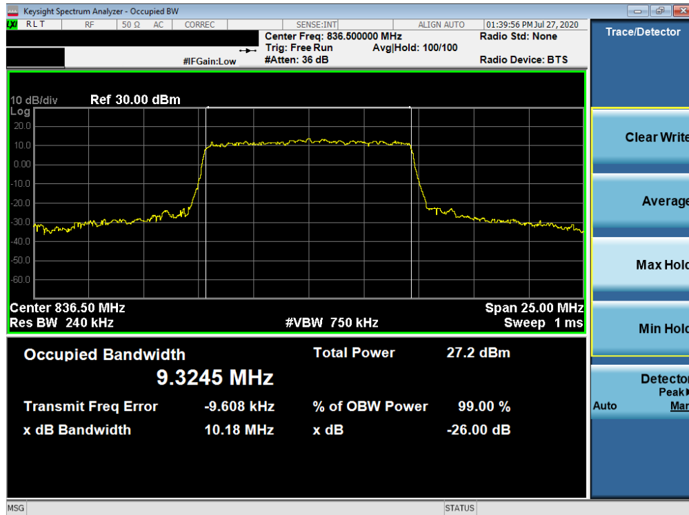
Plot 7-75. Occupied Bandwidth Plot (NR Band n5 - 10.0MHz CP-OFDM 256QAM - Full RB)
