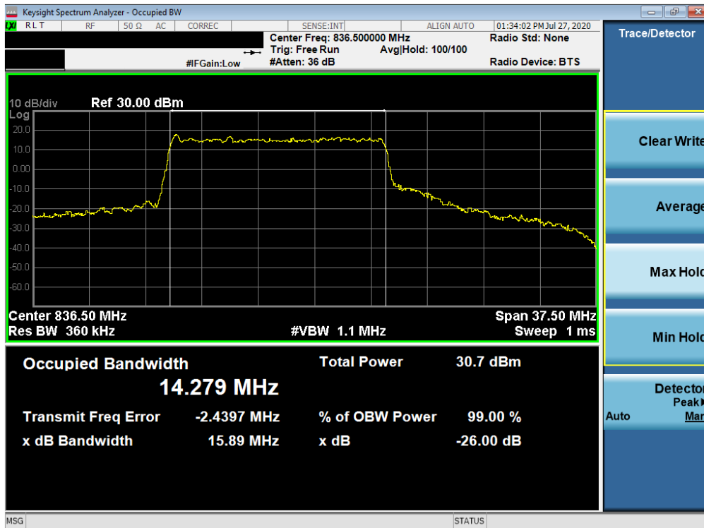
Plot 7-77. Occupied Bandwidth Plot (NR Band n5 - 15.0MHz CP-OFDM QPSK - Full RB)
