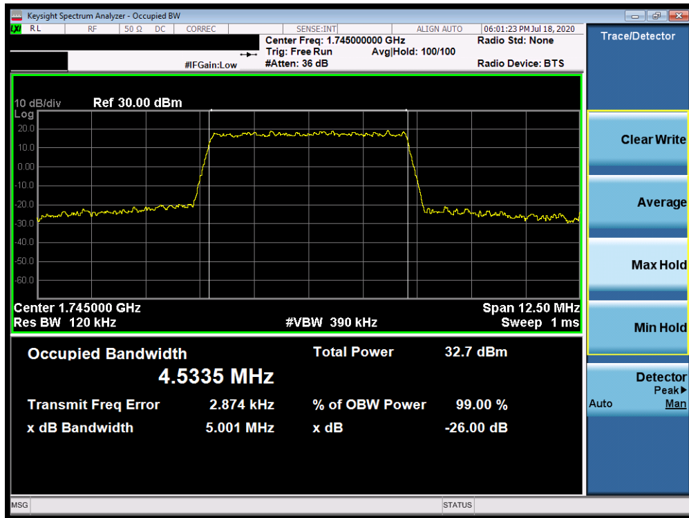
Plot 7-92. Occupied Bandwidth Plot (Band 66/4 - 5.0MHz QPSK - Full RB Configuration)
