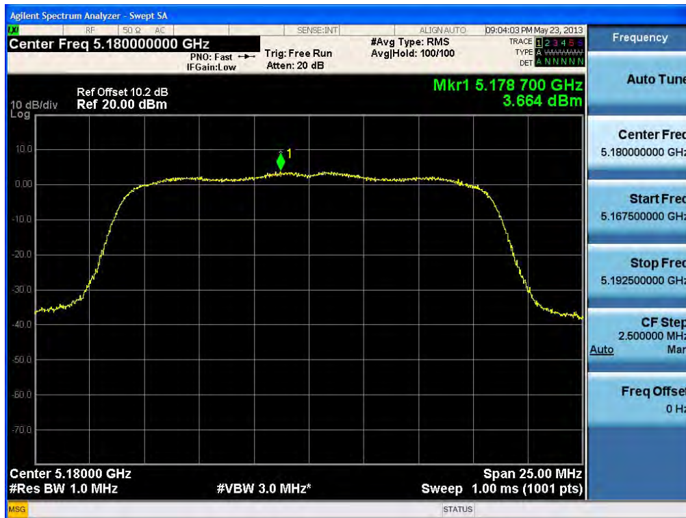
Power Spectral Density (802.11a-CH 40)
