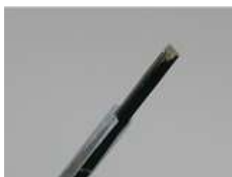
Figure 4.3 EX3DV4 E-field Probe
