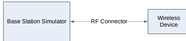
Figure 9-1 Power Measurement Setup
