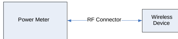
Figure 9-3 Power Measurement Setup
