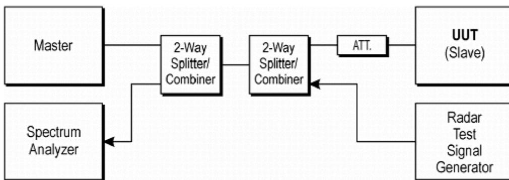
**Figure 3-1. Conducted Test Setup for DFS**
