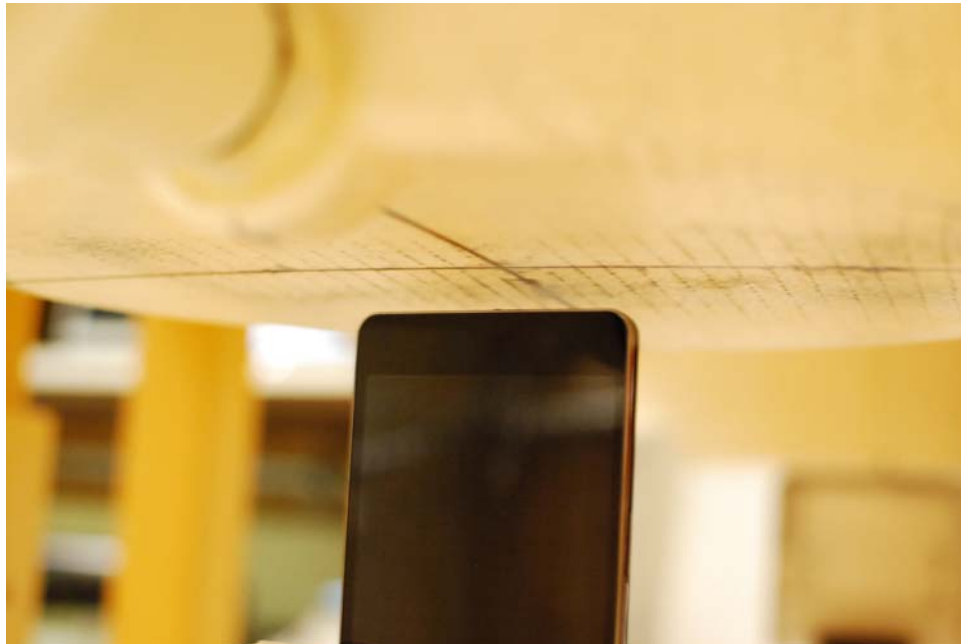
SAR Test Setup Photo 8: Bottom at 1.0 cm
