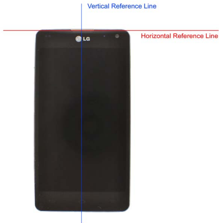
SAR Test Setup Photo 12: Vertical and Horizontal Reference Lines
