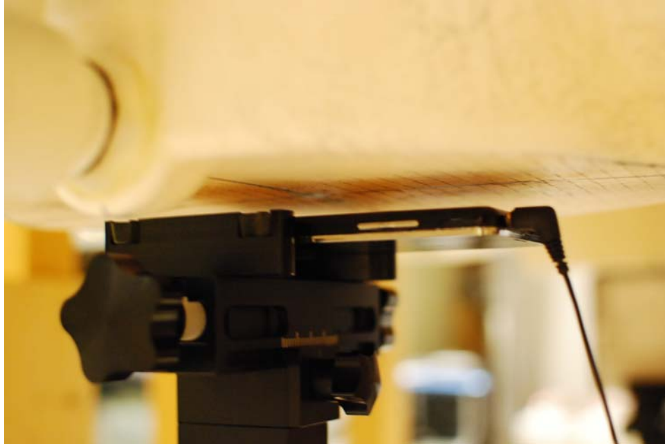
SAR Test Setup Photo 11: Body-Worn at 1.0 cm
