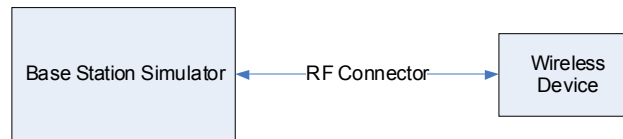
Figure 10-2 Power Measurement Setup
