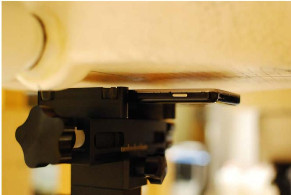
**SAR Test Setup Photo 6: Front at 1.0 cm**
