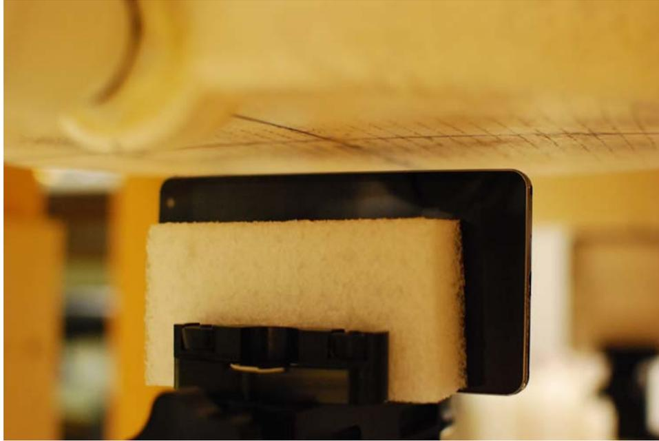
**SAR Test Setup Photo 9: Right at 1.0 cm**
