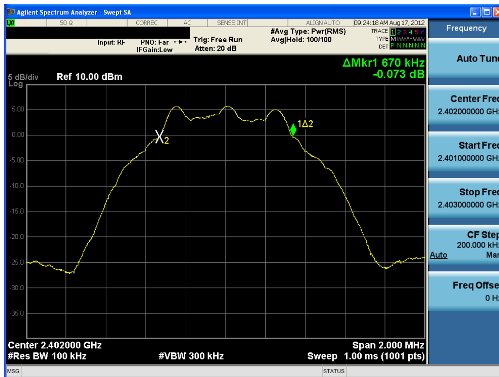
Plot 6-1. 6dB Bandwidth Plot (Bluetooth (LE) – Ch. 0)
