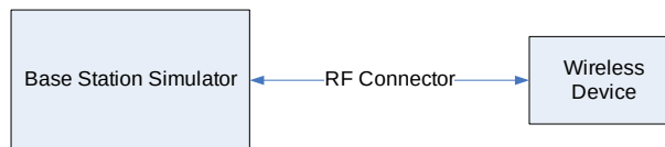
Figure 10-3 Power Measurement Setup
