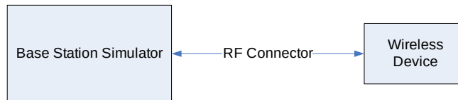
Figure 10-2 Power Measurement Setup
