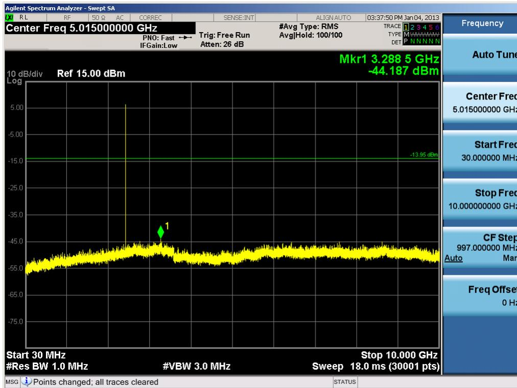
Plot 6-38. Conducted Spurious Plot (Bluetooth, 1Mbps – Ch. 39)
