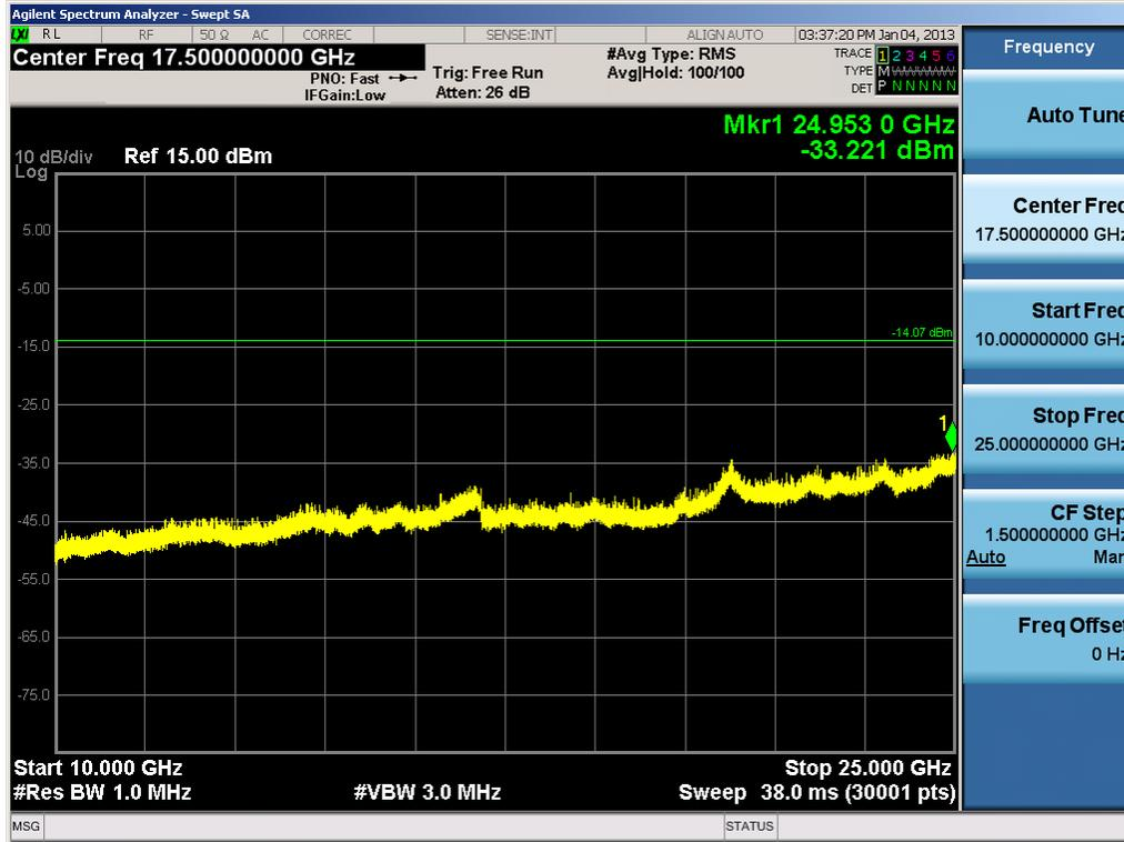
Plot 6-37. Conducted Spurious Plot (Bluetooth, 1Mbps – Ch. 0)
