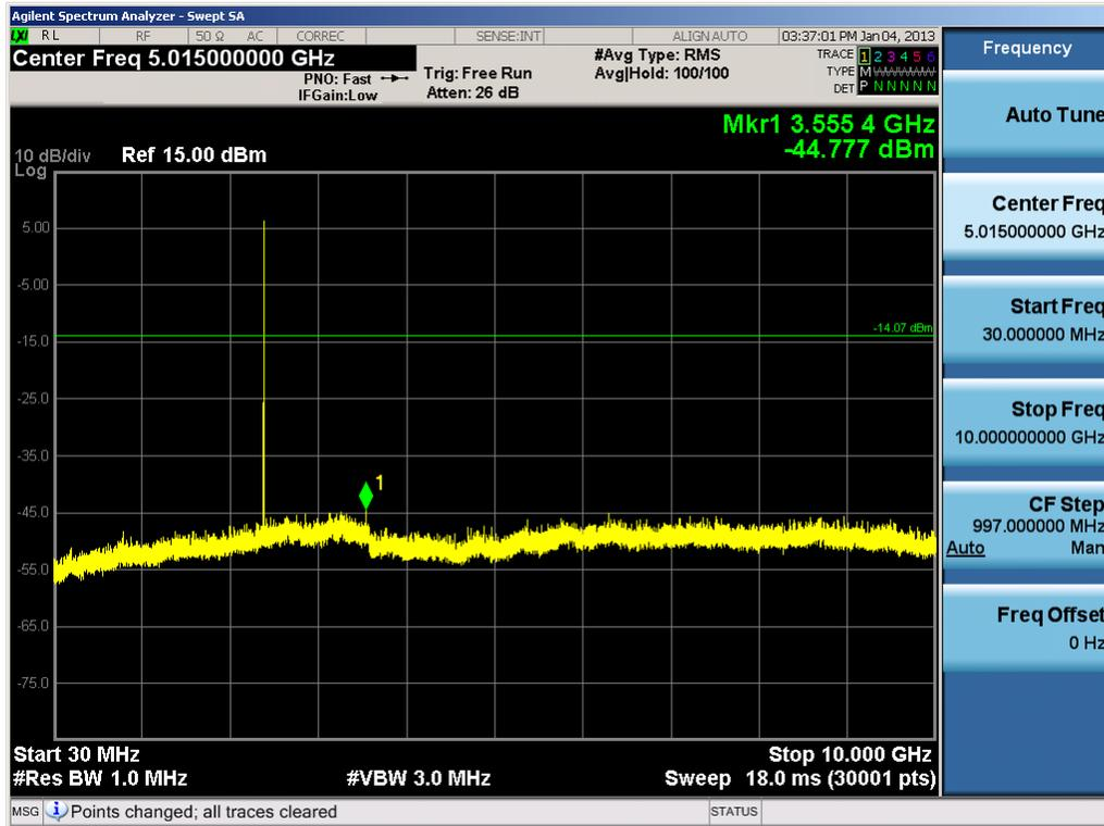
Plot 6-36. Conducted Spurious Plot (Bluetooth, 1Mbps – Ch. 0)
