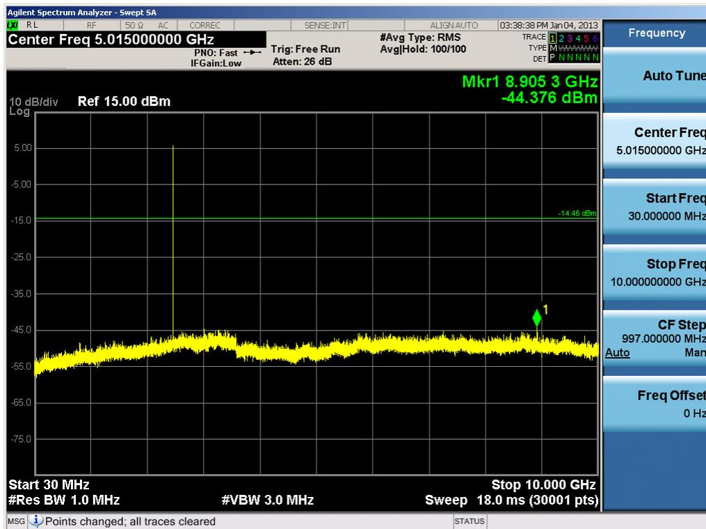
Plot 6-40. Conducted Spurious Plot (Bluetooth, 1Mbps – Ch. 78)
