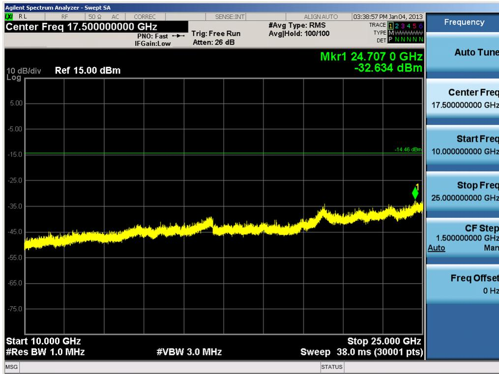
Plot 6-41. Conducted Spurious Plot (Bluetooth, 1Mbps – Ch. 78)
