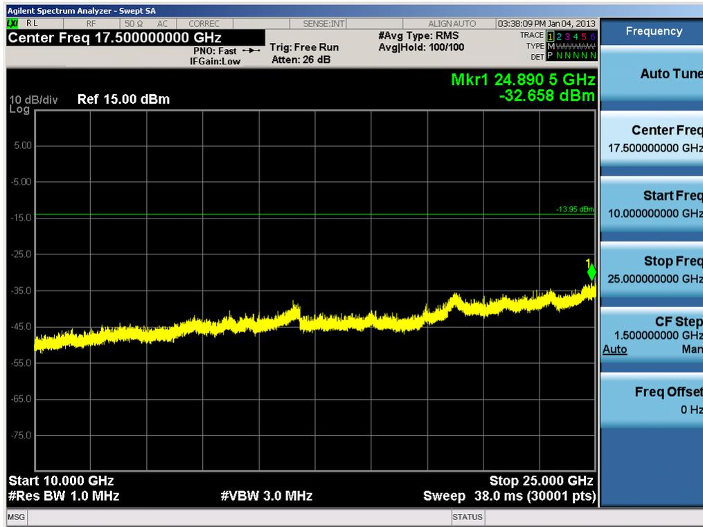
Plot 6-39. Conducted Spurious Plot (Bluetooth, 1Mbps – Ch. 39)
