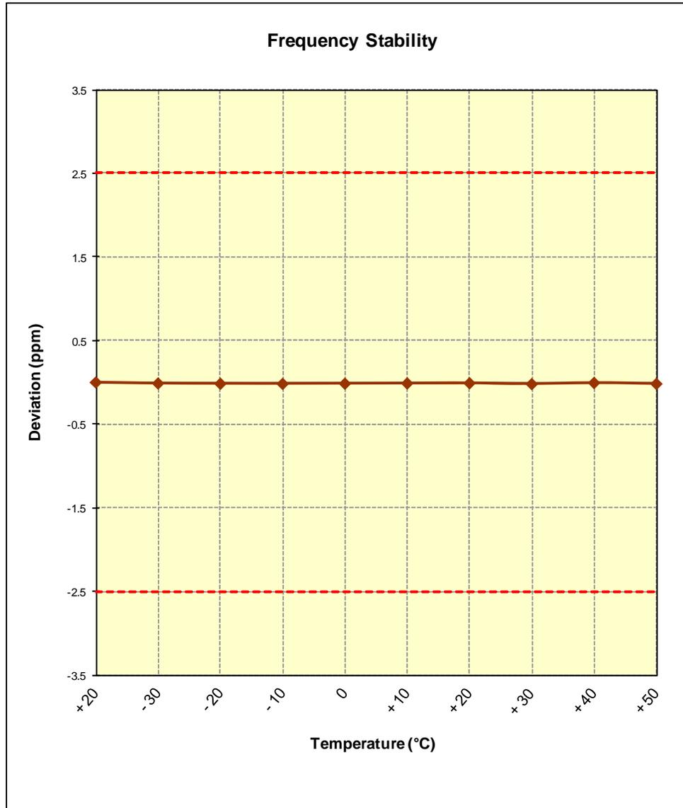
**Figure 6-1. Frequency Stability Graph (Cellular GSM Mode – Ch. 190)**
