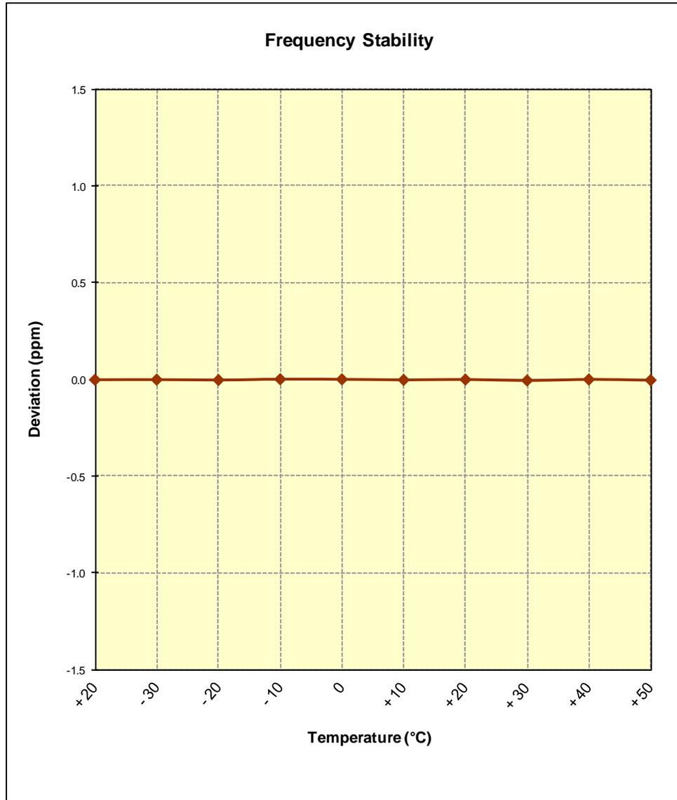
**Figure 6-4. Frequency Stability Graph (PCS WCDMA Mode – Ch. 9400)**
