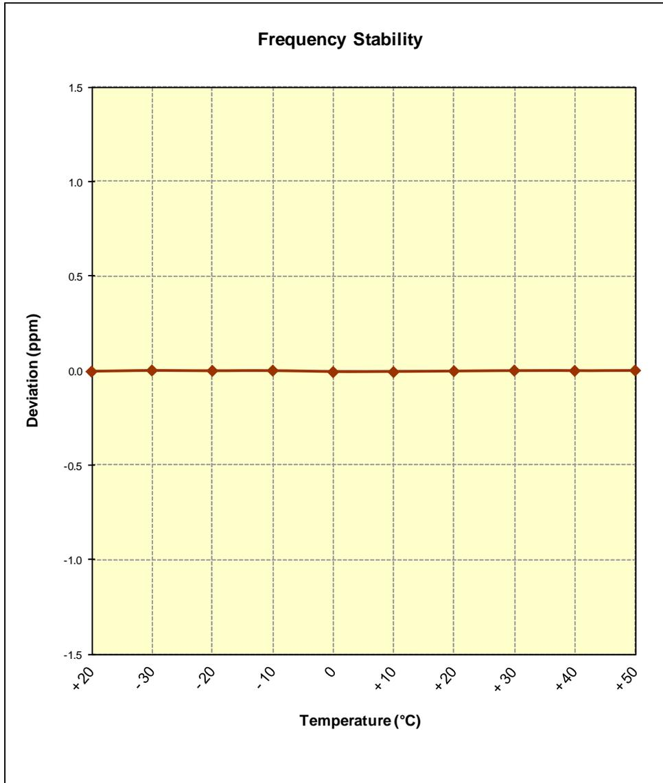
**Figure 6-3. Frequency Stability Graph (PCS GSM Mode – Ch. 661)**
