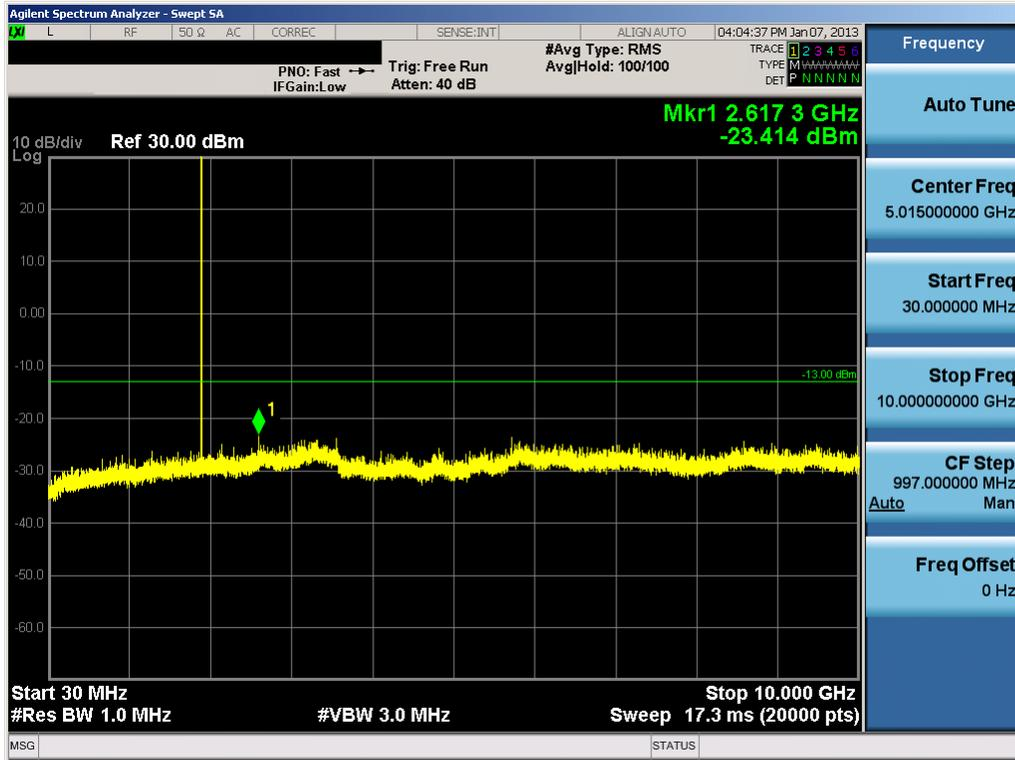
Plot 7-17. Conducted Spurious Plot (PCS GSM Mode – Ch. 810)
